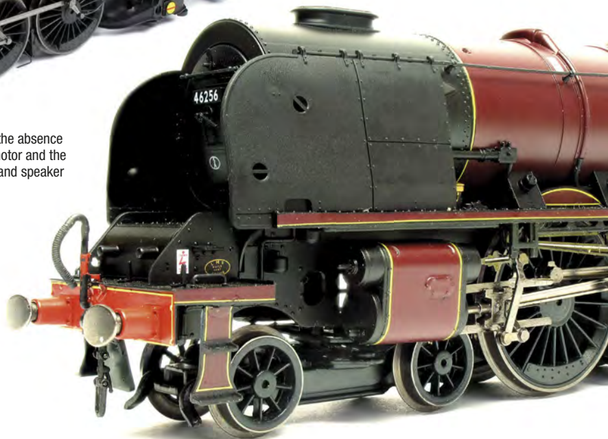
It should be possible to fit the front steps and allow sufficient movement on all but the sharpest of curves.
