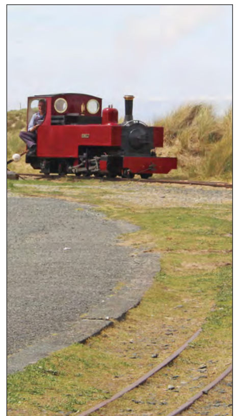
■ The Fairbourne Gala also featured the official return to service of the line's 12.25in gauge 2-6-4T 'Russell' after a major overhaul. This loco was built in 1979 in the style of a Leek & Manifold Railway Kitson loco and remodelled in 1985 to look like the famed North Wales Narrow Gauge/Welsh Highland engine.
