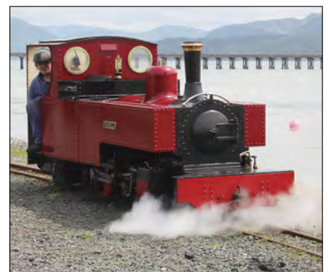
■ The Fairbourne Gala also featured the official return to service of the line's 12.25in gauge 2-6-4T 'Russell' after a major overhaul. This loco was built in 1979 in the style of a Leek & Manifold Railway Kitson loco and remodelled in 1985 to look like the famed North Wales Narrow Gauge/Welsh Highland engine.
