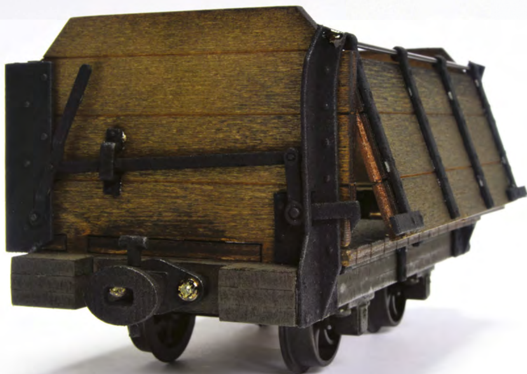
The completed Mill wagon showing side operating linkage with extending side open door
