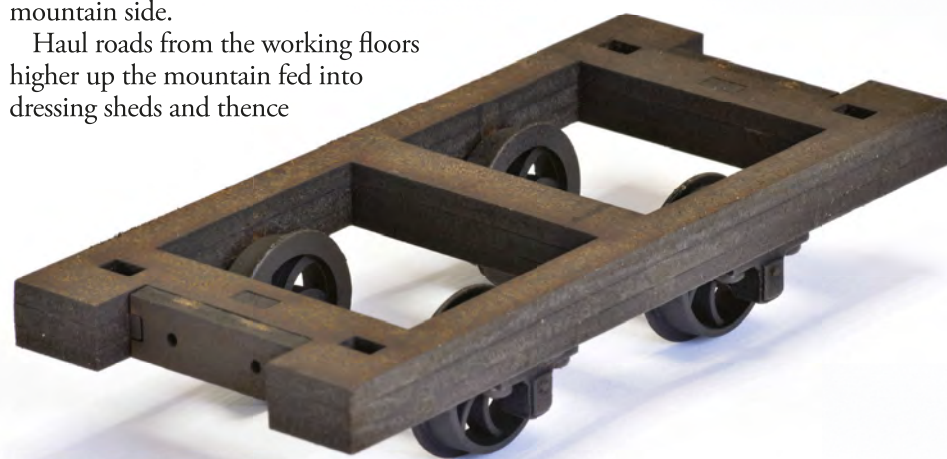
The very versatile solebars of this chassis could have many applications
