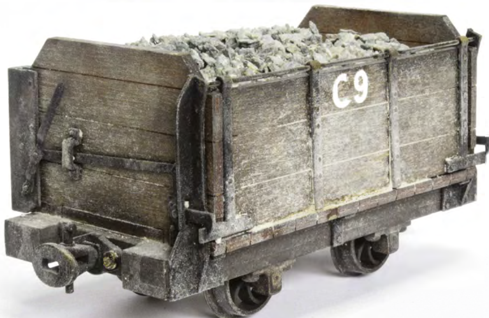
A fully loaded and weathered Mill wagon (side tipping) in typical guise
