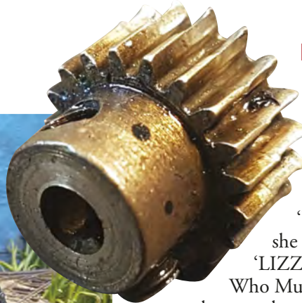
Heavily worn pinion gear from 'LIZZIE'
