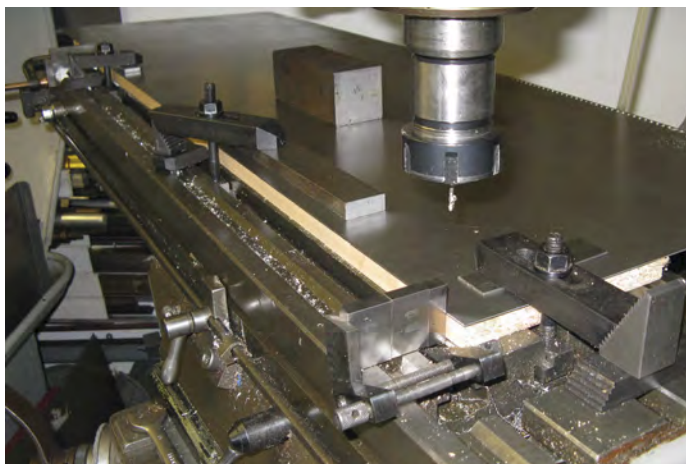
LEFT PHOTOGRAPH 3 Drilling the top the cover sheet.
