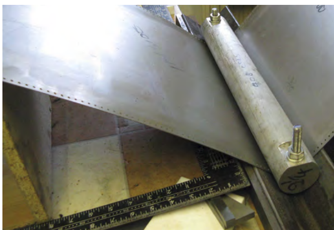
LEFT PHOTOGRAPH 5 Bending the cover. Note roofing square to keep accuracy and the sheet of chipboard (to the left) to prevent the sheet flopping about.
