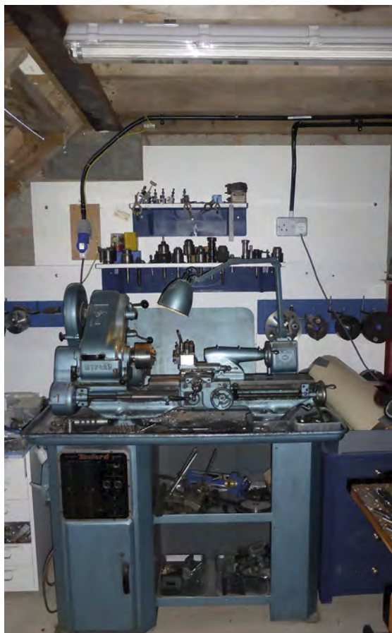
ABOVE – PHOTOGRAPH 2 1960 Myford S7 with low voltage lighting.
