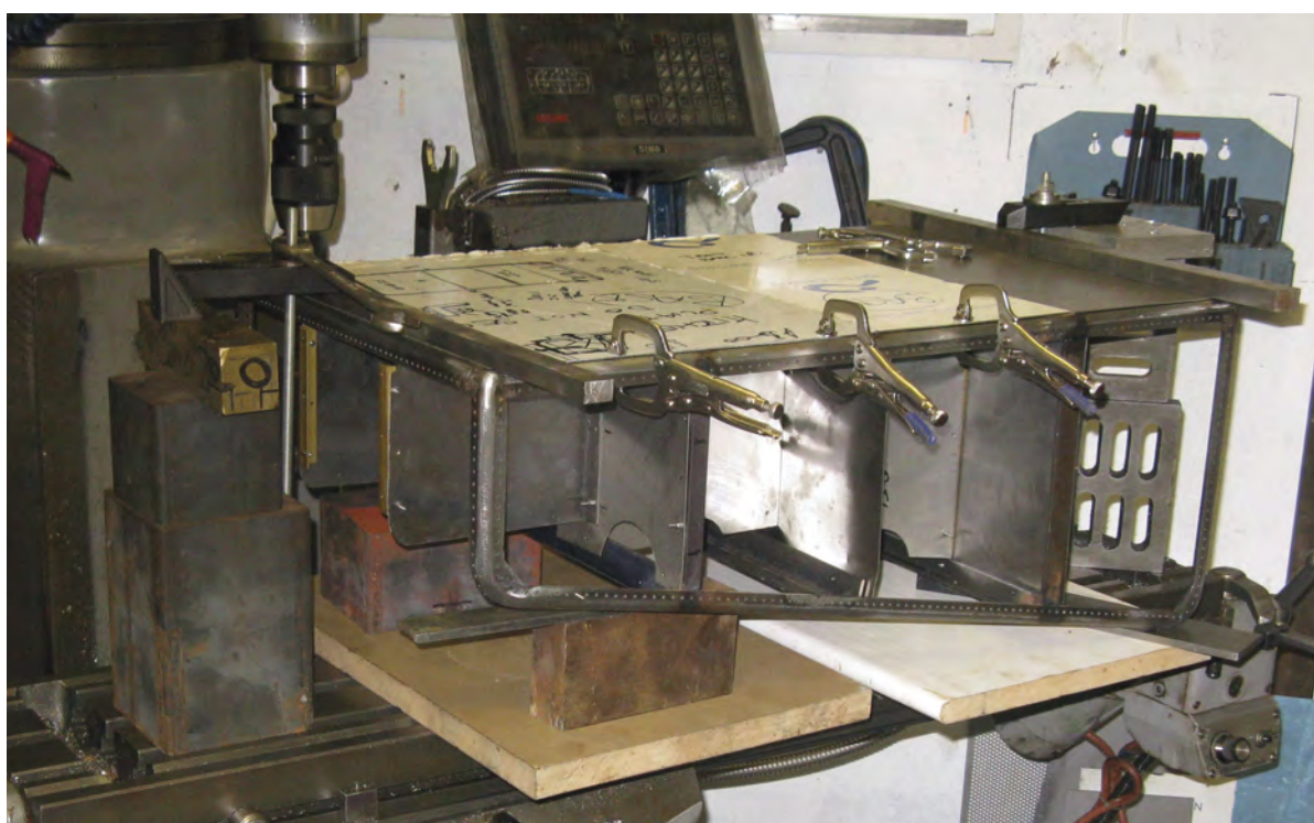
ABOVE PHOTOGRAPH 9 Welding the bottom angles.
