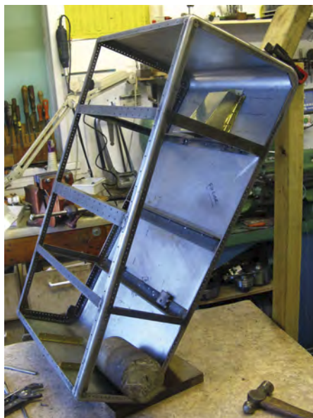
LEFT – PHOTOGRAPH 14 Setup for riveting the corners.
