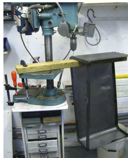
BELOW – PHOTOGRAPH 8 Drilling the holes. The end angles are not yet fitted.
