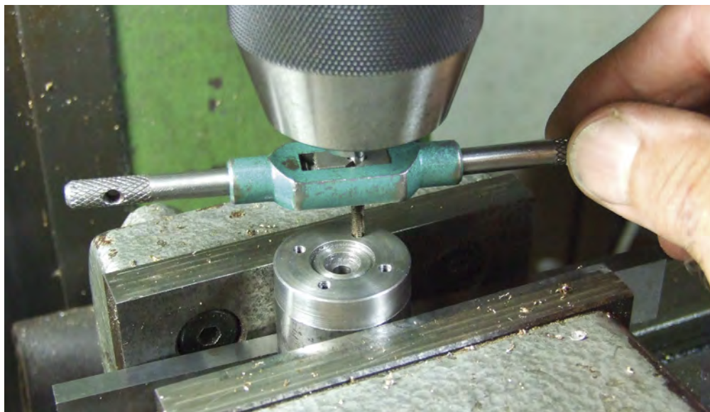
ABOVE PHOTOGRAPH E30 Threading fixture for M3 cover securing bolts.
