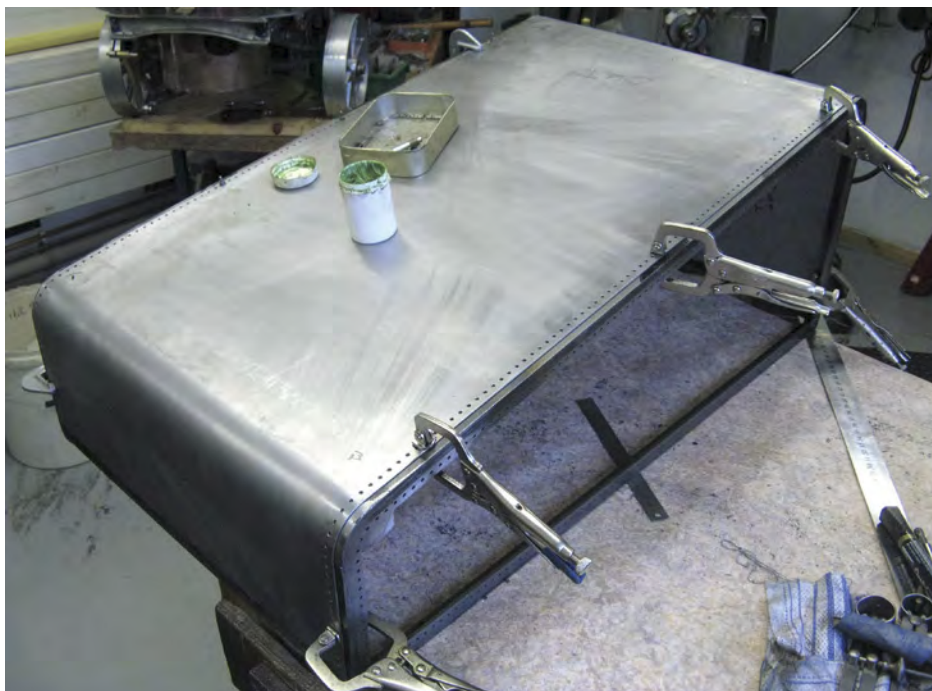
LEFT – PHOTOGRAPH 7 Clamping the top sheet in place.
