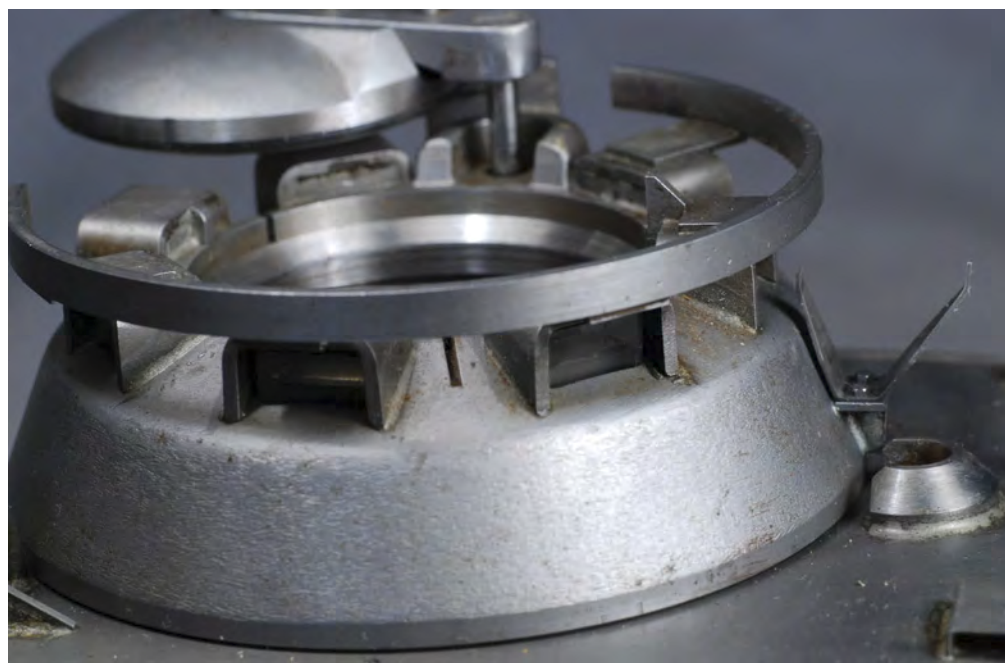
BELOW PHOTOGRAPH 7 The cupola, mounted on the turret, and its seven viewing hoods.
