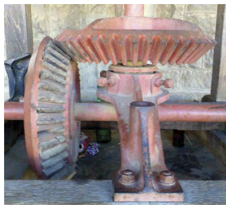
BELOW A pair of bevel gears of a similar type to those used at Rippingale.
