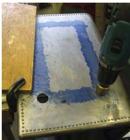
BELOW – PHOTOGRAPH 15 Cutting out the front hatch.
