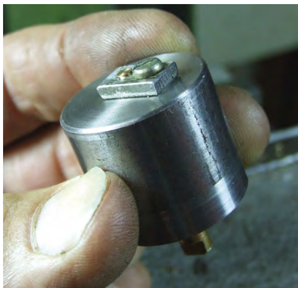
BELOW PHOTOGRAPH E31 Retaining screw for "Captive Nut" in fixture.
