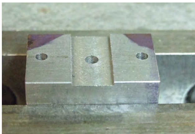
LEFT PHOTOGRAPH E32 Recess in port face – milled 1st stage.
