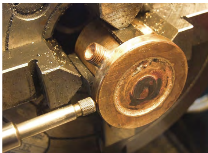
ABOVE – The fabricated brake cylinder being set-up for the drilling and boring operations.
