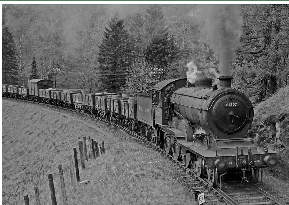
B12 4-6-0 No. 61507 climbs through Glen Fiddich from Craigellachie, with an up goods loaded with whisky in barrels in 1951. In accordance with the rules, the barrels are loaded on their ends and secured in position with ropes. RAIL ARCHIVE STEPHENSON
