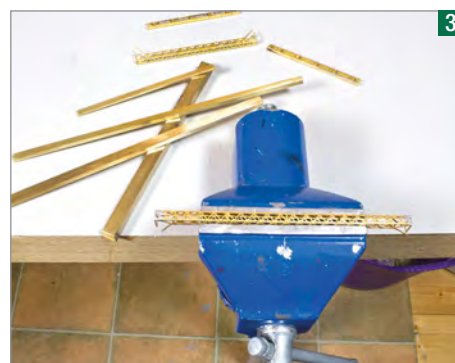
The bending formers supplied by NBL for its portal kits are strongly recommended, along with a bench vice for folding the long thin etchings.
