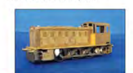
The other half of the test etch sheet was used for the 440hp 0-6-0. This has many parts in common with the 330hp 0-4-0 and will be released as a kit in the near future.
