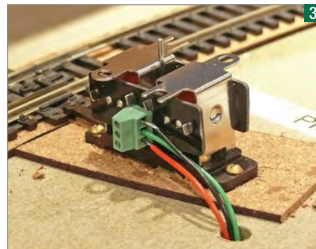
3 Run three wires (red, green and black are commonly used for point motors) from the ADS decoder to the three terminals on the motor.
