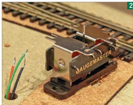
2 I'm mounting it above the board for ease of maintenance as it is in an off-scene yard. Mark the position and ensure the PL-12 is at the correct distance from the point.
