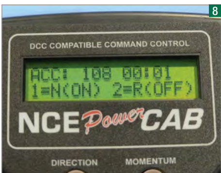
8 Slide the switch back to 'RUN' and press 'Select Accy' again. Press '1' to select 'N(ON)' and your motor should change. Adjustments may be required to ensure reliability.
