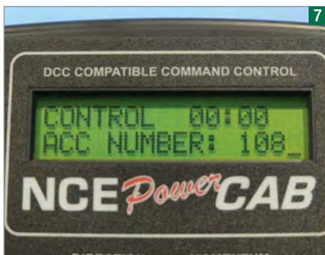
7 Key in the desired ID number, press 'ENTER', Press '1' to select 'N(ON)' and toggle backwards and forwards several times to inform the ADS of its new identity.
