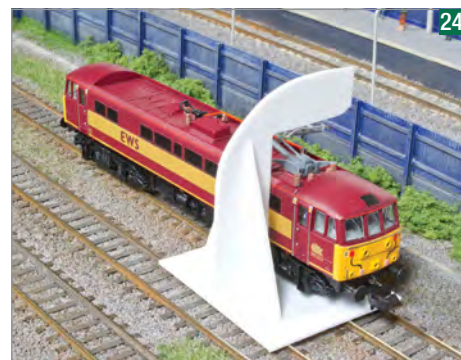
Setting registration arms to a standard height allows the operation of the unsprung Dapol pantographs. A gauge sets the height of the pantographs correctly.
