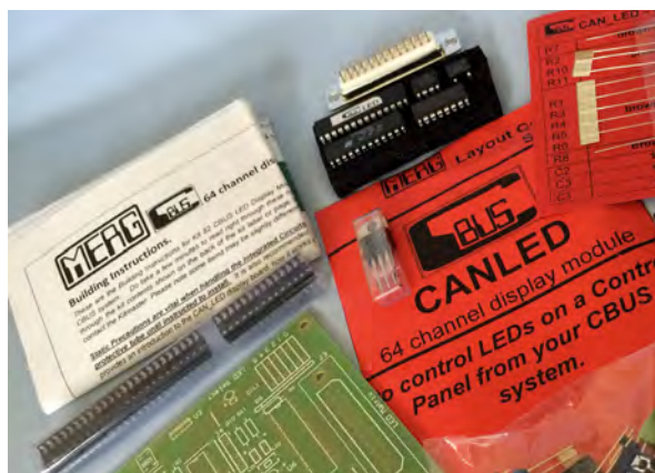
LEFT: Components and instructions on display from a MERG CANLED electronic kit. The only skill required to assemble any MERG kit is basic soldering.
