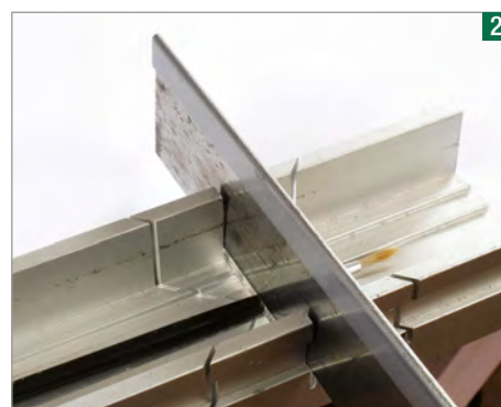
Start by removing the ferrule and bristles with a razor saw. Invest in a mitre box, which will give you a safer, straighter cut.
