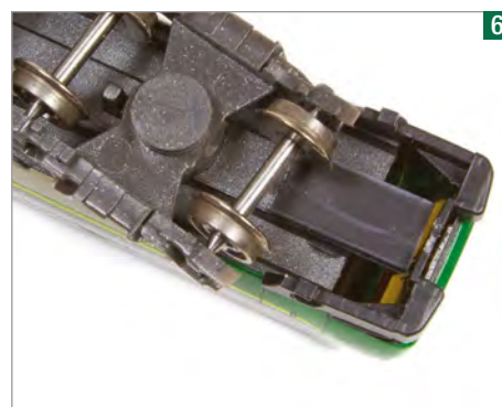
Shims of 20thou' styrene are built up on the underframe until the new coupling can be fitted in the gap in the modified front fairing.
