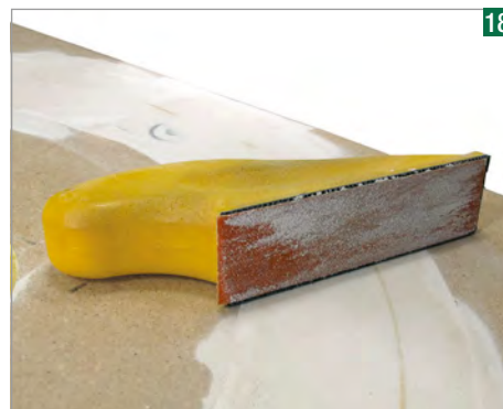
Using a sanding block, the surface is flattened until the guide wire is visible. The van can get 'lost' if separated by more than 0.75mm from the guide wire.
