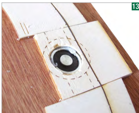
The magnet is too powerful and pulls the van away from the wire. Setting it a few millimetres below the surface solves the problem.
