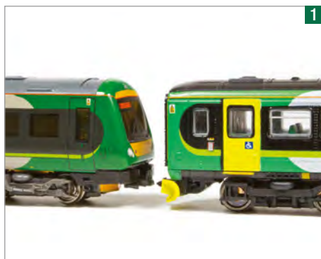
As supplied the models cannot be used together. The position of the new couplings was determined by the gap in the fairing of the '170' occupied by a cosmetic coupling.
