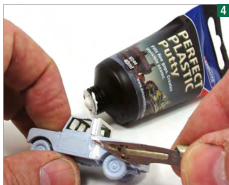
Perfect Plastic Putty from Deluxe Materials is applied with a knife tip filling the gaps smoothly. It is easily sanded for a smooth finish.
