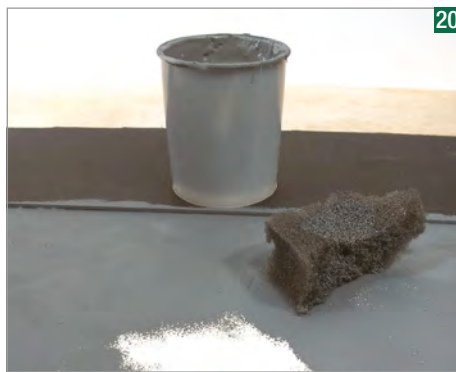
Faller suggests applying the road paint with a small roller. Not having one to hand, I applied it with a sponge to give a more realistic texture.
