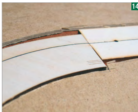
The road is 3mm thick, so the surrounding surface has to be built up to the same level. Thin MDF is cut to shape and fitted.
