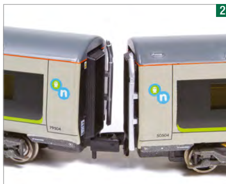
The inner ends of the '170' will benefit from MT couplings to close up the gangways, yet still be reliable on 12in curves. New couplers will be mounted on the underframes.
