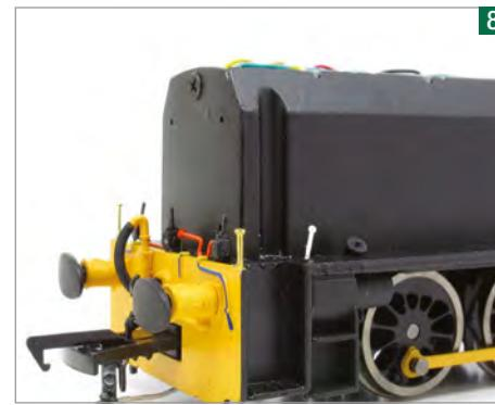
The plastic handrail pommels by the front steps are vulnerable to knocks. One had already broken away, so replacement with brass pins is an improvement.
