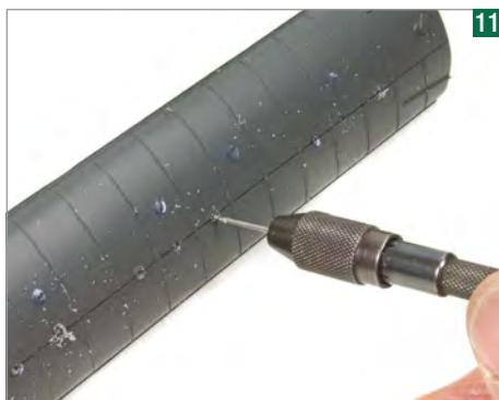
Some vent positions differ between model and prototype. The new positions are determined and 0.6mm diameter pilot holes are drilled in each vent position.
