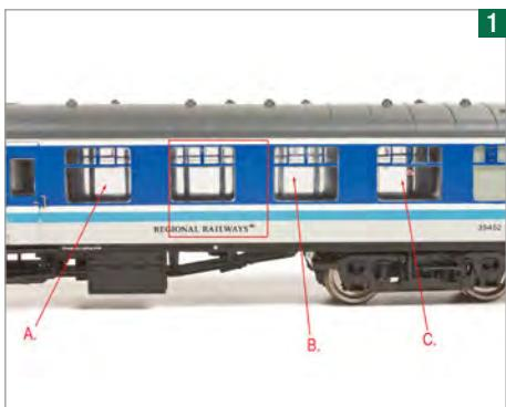
Windows (A) and (B) are fitted with blanking plates, the latter with a small vent. One passenger compartment is retained (C) together with the toilet compartment.
