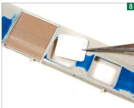
Window plating is completed with 10thou styrene sheet. If you prefer, 5 thou' brass sheet is a better material to use as it is thinner, and more prototypical.
