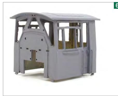
Although I wouldn't normally prime plastic, in this instance a spray from a car aerosol makes it easier to identify areas that require more attention.
