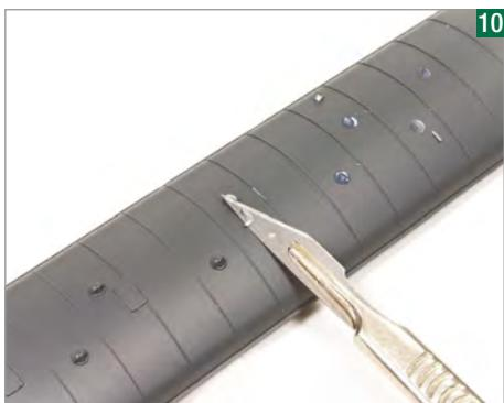
NNX 80212 (former BSK 35307) had dome vents rather than ridge dome vents as modelled. The mouldings are shaved off with a sharp scalpel.
