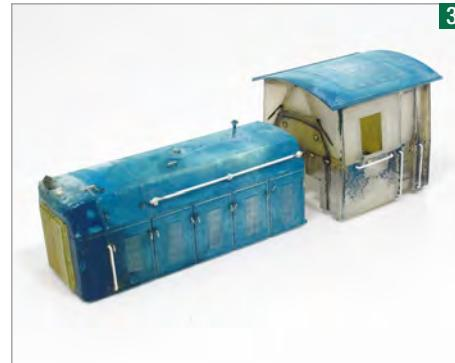
Deluxe Materials 'Superstrip' removes the paint but should be washed off after five minutes. After 20 minutes the cab glazing has reacted - read the instructions!
