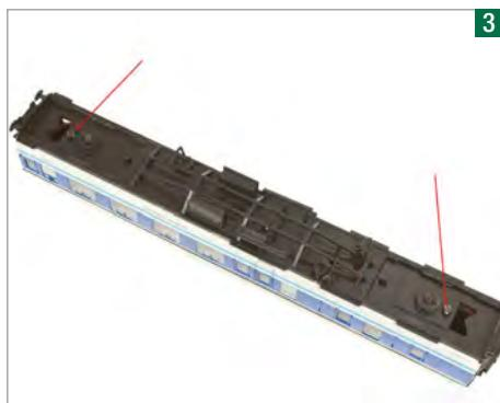
Bachmann Mk 1s are held together by the interior moulding securing the sides to the underframe. Three screws secure the interior to the underframe.
