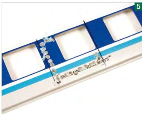
Cutting out commences by drilling around the edge of the new door opening with a 2mm drill. Retain the top section of the side - it has holes to secure the roof.
