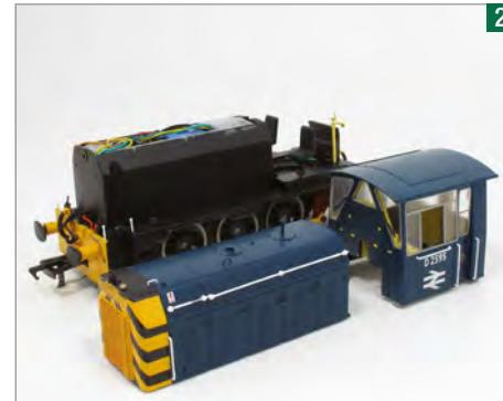
Disassembly starts by removing a couple of screws under the front of the footplate. The cab then slides off followed by the bonnet.
