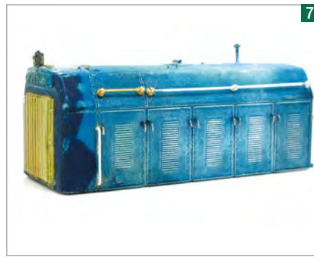
When stripping the paint, I damaged the handrail knobs on one side. The broken ones are replaced with short brass versions and straight wire.
