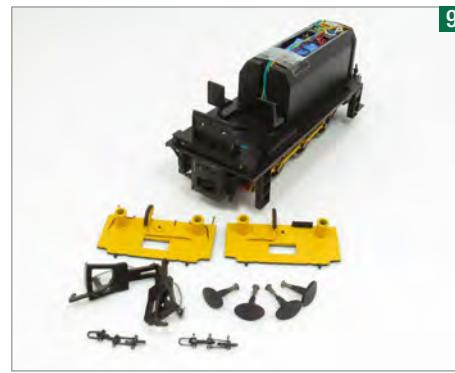
The bufferbeams pull away from the chassis. There doesn't appear to be any glue used in assembly which makes painting easier.
