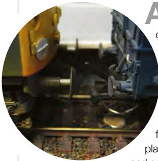
**A** Before ballast was added I set about placing small circular magnets at various strategic points in the track to allow me to uncouple stock and locomotives thus giving me 'hands free' operation. A 10mm diameter neodymium magnet sourced from First4Magnets was placed just below sleeper height and covered by a thin piece of black weathered plastic card.
