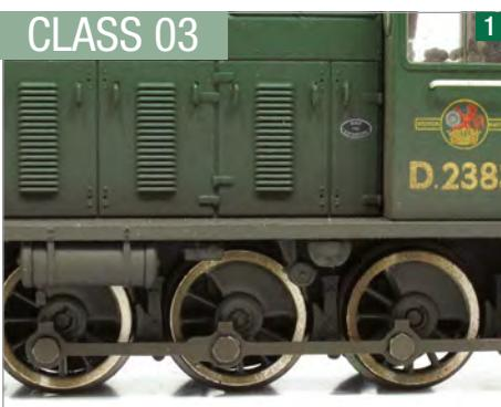
On the production line, weathering is applied with a quick pass of an airbrush. Where the coupling rods shield the wheels, shiny metal catches the eye.
