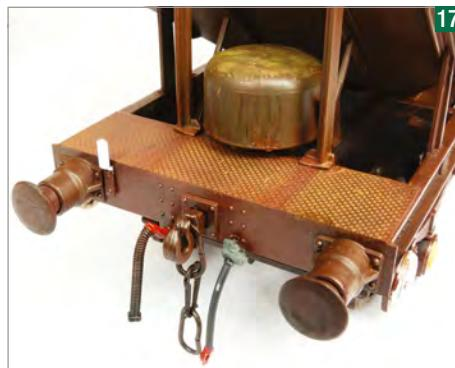
The TOPS code ZFW was given to a small number of 'Dogfish' with a through airpipe. I'm using a spare from a Heljan sprue, painted and superglued into place.
