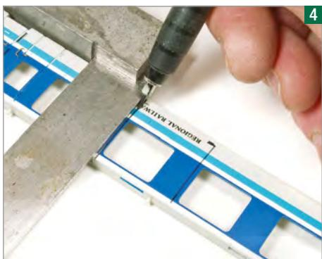
The position of the roller shutter doors is measured and marked in place. They are 28mm in width. Note the proximity to one of the window openings.
