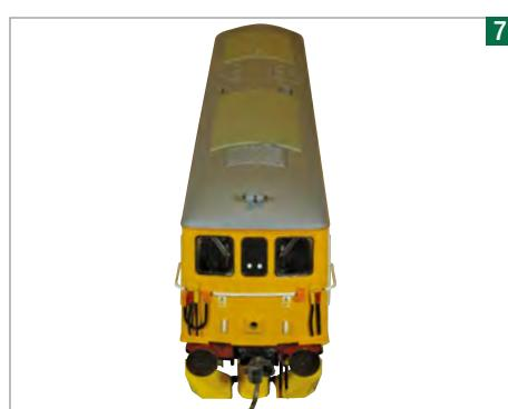
Painting complete - note the different colour of the two removable fibreglass panels between the cabs. These allow some daylight into the engine room.
