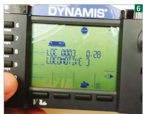
The default locomotive address default is '3'. Calling it up on screen is a quick procedure that involves scrolling left and right using the keys until it is found.
