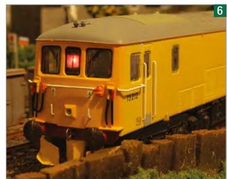
As the '73' will be permanently coupled to a test train, the SR headcode blind only lights up (in red) when the locomotive is propelling.
