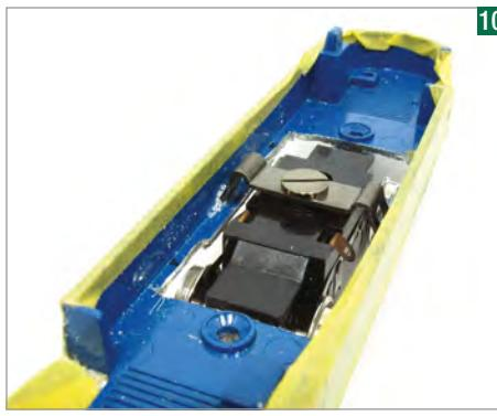
Bending the legs of a support supplied with the SPUD allows the bogie to sit at the perfect height. I'm gluing the bracket centrally within the model using two-part epoxy.
