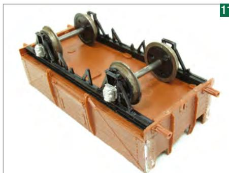
The Romford wheelsets aren't going to turn, so I'm replacing them with ones from my scrapbox held in place with epoxy glue.
