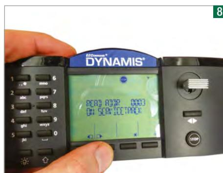
Entering programming mode is as simple as using the joystick to flick up and down until 'Program' is displayed. The tick button below is then pressed.
