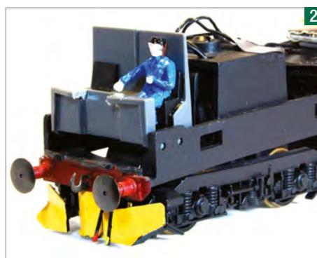
Extra details include miniature snowploughs (unique to NR's Class 73s), bufferbeam hoses and couplings, new Oleo buffers and a driver in one cab.
