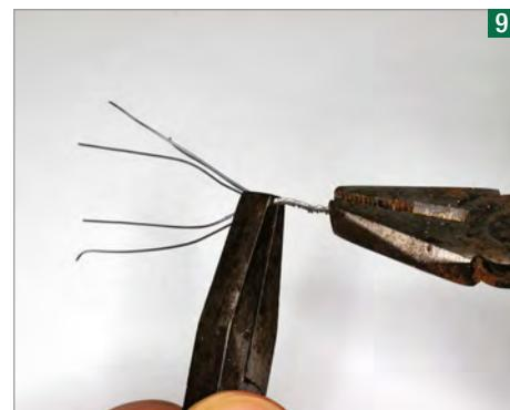
Acquire some wire from a DIY or garden centre (about 0.7mm is ideal) and make an armature by twisting several strands of wire together using pliers.
