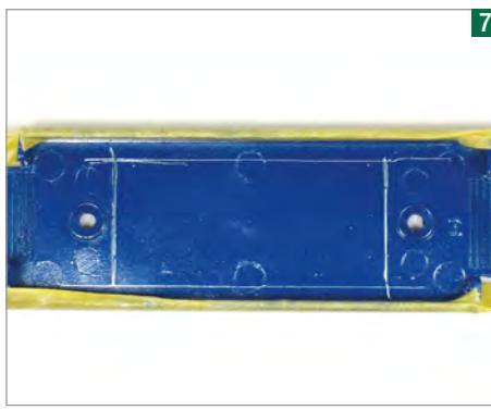
Fitting the power bogie requires a hole to be cut in the floor. Leave around 2mm on each side for the support to fit. The cut-out is 42mm long.
