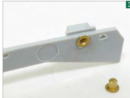
To further improve how the wagon runs, drill the axleboxes with a 2mm bit and insert brass top hat bearings with glue - it makes a big difference.
