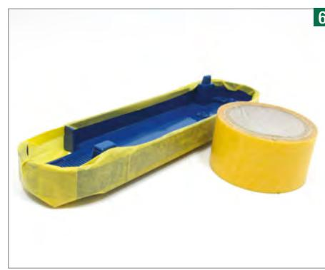
I'm covering the body parts with low-tack masking tape to protect the paint from damage while handling. It'll avoid having to repaint the model later.
