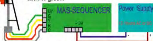
The diagram shows the simplicity of the wiring. A terminal is also provided for Manual override to red for stations and junctions. Lines with more than one signal use IRDASC-4 units to control the other signals. A single wire from the MAS-SEQUENCER to the IRDASC-4 synchronises the aspects of the signals. Units are compatible with conventional and DCC control.
