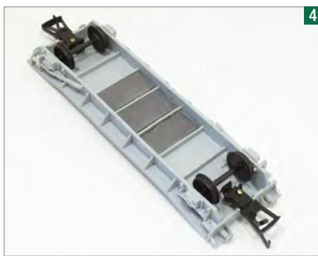
Assembling the kit takes a few minutes. The sides slot into place under the floor followed by the bufferbeams. Lead flashing superglued underneath adds extra weight.
