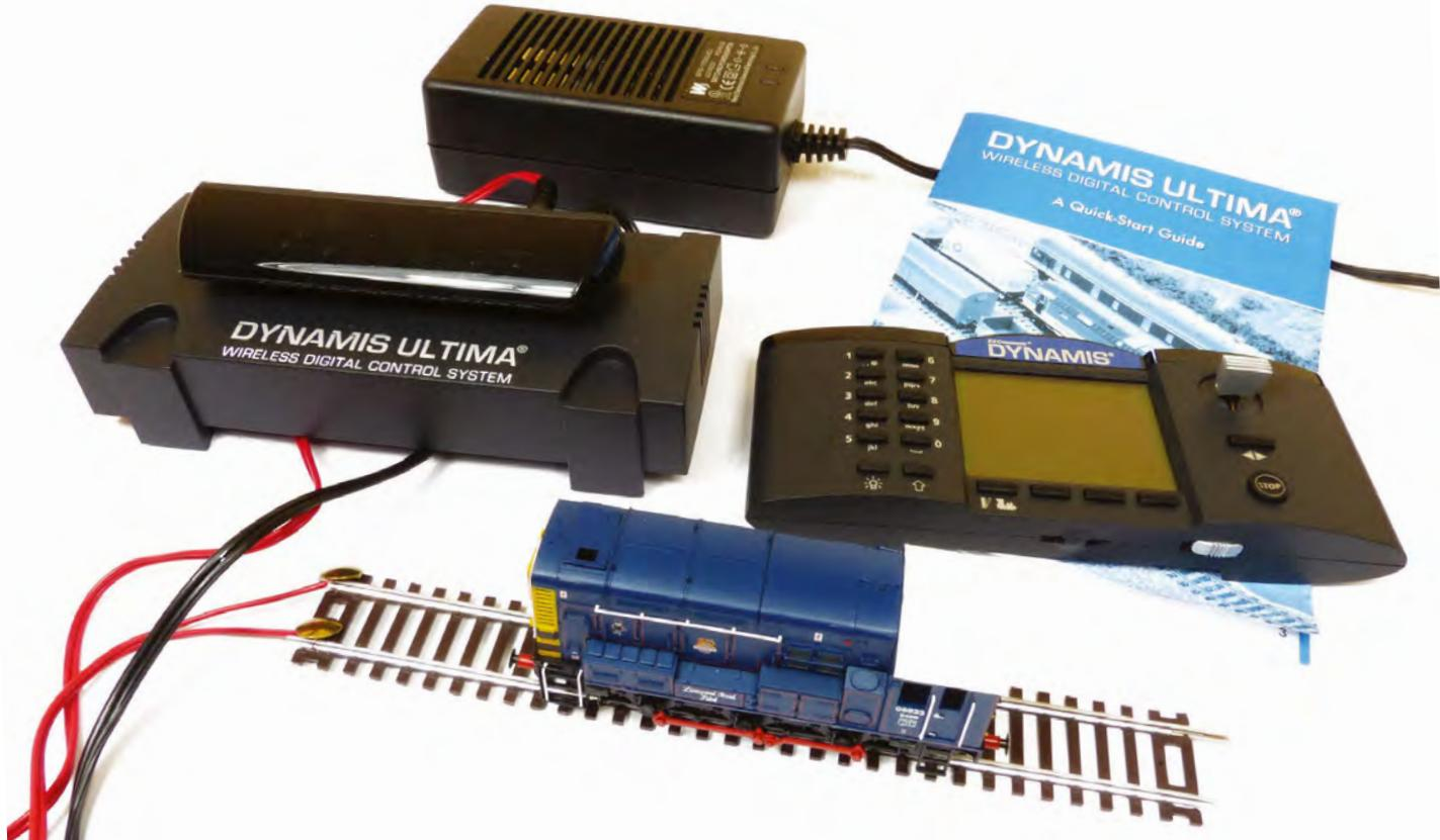
**ABOVE:** All you'll need to get started 'mapping' a DCC decoder is pictured here. A DCC controller (in this case a Bachmann Dynamis Ultima), a locomotive and a section of track connected to the programming track terminals. A DCC system and decoder manual are also helpful to keep at hand.
