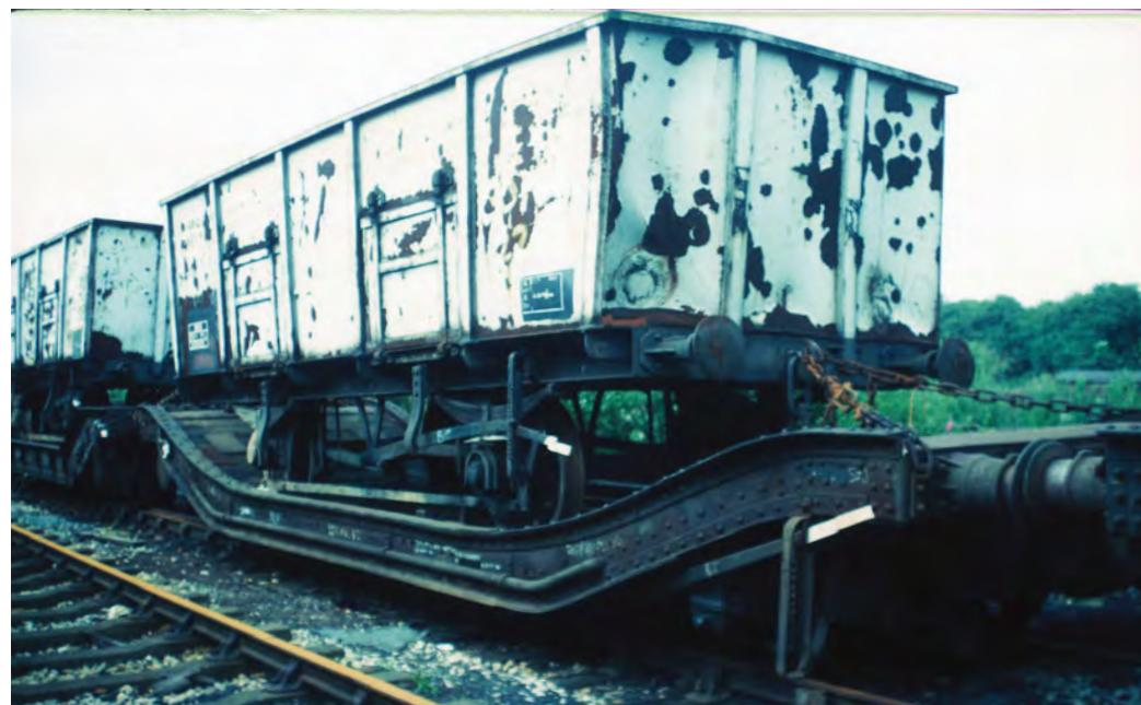
Seen at Horwich Works on June 16 1980, B904116 is a BR-built 'Lowmac' built to Lot 2592 at Swindon in 1955. It is loaded with an accident damaged 21T MDO mineral wagon. The heavy indent at this end caused by 'buffer override' is witnessed by the grease patches left behind. PAUL BARTLETT
