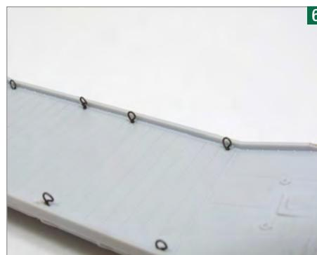
The tie-down rings are cut away and replaced with wire twisted around a 1mm drill bit, then superglued into holes in the deck.
