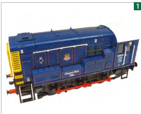
I'm going to re-map the CVs on this Bachmann Class 08 diesel shunter fitted with a Zimo MX645 sound decoder, as shown in parts one and two of this series.
