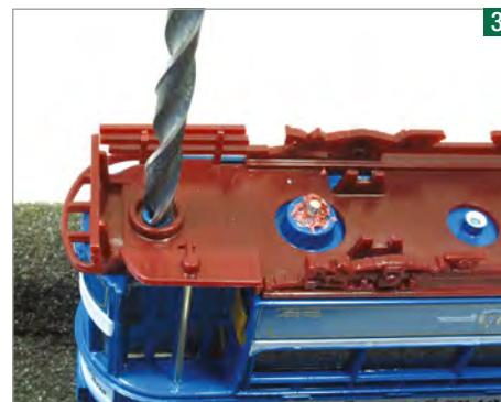
Three rivets heads are drilled away using a 6mm drill bit. The metal is soft so a slow speed power tool such as an electric screwdriver is perfect for the job.
