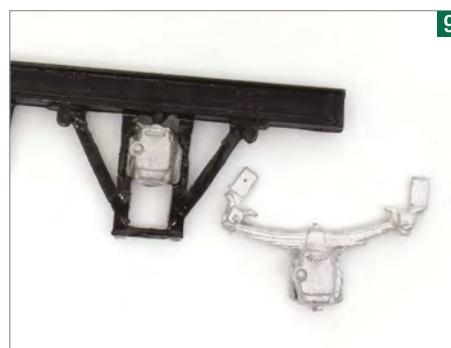
Replacement axleboxes are MJT whitemetal castings without springs. File the back to reduce the thickness, then superglue to the plastic W-irons at the top.
