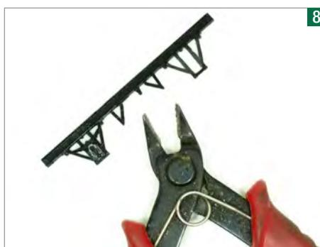
It might look brutal, but the easiest way to remove the axleboxes is with electrical cutters. Chew the box flush with the W-irons, then remove the rest with a sharp knife.
