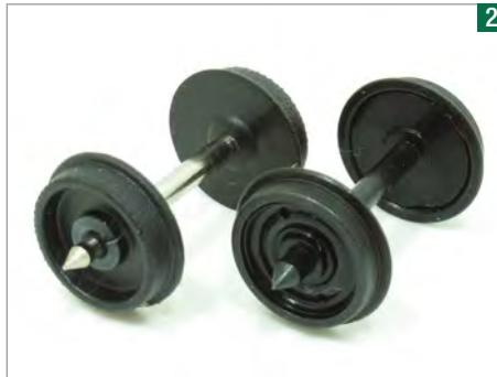
Dapol plastic wheels on metal axles are a big improvement on the original Airfix parts but 10.5mm diameter Keen Maygib metal versions are even better.
