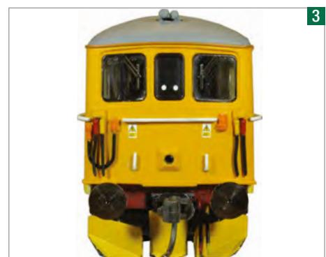
The finished 'inner' end (without lighting) which couples to the train, with Kadee coupler and extra details such as bufferbeam hoses.
