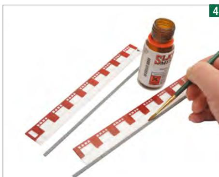
Though the skirts were removed, the coverings for the solebars were retained. After I'd cut off the skirts, I carefully fixed the coverings with Mek-Pak.
