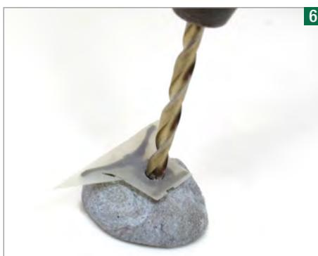
To fit over the bearings, each axlebox has to be drilled out with a 1.6mm bit. Support the fragile part in a blob of Blu-tack and work it carefully with a pin vice.
