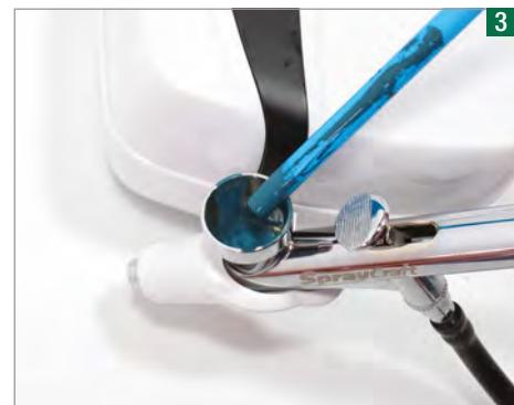
The easiest way to transfer paint into the paint cup is with a drinking straw. Dip it in the paint, seal the open end with your thumb and then drop it into the airbrush.
