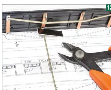
I used bullhead rail to make the trussing - the eye reads it as angle from normal viewing distances. I made a simple plastic jig to give me the height of the king posts.
