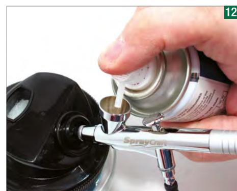
Spray some airbrush cleaner into the cup and then spray some of this through the tool into the cleaning jar. Ideally leave some cleaner in the working parts of the airbrush.
