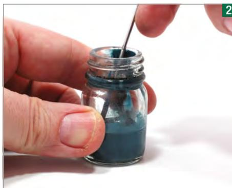
Thin the paint to the consistency of skimmed milk in a container - not the airbrush paint cup. Stir thoroughly, as lumps will block the airbrush leading creating problems.
