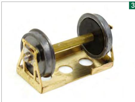
Each wheelset is held by an etched cradle. Just fold it up, with the half etched lines on the inside of the bend and solder - or superglue - each corner for strength.
