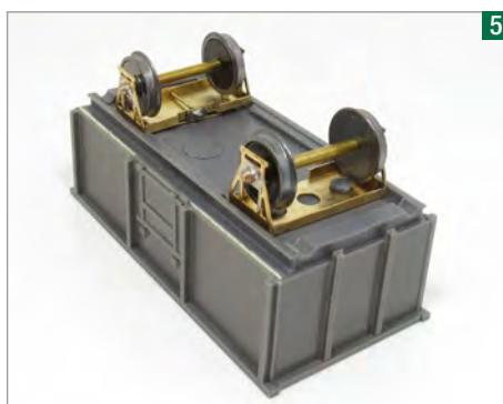
Each wheelset cradle fits over raised lugs under the floor. A dry run is recommended to ensure they sit properly. At this point a quick test run is a good idea.
