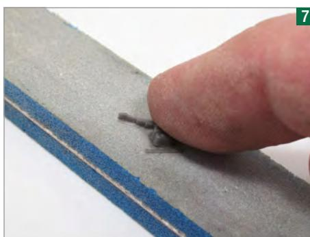
Many of the detail parts are moulded into a thin resin sheet. The instructions recommend removing excess by sanding the backs, but if find it easier cutting it away.
