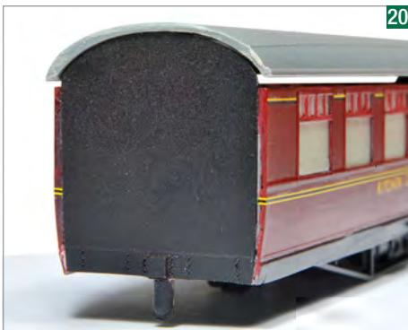
Initial inspection suggested the roofs sat too high at the ends, so I filed and scraped away the underside. Even with this treatment, they still were perched too high.
