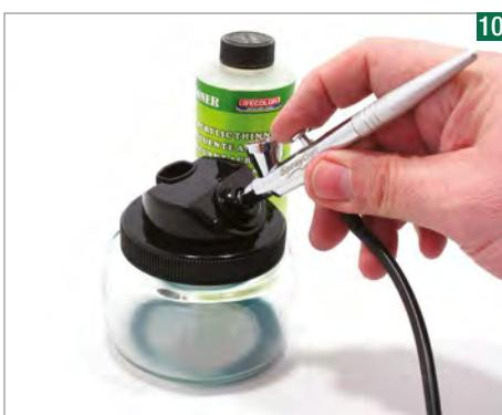
It's vital to clean your airbrush thoroughly. Start by spraying thinners though it, spraying into the cleaning jar to collect the waste and reduce fumes.
