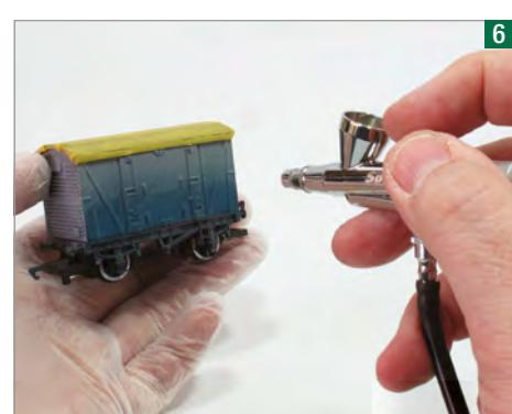
Working on a test wagon, point the airbrush to one side of the model and pull the trigger back. Move the tool sideways, keeping it about 20cm from the side.
