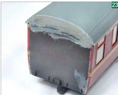
With all the scraping and filing necessary, there were eventually some little gaps left. These were filled with Plastic Padding, then rubbed down and glued.
