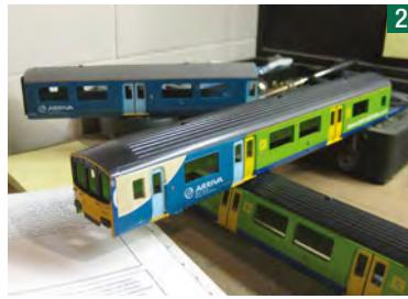
Class 150/1 bodyshell with the new '150/2' section inserted. Note one of the largest sections of the future centre car behind.
