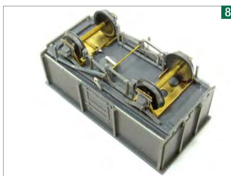
Brake gear is glued in place keeping the shoes in line with the wheels. Before fitting the cross-wire, holes are drilled in both the V-hangers and pivots.
