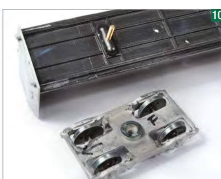
I drilled a hole through the pivot to fit the bogies, tapped it, then fitted an 8BA bolt. A washer was added to correct the ride height for the MJT bogie at the outer ends.
