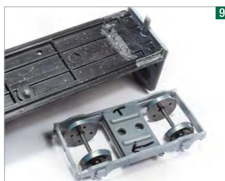
Part of the longitudinal trussing underneath the floor pan needed removal to clear the flanges. This was achieved with a mini drill and dental burr.
