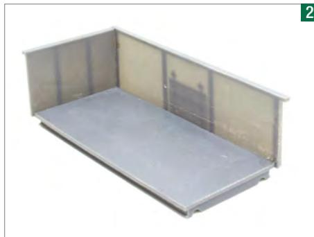
With no aids to locate parts, assembling the sides and ends around the floor needs care and superglue. Start with an end, making sure it is perpendicular to the floor.
