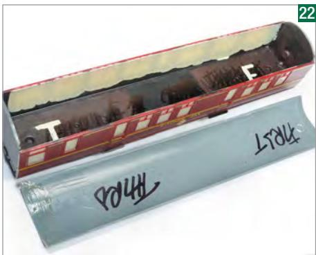
Once 'happy' with the fit, each roof section was labelled with a black marker to ensure they were installed the correct way round.
