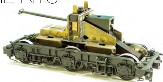
Non-functional details are included where appropriate: for parts which are either missing from, or placed incorrectly on, the original mouldings, or to replace items, most usually brake rigging, that have to be removed when EM or P4 wheelsets are fitted.
