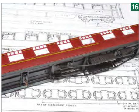
Once the sides were carefully glued onto the frames/ends, the lining was added using Modelmasters' transfers. Some careful joining was called for.
