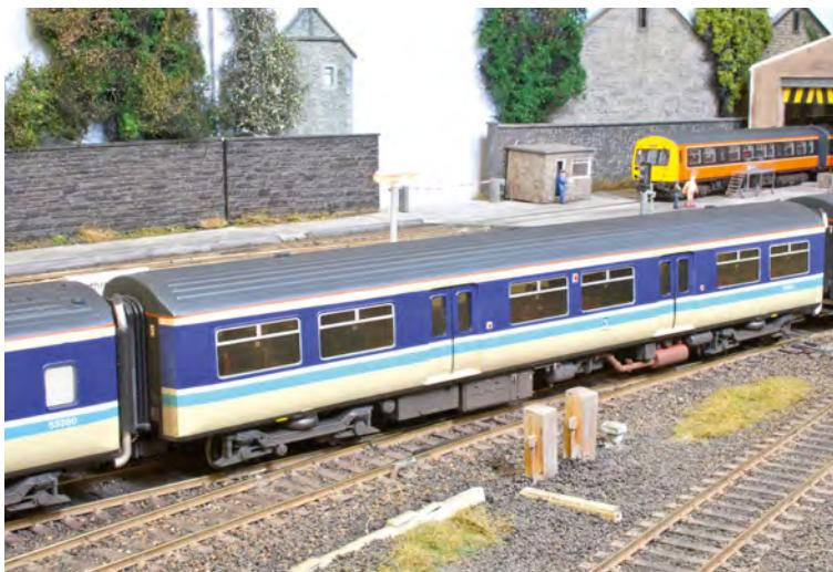
The remaining cab-less two-thirds sections of the Class 150/2 cars were used. The DMS vehicle section, measuring 175mm, needs no more cutting but the DMSL had to donate two sections required to create the centre coach. The centre saloon of the DMSL needs to be cut completely away from the remaining section with cuts made across the whole bodyshell between the passenger doors and adjacent windows. See the supporting schematic at [www.rmweb.co.uk](http://www.rmweb.co.uk) for how this was achieved.
