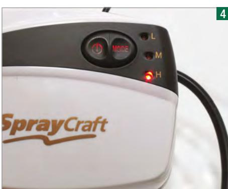
Switch the compressor on and it starts in high pressure mode. Pressing the mode button toggles between the pressures. Low pressures are useful when weathering.
