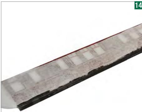
Once the body painting was dry, the sides were masked and the coverings for the solebars brush-painted in Humbrol 85. There should be a slight lip at the joint.
