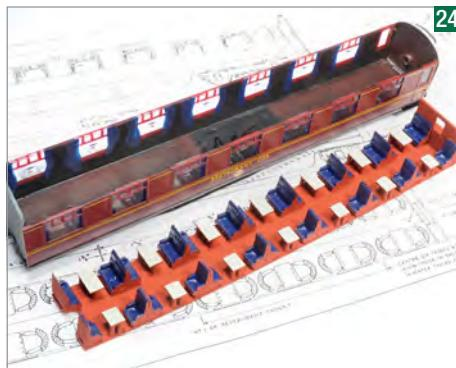
Interiors were made from Southern Pride parts. The original RFO arrangement was 1+1 armchairs, later changed to 2+1 fixed seats.
