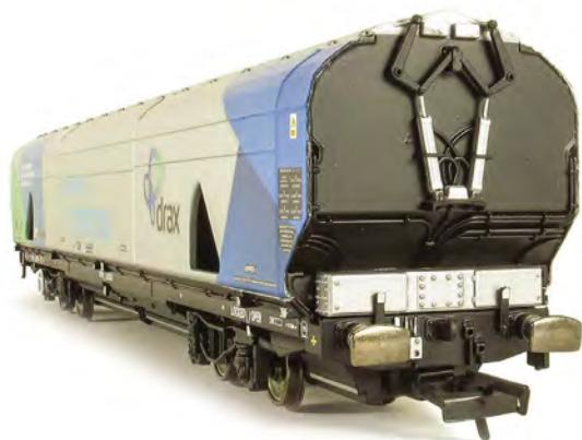
The outward hopper discharge chutes, on which the coupling arms/sockets are mounted, are combined with the bogie which means that they will swing with layout curves, necessary for the models to work on second radius 'train set' curves.
