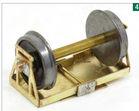
The compensated cradle is similar with the addition of a support. If you solder rather than superglue, apply permanent marker to parts you don't want to solder first.
