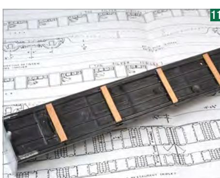
For my period it's necessary to replicate the underframe trussing. I substituted the plastic trussing for metal. PCB was superglued at the appropriate points to mount it.
