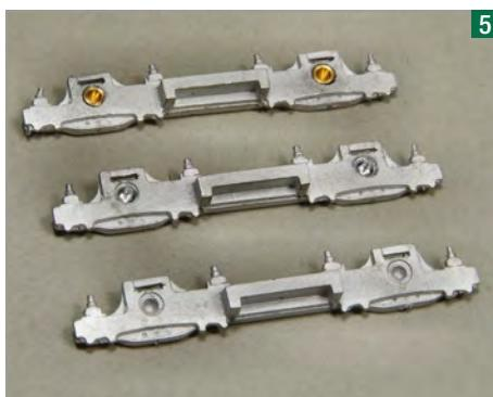
Ian Kirk-type 8ft 6in bogies are supplied for the non-articulated ends but they're not the correct type. I substituted MJT cast-metal ones with top-hat bearings.
