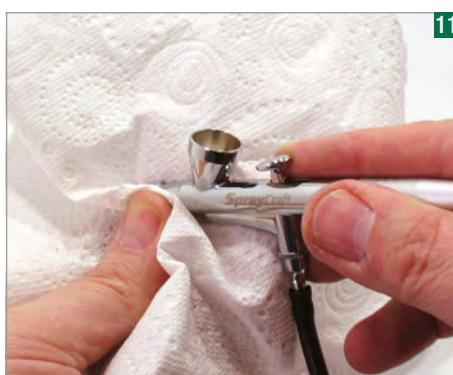
Dampen kitchen towel with thinners and wipe down the outside of the airbrush and the paint cup interior. Cotton buds are useful for reaching small areas in the nozzle.
