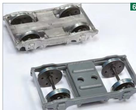
The articulated bogies were 10ft heavy-duty types. I used the plastic ones supplied in the kit, fitting top-hat bearings as I went. Wheels are Markits 14mm disc.
