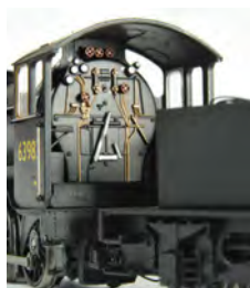
ABOVE: Boiler backhead is more minimalist than some recent efforts in OO, but still has all the required features.
