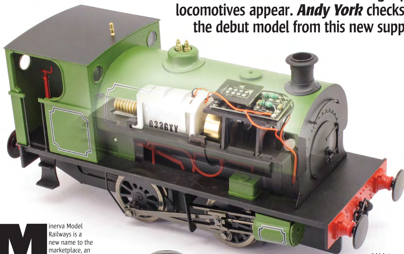
A high-torque motor and flywheel provide smooth operation. There's also an eight-pin DCC decoder socket.
