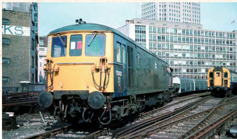
ABOVE: The kind of duty for which it was designed; 73002 shunts Waterloo & City Line stock on to a non-electrified siding at Waterloo on April 6 1978. Until the early-1990s, W&C vehicles were taken in and out of their tunnels by lift and transported by rail to Eastleigh Works for overhaul.
