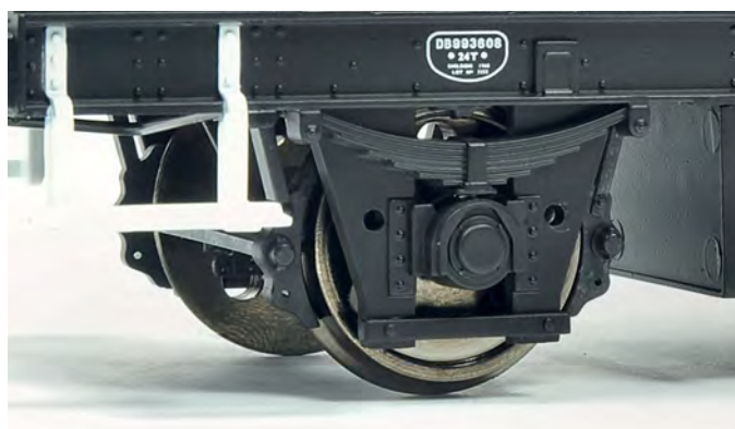
Above The Timken roller bearing axleboxes on the 'Dogfish' differ from the oil types on the 'Catfish'. Perhaps Heljan will produce a model of each with alternate axleboxes. Both are interchangeable if you're willing to separate the bottom of the axle guards.
