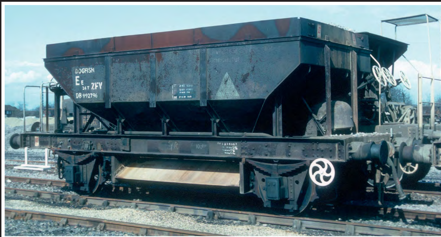
Waste ballast, known as slag, was often re-used by the Eastern and North Eastern Region on secondary routes. During the 1960s, almost a fifth of 'Dogfish' had gin side extensions fitted to the hopper bodies for carrying slag. DB992796 was one, photographed at Hitchin on March 3 1983. PAUL BARTLETT
