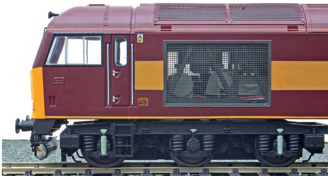
Prototypical 'daylight' and traction equipment is visible through the grilles - a key feature of a Class 60's character.
