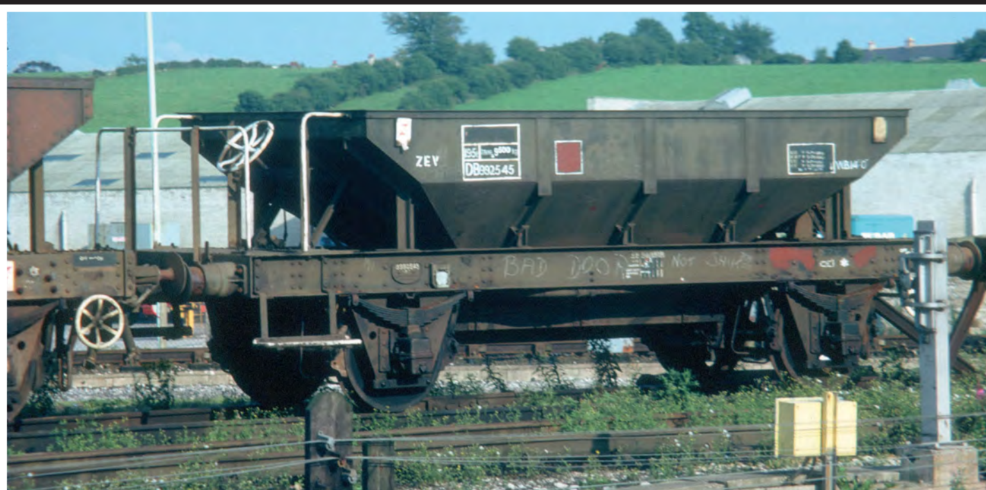
Engineers' wagons didn't live a life of luxury. Seen in its original olive drab livery, DB 992545 has many markings of interest to the modeller. Note the raised OLE warning plates, black and Gulf red patch painted sides and the chalk marking in pigeon English 'Bad door not shut'. Carnforth sidings, August 25 1979. PAUL BARTLETT
