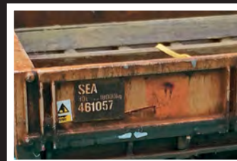
Many of these steel-sided wagons have scars from loading and unloading and frequent rough treatment. I replicated these with a scalpel blade, following prototype photographs to ensure correct positioning.
