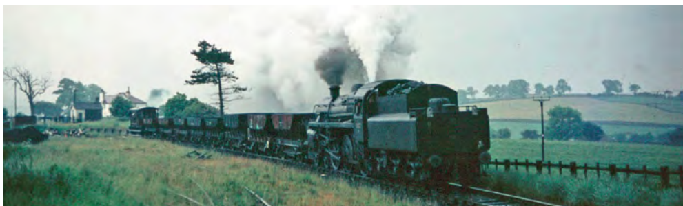
A short engineer's train of the 1960s personified. A BR Standard Class 4 4-6-0 passes through Rylstone on the Skipton-Grassington quarry branch with a train of empty ballast hoppers. The old goods yard sidings can be seen on the left. Amongst the mixed wagon types, the first is a 'Dogfish' accompanied by examples of 'Trout' and 'Mackerel' hoppers. DAVID HEY
