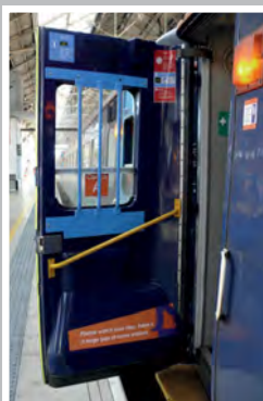
Window bars and safety notices have been added to the Cumbrian Coast Mk 2s as the route features tight clearances, low and short platforms in various locations. BEN JONES
