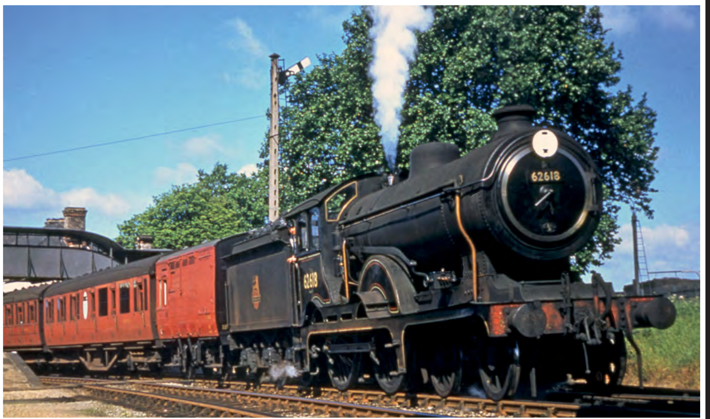
Those D16/3s rebuilt from D16/2 'Super Clauds' generally retained valancing over the driving wheels, including No. 62618, captured at Sudbury in July 1956. Behind the tender is an ex-LNER horsebox, followed by a Thompson non-gangwayed Composite (CL) and a Gresley wooden-panelled non-gangwayed coach, all of which are in the Hornby range. All are painted in BR crimson. COLOUR-RAIL (BRE1949)
