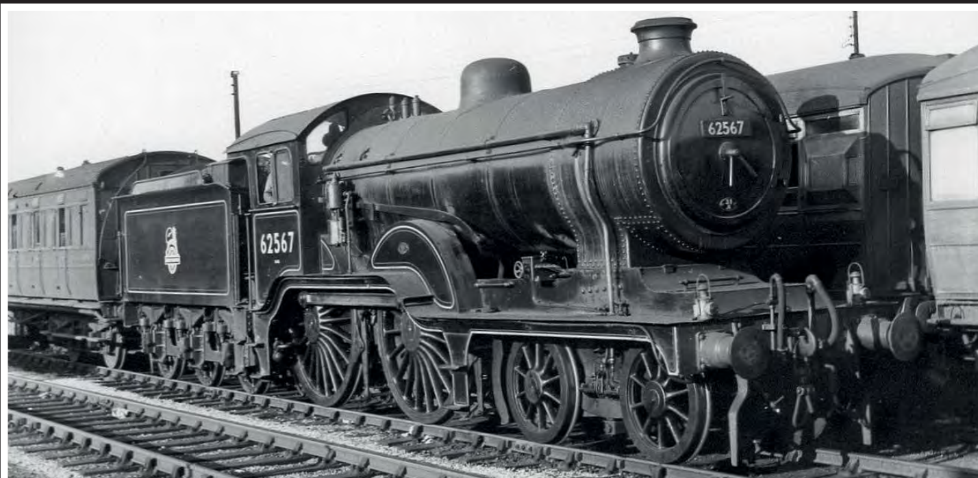
Built by the GER as a D56 in 1908 and rebuilt by the LNER from a D15 after 1933, Cambridge's D16/3 No. 62567 retains its Westinghouse air-brake equipment in this undated view. Not all D16/3s were lined out when painted BR black, many retained plain black until withdrawal. STRATHWOOD COLLECTION
