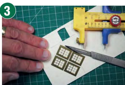
I chose to use etched brass twelve pane sash windows produced by GT Models, which I acquired at an exhibition. These were measured for the cutting of the apertures, using a compass cutter for the curved tops.
