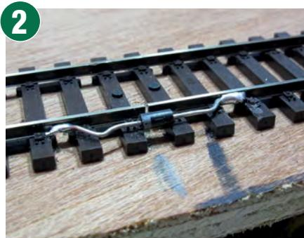
The trains stop when they cross a break in one rail bridged by a diode. This allows them to reverse out of the dead section under control of the shuttle. The Tillig trackwork has chemically blackened rail sides which need to be cleaned before soldering. Mounting the diode beside the track looks ugly, so in areas where it can be seen I've dropped a couple of wires through the baseboard and secured it underneath.
