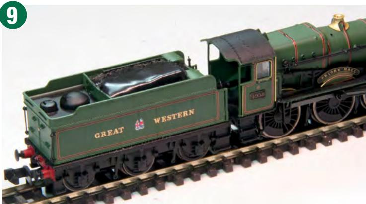
With the decoder covered in electrical tape (overlapping a little to cover the entire hole), press it right through so it sits flush on the motor top and click the tender body back into place. If you've filed the hole enough, it should go perfectly flush. You may need to adjust, or even flip the decoder over to get good motion out of the motor. Once you're happy with the fit, and the motion, reconnect locomotive and tender and test thoroughly before proceeding.
