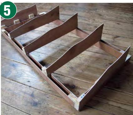
The plywood formers were cut out using a jigsaw. Screw and glue the finished formers to the spacer uprights.
