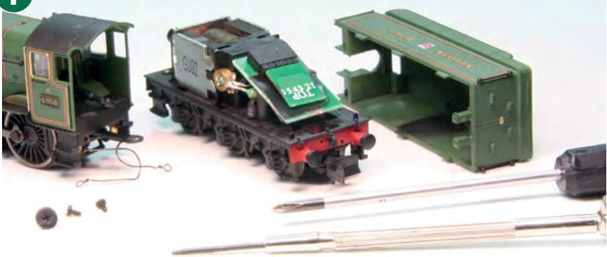
Pop off the tender body, being careful not to break the plastic retaining clips as it lifts off, pressing in from the sides to release the body clips. This reveals the six-pin DCC socket mounted at an angle in the rear of the tender space.
