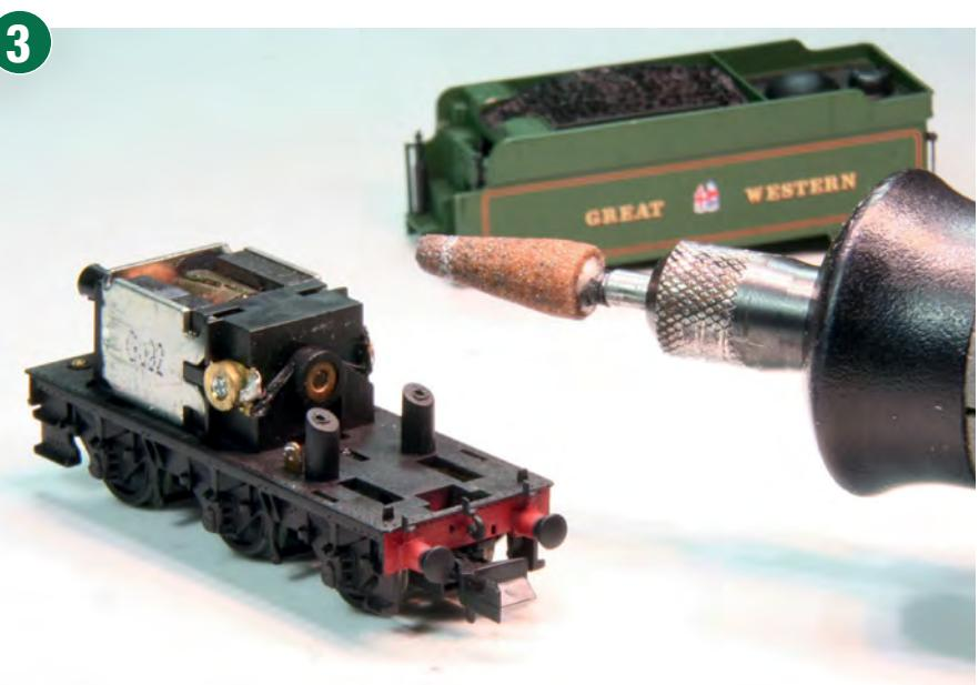
File down the circuit board mounts flat as this is where we'll mount the YouChoos SugarCube7 speaker. The speaker's 15mm x 11mm footprint fits perfectly between the pick-up tabs, and the total height of 7mm is a comfortable fit too - no modification required to the enclosure. You might find it useful to file an angle off the rear of the motor housing plastic to give the decoder wires space, but it's possible to get everything in without doing this if you're neat.
