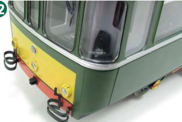
As supplied, the 'buffers' are too rounded. Pulling them away from the body and tweaking them with fine nosed pliers improves their look - the buffer furthest away is original, the nearest has been flattened. When they came into contact with anything on the prototype, a certain amount of bending changed the shape even further.
