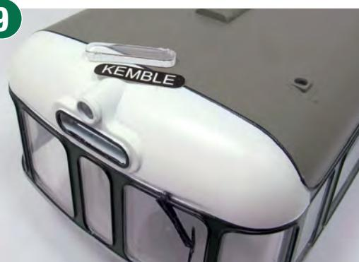
Changing the destination blinds starts by popping out the old ones. Push them from the inside with the end of a wooden paintbrush handle. It might be possible to lever the plastic out carefully from outside but there would be a risk of damaging the roof paint.
