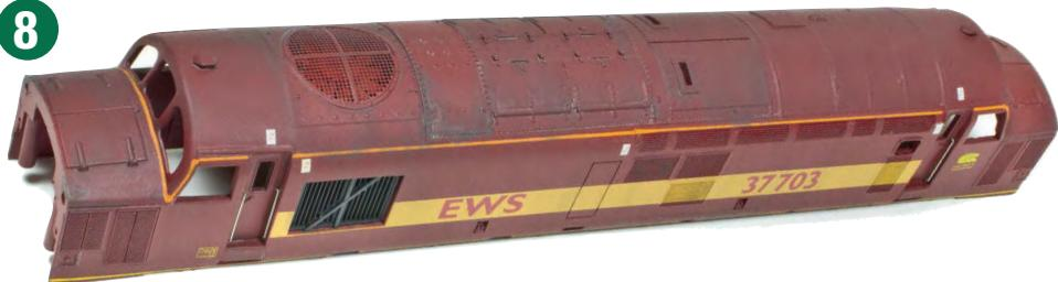
Grimy paint collects in moulded detail and along raised panel lines. It tones down the bright livery and highlights Bachmann's fine tooling work without making it appear too dirty. The grime wash was followed up with exhaust and frame dirt applied sparingly with an airbrush.
