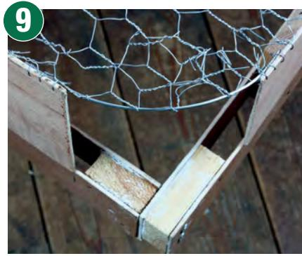
I wanted a curved backscene to avoid any unsightly corners. I used a piece of wire as a former to work the chicken wire mesh to shape.
