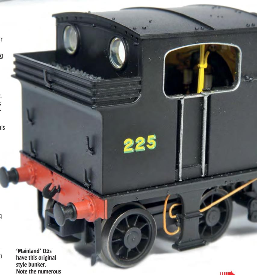
'Mainland' 02s have this original style bunker. Note the numerous separate detail parts.
