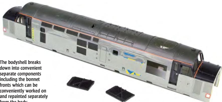
The bodyshell breaks down into convenient separate components including the bonnet fronts which can be conveniently worked on and repainted separately from the body.
