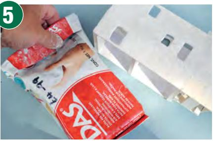
The clay was applied in the same way as the bridge, until a skin covered all the walls. The clay was left for around 24 hours to dry before scribing it, starting with the corner quoins and the lintels over the windows and doors. The apertures can all be cleaned out with a small file later.
