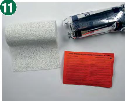
The wire mesh is covered in plaster bandage to form a light, but strong shell. I used two of the Javis packs to cover a 36" x 18" area.
