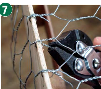
Use pieces of 0.6mm (approx.) wire to hold the chicken wire mesh in place. Twist the wire using a pair of pliers until the slack is removed.
