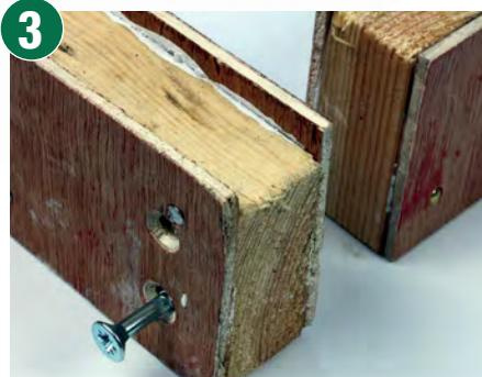
The side and end runners were screwed and glued together. Ensure that the screws bite into the side and not the end grain of the 2" x 1" spacers. Pre-drill the holes to avoid splitting the wood.
