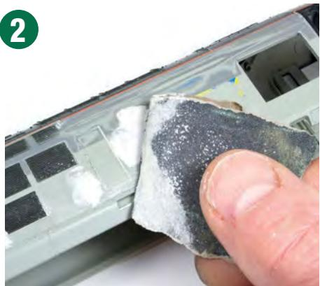
Squadron white putty is applied to the unwanted detail and the window openings before being finished with grade 800 and 1200 wet-and-dry paper. Any filler which has entered the door seams is carefully removed with the tip of a modelling knife blade.
