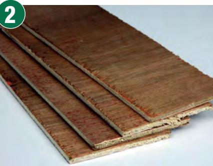
Since the baseboard measures only 36" by 18", I used 3mm plywood. The wood yard cut some of the board into strips to match the 2" x 1" timber I used for the rest of the framework.
