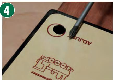
The delay between trains can be set from 20 to 70 seconds by twiddling a control under the sticker in the shuttle unit. A small cross-head screwdriver is required for this. The instructions recommend operating the unit before adjustment which seems a good idea.
