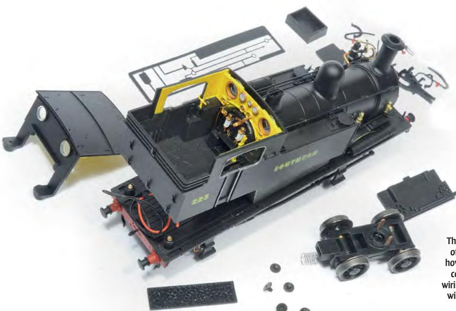
This 'exploded' view of the model shows how the components come apart and the wiring provided if you wish to install a DCC sound speaker.
