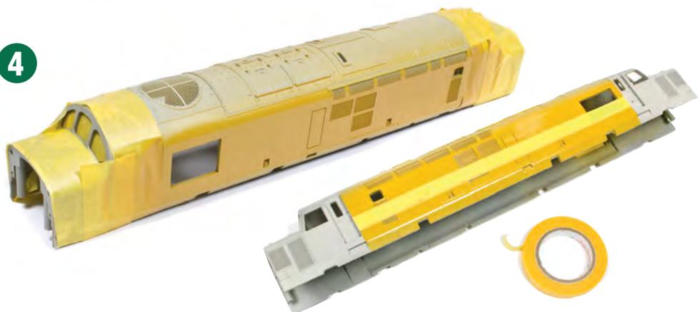
A second coat of grey primer is applied to the model which makes the perfect base coat for EWS gold paint which does not cover dark colours particularly well. Two light coats of EWS gold were applied, allowing at least 24 hours drying time between each. Particular care was taken to be sure the paint was completely hardened before applying masking tape to the body in preparation for EWS maroon.
