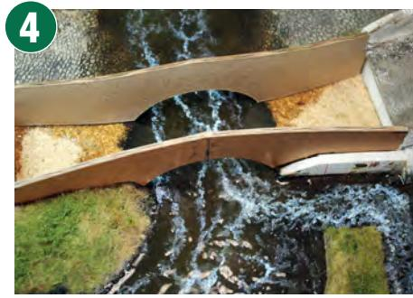
The two sides of the bridge were bent to profile. These are placed into position and secured by cutting and gluing in a spacer made from 5mm foam board.
