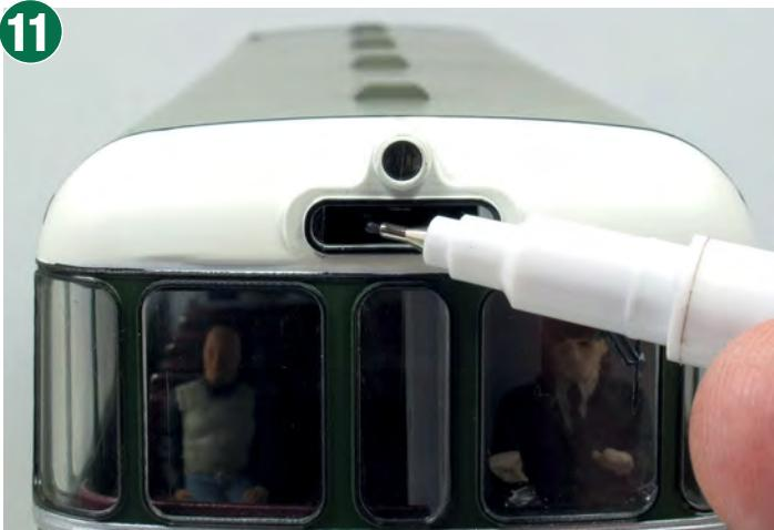
Heljan's destinations have nice rounded ends. Cutting these perfectly is fiddly but colouring the plastic with a CD marker pen avoids any white showing through if the job is less than perfect.
