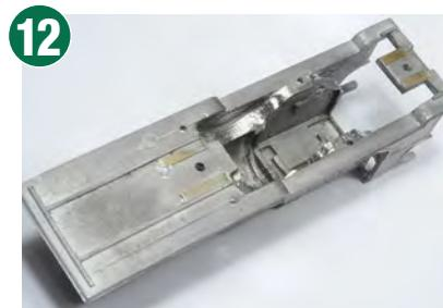
12 I also needed to lift the whole body up on the chassis, just to give the necessary clearance so that no binding/shorting occurred. This was achieved by soldering on four small pads made from scrap brass etch. The internal metal removal from the underside of the splashes is evident.
