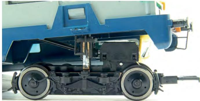
Above We've 'jacked up' the chassis frame here to show the cardan shaft, gearbox and current collection arrangement of the bogies. All four axles are driven and this, coupled with the weight of the model, means there's no need for tration tyres.
