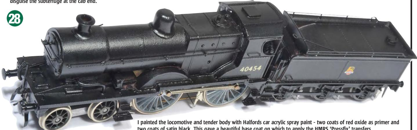
I painted the locomotive and tender body with Halfords car acrylic spray paint - two coats of red oxide as primer and two coats of satin black. This gave a beautiful base coat on which to apply the HMRS 'Pressfix' transfers.
