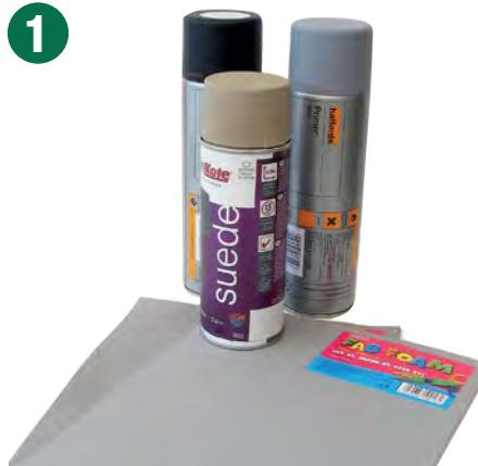
The surface of the 'Fab Foam' is sprayed with a mixture of spray cans. Grey primer, satin black and tan Plastikote suede touch give a variety of grey and brown tones. Look at the tones of road surfaces around you for inspiration to avoid the repeated error of a model road being too dark or uniform.
