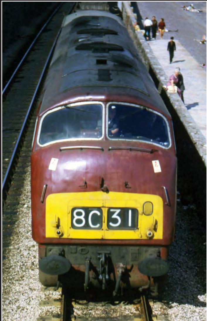
**D857 Undaunted** pictured in July 1966 at Dawlish in maroon small yellow panel livery shows the offset exhaust vents and the North British style walkways over the roof grilles. This image also shows the difficulty of placing the overhead warning flashes in a non-vertical position. COLOUR-RAIL
