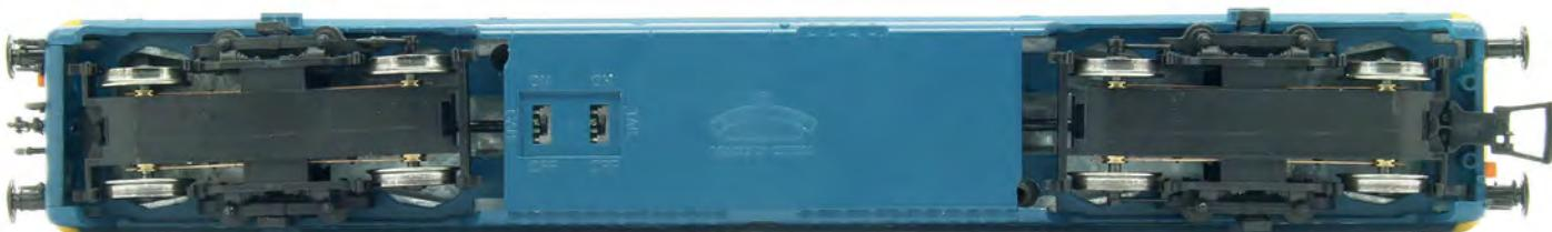
The underside of the model features the on/off switches for the cab and tail lights. The axle mounted track current collecting bushes can be seen too.
