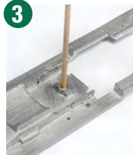
The footplate was very cleanly cast and needed very little in the way of flash removal and no filling-in of surface blemishes. As prescribed in the instructions, the two 8BA nuts for fixing the chassis to the body were soldered in place, held with a cocktail stick.
