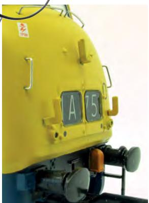
The '43' accurately depicts the cranked mounting of the WR lamp brackets on the nose. The circular air vents beneath the headcode boxes are accurate in size and position for D842 and are reproduced by printing onto the nose surface.
