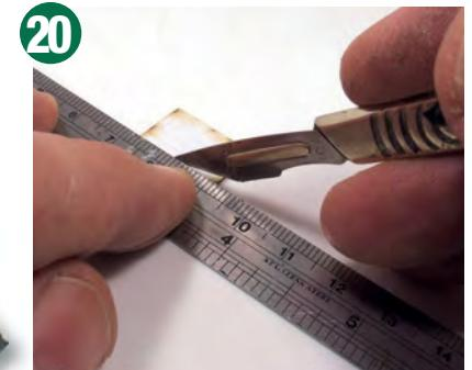
One problem with the laser cutting process is that it only produces detail on one side of each component. Where both sides are on show, such as with the wheelbarrow, I scribe the plain sheets with a blunt knife to add planks.
