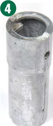
Both boiler halves matched quite well, though there was still a slight depression where the two met at the top. I soldered the pair together, then filled the depression with low melt in a series of small 'blobs', finally filing down to the correct shape.
