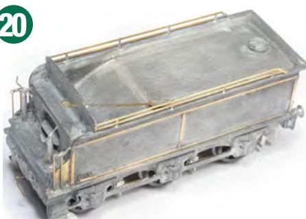
The completed tender. The two triangular bits designed to prevent coal spillage from the footplate were cut from brass shim and soldered in place before adding the vertical handrails. Different styles of coal rails are supplied to cater for the varieties amongst these tenders.
