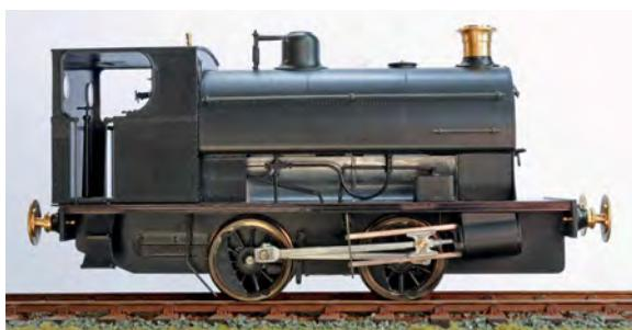
**T**he first production samples of Minerva Models' O gauge Peckett E class locomotives are now being checked. To date, only CAD drawings and specifications had been given, but progress to the tooling stage and evidence of a prototype model is proof that the project is well underway.
