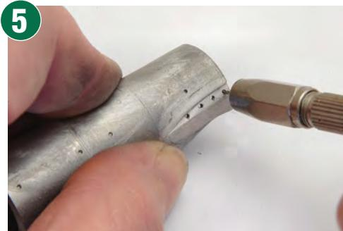
Because I was changing this locomotive to a right-hand drive (Midland-built) example from a left-hand drive (LMS-built) one, the cut-out in the boiler cladding to take the reversing lever had to be filled in. Solder was impractical, so I first drilled holes in the cut-out to give the filler a key, then used Plastic Padding to fill the cut-out, finally paring it down once it had cured. I finished it off with some files and wet and dry to match the boiler radius.
