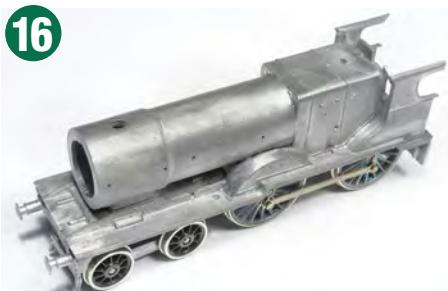
16 With the bogie sprung and forcing the front end back up, the locomotive was then nicely balanced and ran very sweetly. One compromise I had to except was the footplate valance not being recessed enough - Midland-built 2Ps had the valance much further in, though it's right for an LMS-built one.
