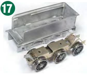
17 As already mentioned, an SE Finecast MR-style tender was used. Like all Finecast's whitemetal tenders nowadays it comes with an etched chassis which ensures accuracy and thus achieves good running. Clearances between the outside frames will only suit OO, though.
