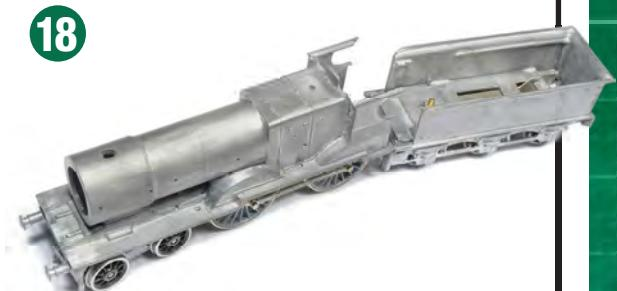
18 With the locomotive and tender in their respective part-built states, the pair was checked for mutual compatibility. At this stage the guard irons were still fixed to the bogie, as supplied and prescribed. They should be fixed to the frames - see later.
