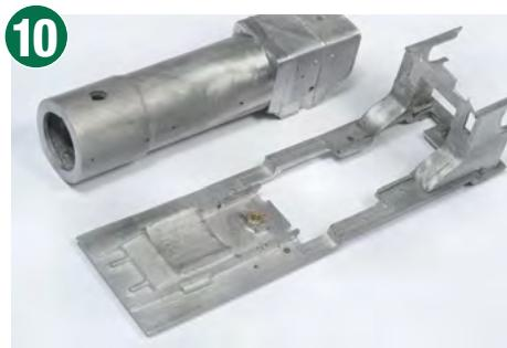
10 The cabsides and spectacle plate fitted with a minimum of cleaning up and were easily soldered in place. The relative fit of the boiler/firebox to the footplate was also perfect, resulting in a very rapid build thus far.
