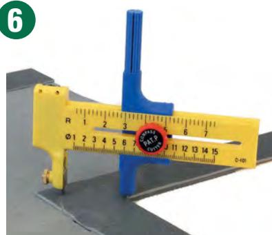
I'm curving the edge of the pavement with a compass cutter, in this case set to the same radius as the width of the pavement at 32mm. It's quite a tight turn for a junction, but not unknown in built-up areas.
