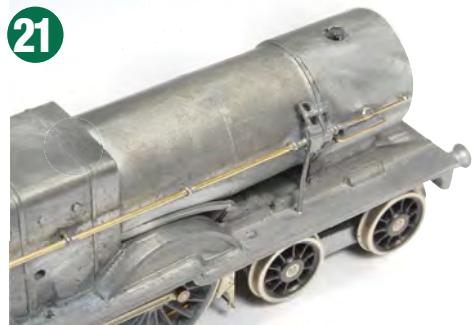
Because the locomotive was to have right-hand drive, I ordered the appropriate steam gubbins from SE Finecast from the firm's 4F kit. This was beautifully cast in one piece. The reversing lever should be slightly recessed - I made provision for this before fixing the boiler to the firebox.
