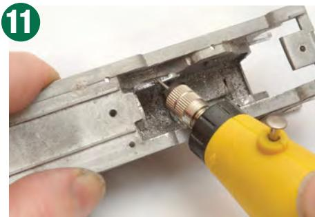
11 The earlier-built locomotives had larger driving wheels, so there was interference between the inside of the splashes and the flanges. Even though the driving wheels weren't quite as large as they should be (6' 10" instead of 7' 0"), the dental burr (using the BRM subs gift) was resorted to.
