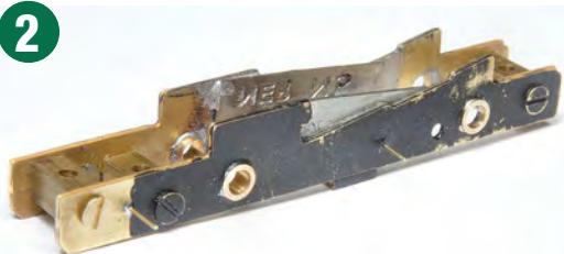
A new etched chassis is to be provided in the 'production' kits, so work such as this - the filling-in of the cut-out with scrap etch - will not be necessary. However, this method might be of use to others who have such chassis still lurking in the backs of cupboards.
