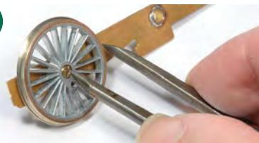
To get this particular kit 'off the ground' so to speak, the original etched-brass Millholme frames were supplied. These date from antiquity, having a cut-out for an X04-type motor and no provision for brakes. I thus plotted the positions for the hangers using sprung dividers.
