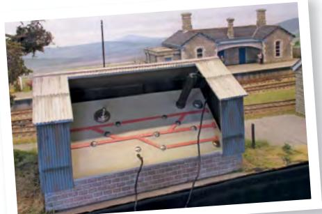
Above Points are controlled by the traditional 'stud and probe' method and cleverly housed in the back of a storage shed.
