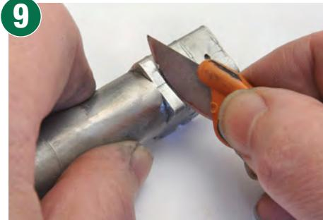
Having soldered the boiler to the firebox (please note the neat seam along the top of the boiler), attention was turned to cleaning the joint along the top of the firebox. There was a very slight depression and this was made good by paring with a Swann-Morton craft knife.
