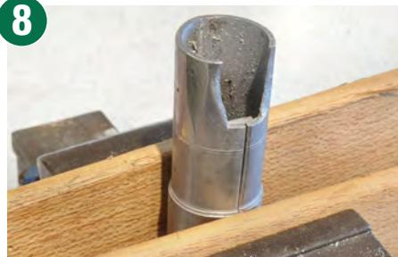
Once happy with the fit of the boiler, I noted that it wasn't true-round. The easiest way to put this right was to squeeze the boiler into the true-round using a medium-sized vice. Because its jaws are serrated, it was essential to use scrap wood 'cheeks' to prevent damage to the soft metal.
