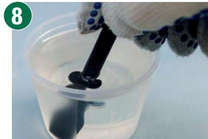
Two parts of the resin is mixed to one part hardener, as advised, to cover the area. The mixture is stirred until both liquids are translucent.
