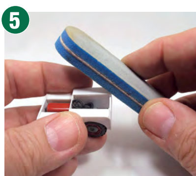
Once dry, the plastic top corners are rounded with an abrasive stick.
