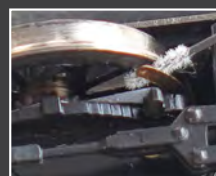
The micro brush is ideal to apply Track Magic onto the current carrying contacts of the point
