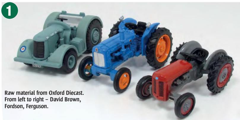
For each model, the rear wheels need to be removed. Gently twist them with your fingers and the axle will pull out of one wheel. The mudguards can be pulled off, they will break so be careful to remove all the plastic around the square axle end.
