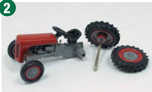
For each model, the rear wheels need to be removed. Gently twist them with your fingers and the axle will pull out of one wheel. The mudguards can be pulled off, they will break so be careful to remove all the plastic around the square axle end.
