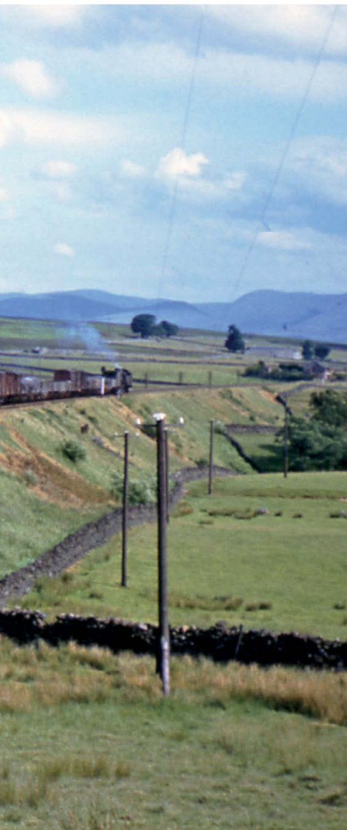
The second wagon behind 'Black Five' No. 44937 is an example of a 'Hybrid High' fitted with a sheet rail for tarpaulins – in this case raised but without the sheet fitted. This mixture of opens and vans, captured on April 2 1966 at Brisco, near Carlisle, is typical of BR era vacuum-braked general merchandise trains. COLOUR-RAIL
