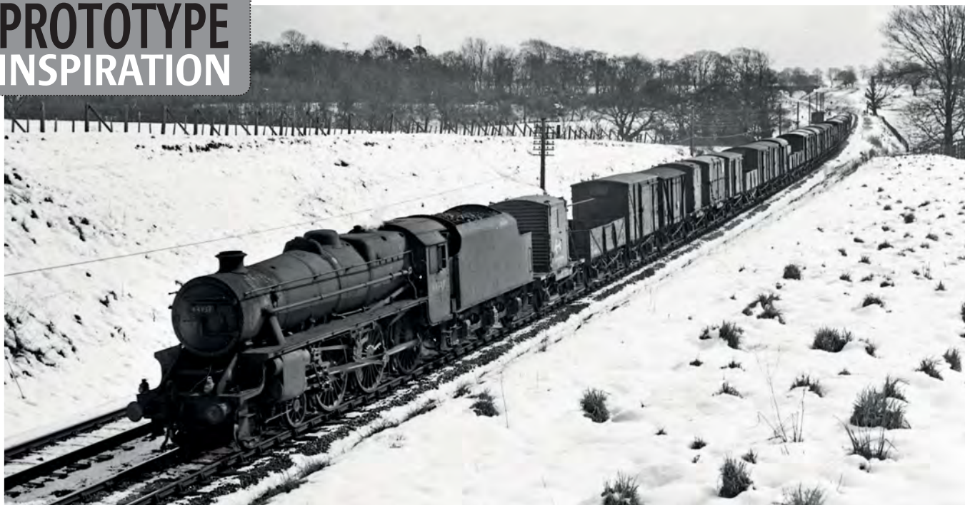
The second wagon behind 'Black Five' No. 44937 is an example of a 'Hybrid High' fitted with a sheet rail for tarpaulins – in this case raised but without the sheet fitted. This mixture of opens and vans, captured on April 2 1966 at Brisco, near Carlisle, is typical of BR era vacuum-braked general merchandise trains. COLOUR-RAIL
