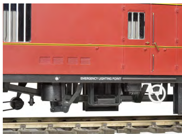
The underframe of the model. A little daylight can be seen between the trussing and chassis. The battery boxes hang a little too low, but not enough to offend the eye.
