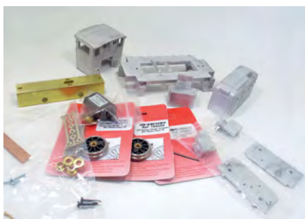
Inside the box there are some very large castings, a length of brass channel for the chassis, wheels, motor and gears plus lots of separately packed detail parts. In the bottom you will find lengths of wire and clear plastic sheet.
