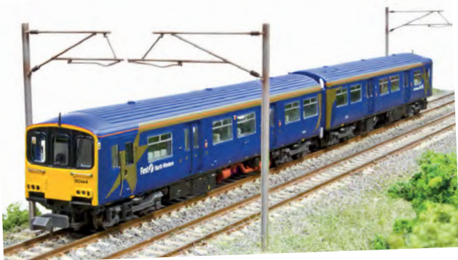
One of the two Class 150/1s is sacrificed to provide the parts to make a new centre car, a process known as cut-and-shut. A Class 150/2 could also be used, with the sliding cab door mouldings saved for the DMS and DMSL.
