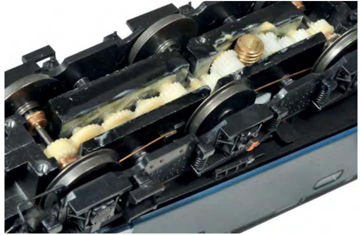
Complicated or what? The system of nylon gears transferring power to each outer axle. For such a heavy locomotive, could this prove problematic? Only time will tell...
