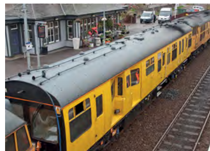
A view of the roof of DB999508 showing the position of roof vents and water pipes.
