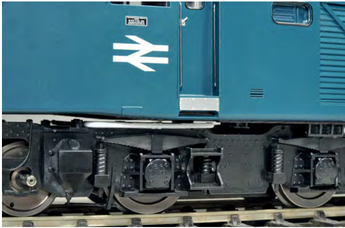
Superb bogie detail is given. 'BR TIMKEN - MADE IN ENGLAND' can be read on each axlebox cover, around which can be seen a fantastic selection of nuts and bolts.
