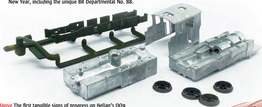
Above The first tangible signs of progress on Heljan's OOg gauge Lynton & Barnstaple Manning Wardle tank were these castings for the body and various plastic mouldings for the frames, detail parts and wheels.
