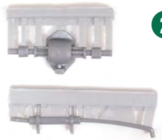
One of the limitations of the resin moulding process is that substantial runners have to be removed from each casting. A small pair of wire cutters will remove the main excess material with a sharp knife used for final clean up. Be careful not to remove supporting brackets when doing this, they aren't that obvious on some parts.
