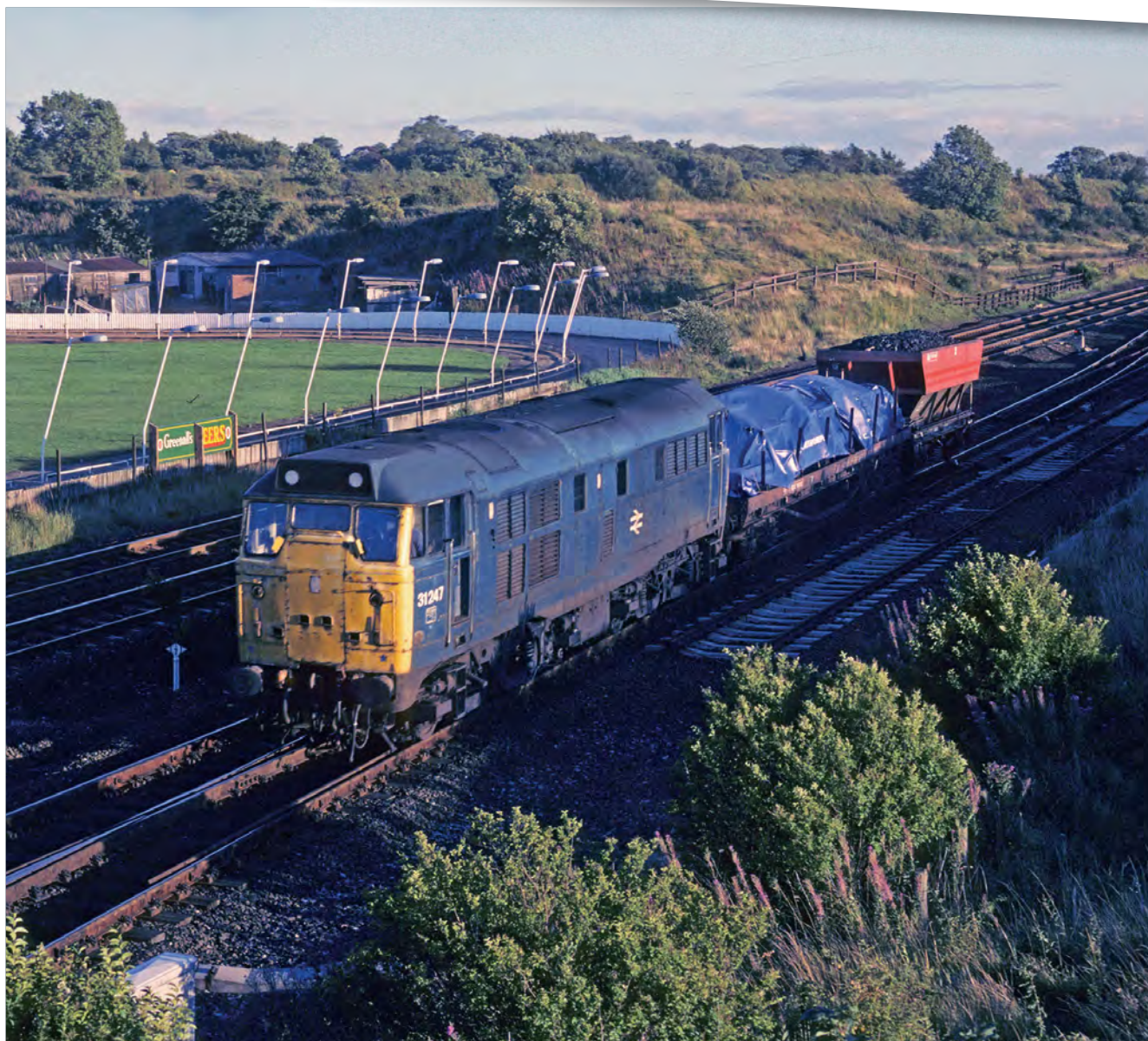
Tyneside: Amazingly this two wagon train is 6S63, the Scunthorpe to Aberdeen Speedlink, seen here in 1985, behind 31 247 at Ouston Junction, south of Tyne Yard. The first wagon is a BDA bogie bolster (Bachmann/Farish) carrying steel from Scunthorpe, whilst the second is a Railfreight HEA coal hopper with coal from South Yorkshire coalfield, attached at Doncaster for domestic depots in Scotland.
