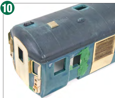
It is inevitable that some remedial filling work will be required. Squadron putty is ideal for this task. Note that the cab fittings have been added to the cab front.
