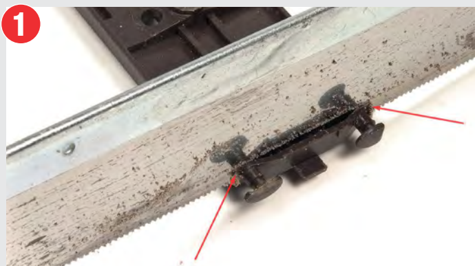
The headstocks of the Mk 2d coach model are the wrong shape. Correct them by removing with a razor saw and rebuilding with styrene strip.
