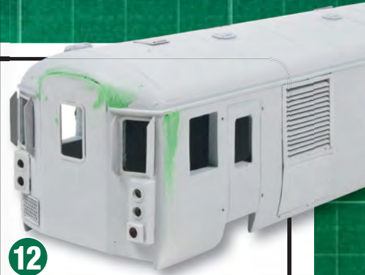
An initial coat of light grey primer reveals any faults in the fitting of components such as the gangway plate and in the bodyshell. A little more filler and a final smoothing down with wet and dry paper tidies things up. I was unhappy with the cabside windows and re-profiled them with the help of a couple of pieces of styrene strip. It is easier to make these changes before painting starts.
