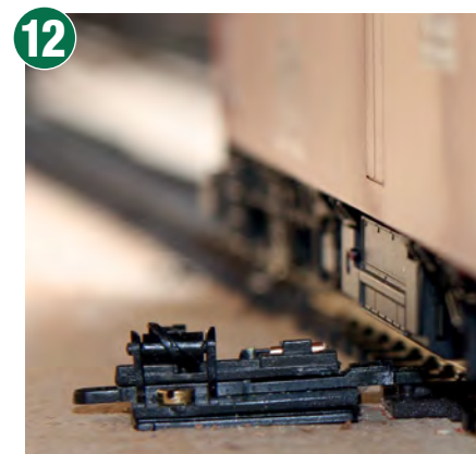
The clearance test, making sure one of the longest vehicles on the layout, with the greatest overhang will clear the ground throw.
