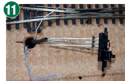
Soldering the polarity wires to the contact strips.
