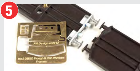
The headstocks can be rebuilt from styrene strip and fitted with extended oval coach buffers. Fold the obstruction guard supplied with the PH Designs kit to shape and glue it behind the headstocks.
