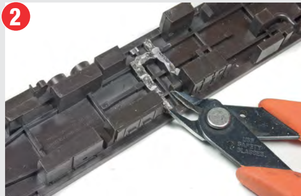
Xuron snips make quick work of chopping away the pressure ventilation ducting – Mk 2f stock does not have this feature. Finish off with a sharp scalpel.
