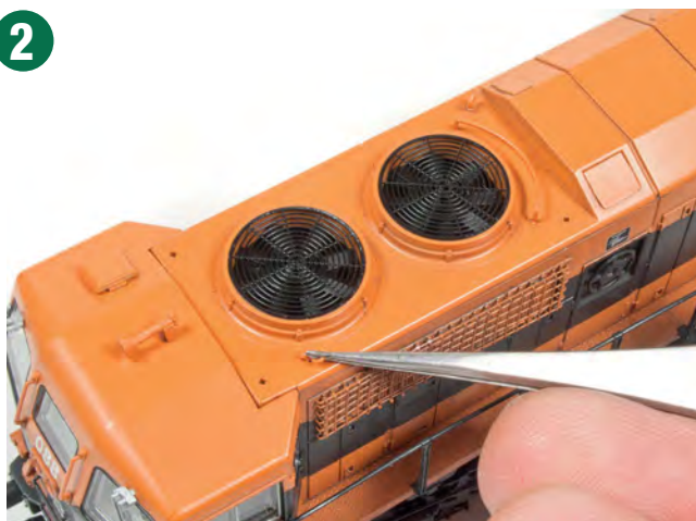
Each lift ring moulding is fitted to a square hole. It is too large to accept metal lift rings and should be filled with a piece of square section styrene before a hole is drilled through.
