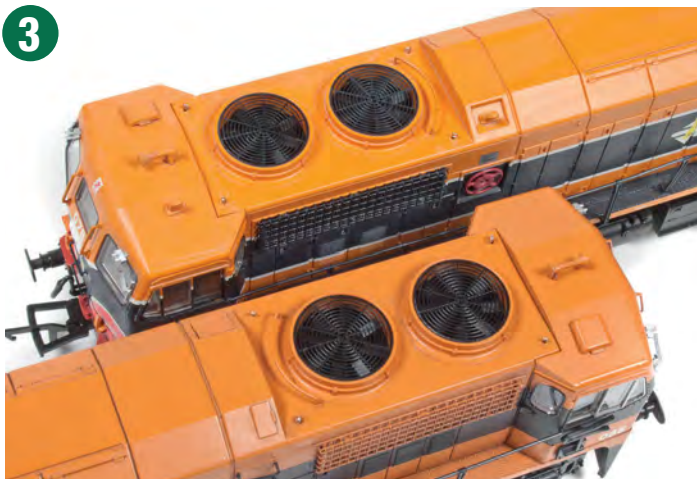
New metal lift rings are fitted to 0.45mm diameter holes and secured with a tiny spot of CA glue (superglue).
