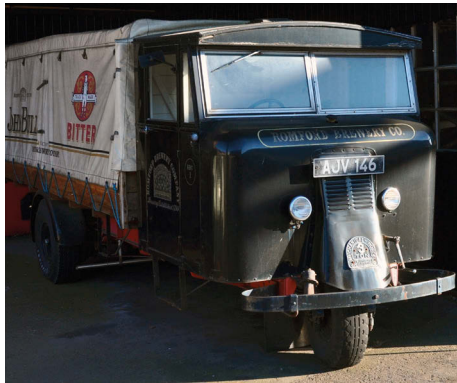
A Scammell mechanical horse. This Romford Brewery Company vehicle isn't an original, but was re-created in the 1970s using the original Scammell drawings and specifications.
