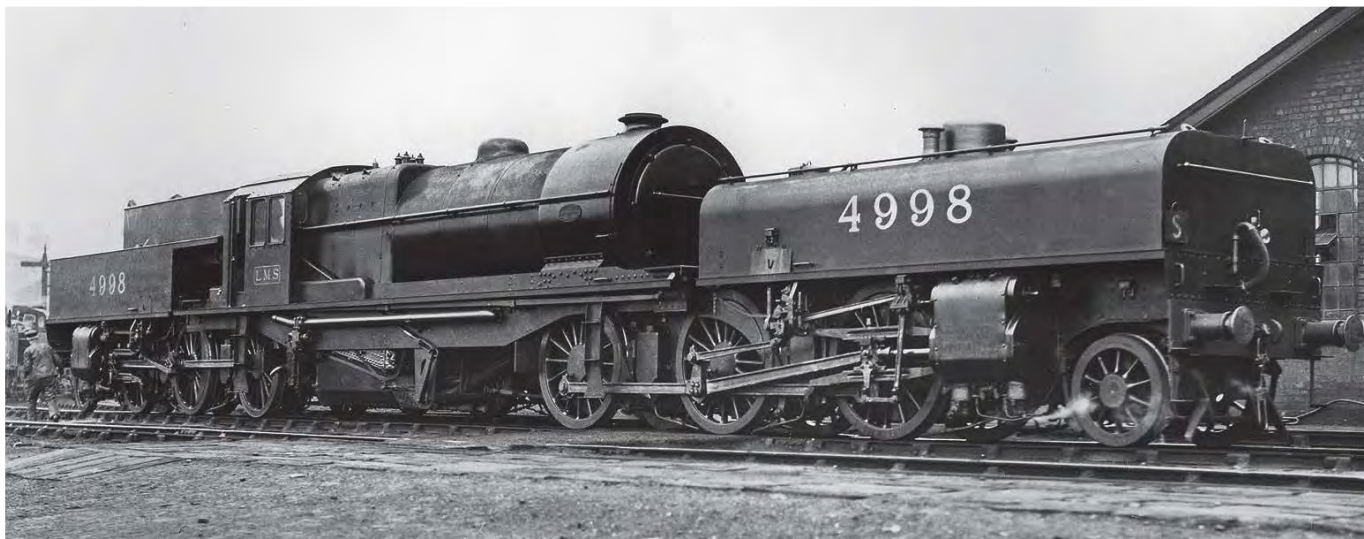
A superb portrait of LMS No. 4998, one of the three 1927 prototypes in original condition with small water tanks and bogie brakes. RAIL ARCHIVE STEPHENSON
