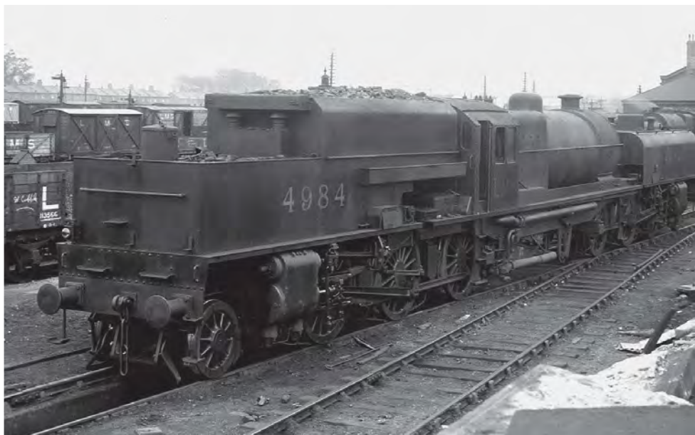
A rear view of No. 4984 in original condition showing the lengthy coal bunker, fire iron trough and a host of original 1930s details, as seen on Hattons' new model. RAIL ARCHIVE STEPHENSON
