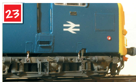
A close up of the loco end showing the test fit of the body-to-bogie shackles, the buffer plates and bogie height 'sit'.
