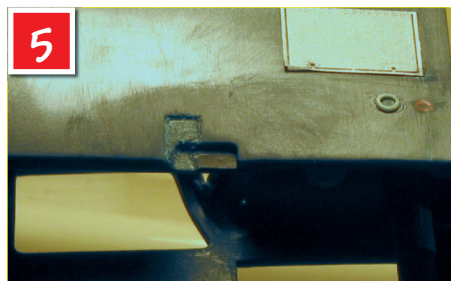
Material removed under the lifting point cover to allow a flush fit, and the recess opened out for the shackle hook and brake lever.
