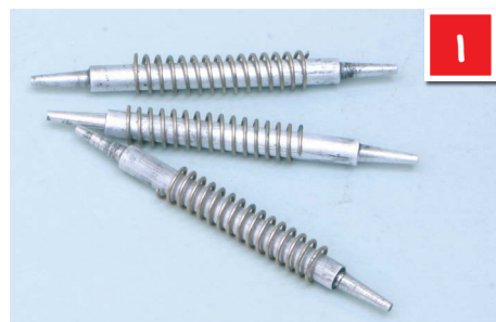
Alignment axles - these from Metalsmith come with compression springs to aid the fitting of hornguides.
