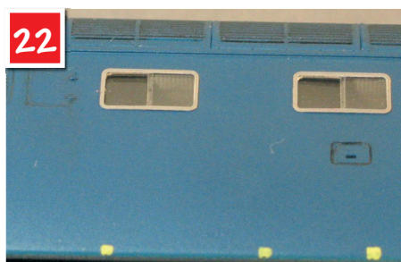
Laserglaze bodyside windows and etched frame surround, all secured using Johnson's Klear.
