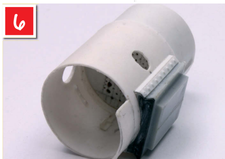
6 A new smokebox was fabricated, but the saddle was cut from the original part and reused. See the techniques' section for more information on this.
