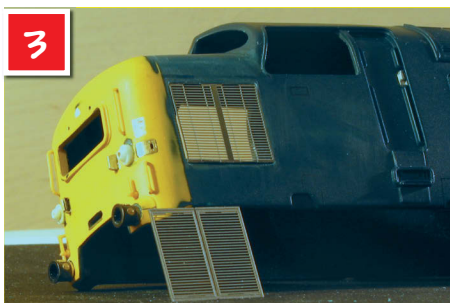
The inner etch for the nose section grille with the outer section alongside during a test fit.
