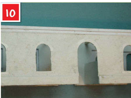
Leave the clay skin at least 24 hours to completely dry before scribing - I use a blunt 10A blade and old toothbrush to brush away the powdered debris.
