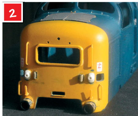
Holes cut for the new sandbox covers; bonnet top doors on re-profiled nose, scratch-built marker light housings; revised buffer beam opening and buffers; etched headboard brackets; 0 and Hornby class 50 buffer housings.
