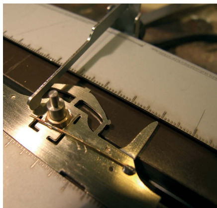
Adding springing to the centre axle.
