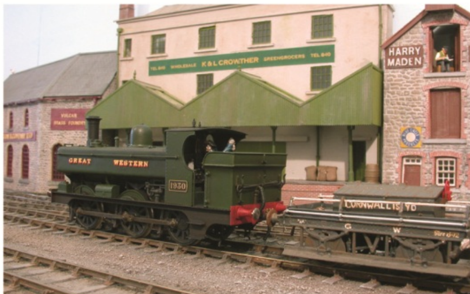
The loco now looks better with its rods weathered, though the eagle-eyed may spot that the injector pipework has been painted black in error, since corrected (see photo at bottom of previous page).
