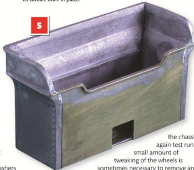
Below: Close-up of the bunker assembly showing the combination of cast white metal and etched-brass components. Attaching the thin, etched bunker front to the cast portions proved a little tricky, achieved by attaching L-shaped pieces of scrap brass to the rear, inside edges of the bunker front. Once glued, a spot of filler was necessary, in places, along the junction between the two parts. The beading along the bunker front top was added using a piece of shaped 0.45mm brass wire, filed flat along its surface once in place.
