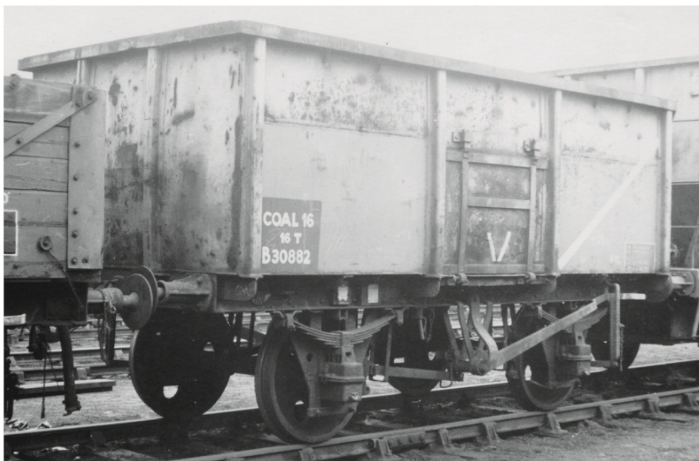
This 16T mineral is one of the former Ministry of Transport wagons and was issued with BR Diagram 1/102, as it does not have the side flap doors. Photographed at Hoo Junction yard in March 1969, the sides have been given new plates, where the fresh paint is, but is otherwise in original condition. Author, WT294/DL
