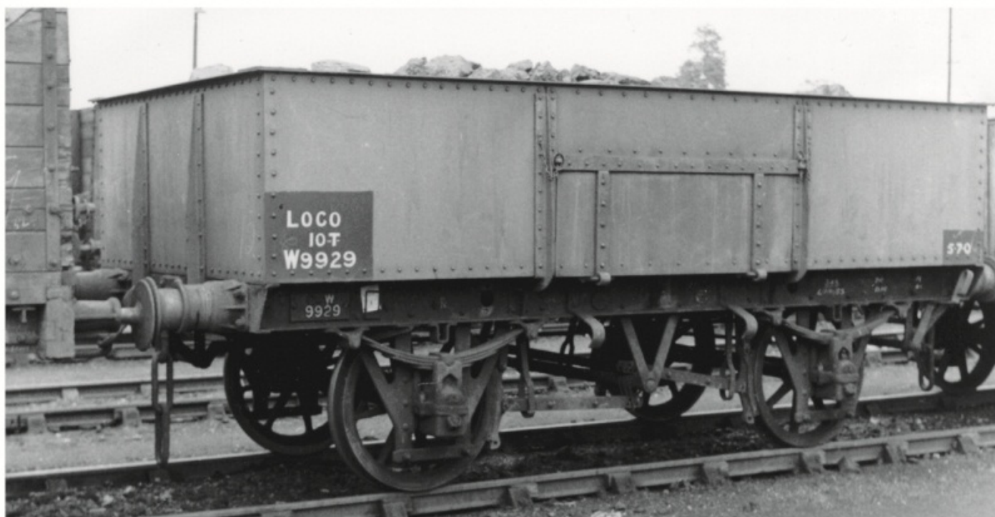
The Great Western Railway had the largest number of locomotive coal wagons and Diagram N'20 is one of the smaller designs. It would have been seen at any former GWR loco shed. Taken at Swindon, early 1950s. Roye England, courtesy Pendon Museum collection
