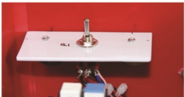
Switch shelf complete with switch. Note the P written to remind me which way to set for programming.
