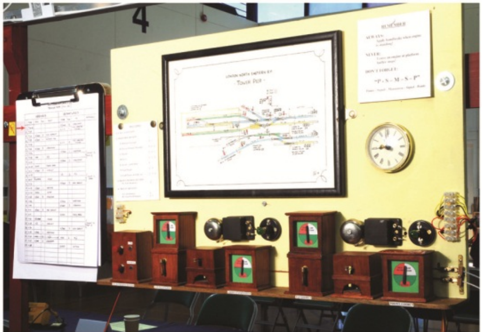
The instrument shelf, track diagram, clock and timetable. There are two sets of instruments for the passenger and goods lines, the tunnel through to St. Katherine Docks is controlled by the plungers on the far left. The bells are dolls house bells and buzzed rather than 'tinged'. I replaced them with house bells fixed behind the board but couldn't get them to sound differently to recognise which were ringing. In the end I settled for one bell with a light which is flashed to tell the signalman which line is being referred to.
