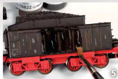
5 Now we dampen the surface with the alcohol.
