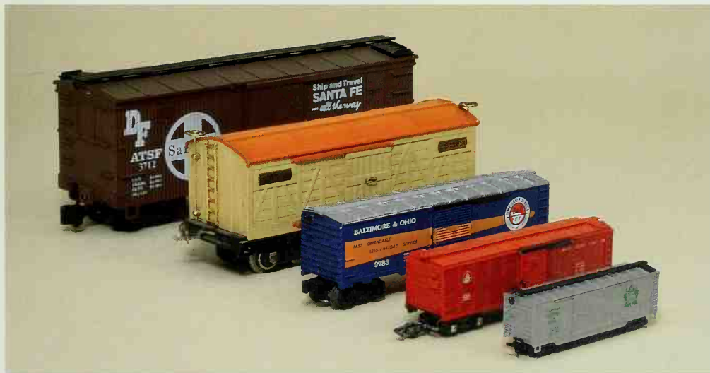
Size comparisons of the various popular toy train gauges. Looking from left to right, you can see G, Standard, O, S, and HO gauges.
