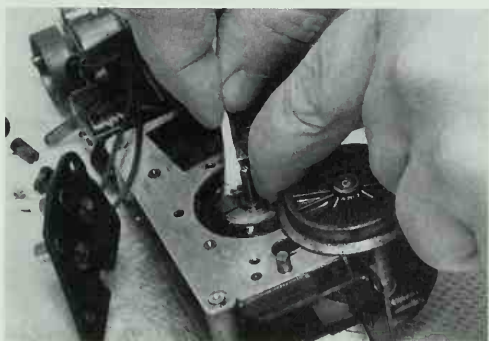
Top: Spray the commutator face with TV tuner cleaner and mop up with cotton swabs. Bottom: Repeat this procedure until the swabs stop picking up dirt.
