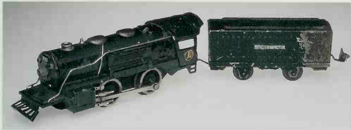
This battered Lionel O gauge 259E locomotive was an excellent candidate for full restoration. The author discovered it in a junk box at a local train meet.
