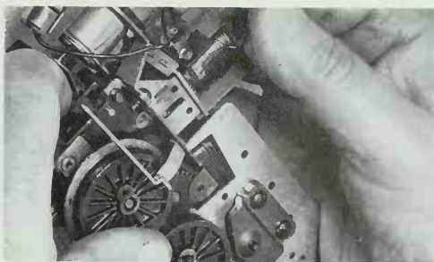
The reverse unit is that coil of wire with a lever attached to it. Remove it with care.
