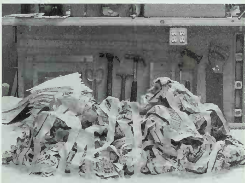
First, position the newspaper wads in the general contour you want and lay strips of masking tape over them to hold them in place.
