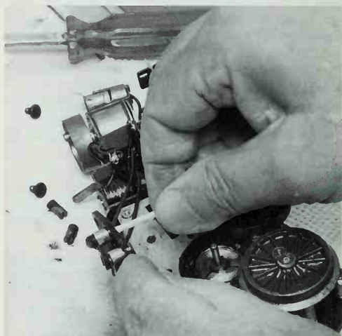
After removing the brush plate and brushes, clean out the brush wells with a cotton swab soaked with solvent.
