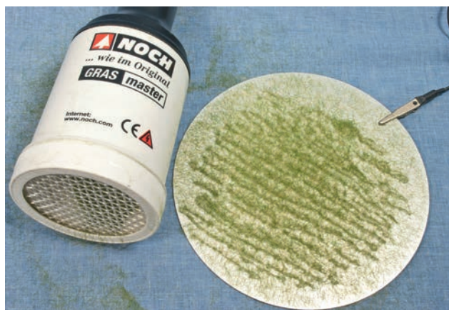
↑ The finished tufts are left to dry after the grass has been applied using a static applicator. They will be easily peeled off the metal sheet.
