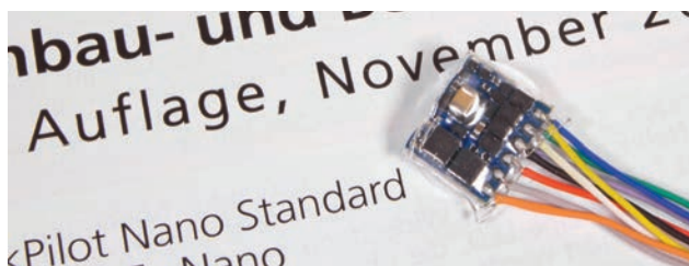
↑ Tiny decoders are also available for the smallest of locomotives with good power ratings and durability, but they can be expensive! The ESU Nano 'Standard' is feature-rich double-sided measuring 8mm by 7mm by 2.4mm with one high spot of 2.8mm. It is available as a wired decoder (shown) or with a NEM-651 6-pin interface.
