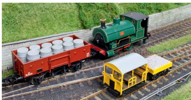
↑ There is a conflict between model size and the need to fit more than a decoder for reliable operation without potential stutters and stalls. The smaller the locomotive, the more likely it will need a stay-alive in addition to a decoder. Yet space is tight because such models also need as much weight as possible! Researching the choice of decoder will be important to achieve the best result.
