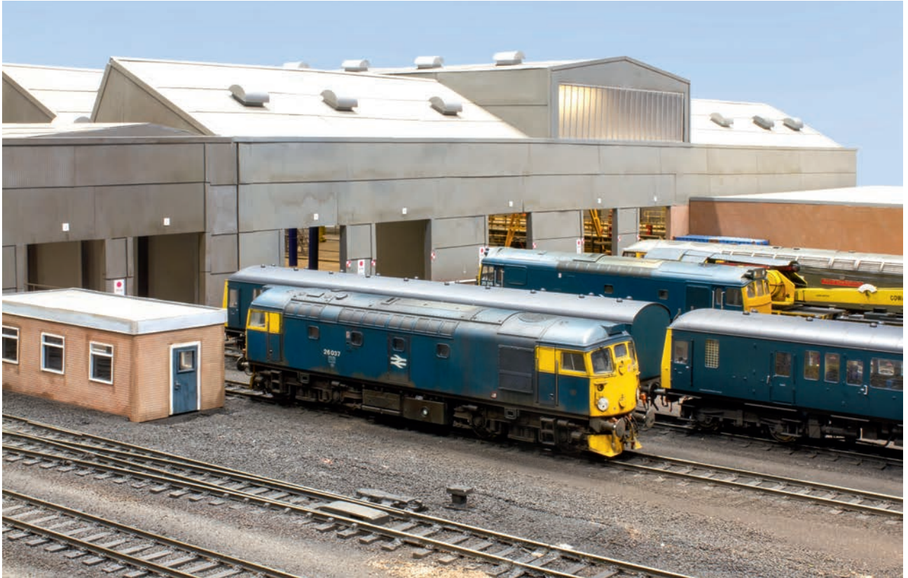
↑ The depot building was constructed using a mixture of known dimensions and measurements worked out from photographs. It too is built from a mix of styrene and foam board. The interior is lit and detailed.
