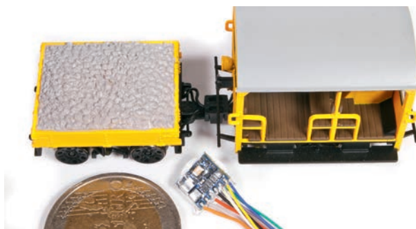
↑ The smaller the model, the greater the challenge of finding and fitting a suitable decoder. The Bachmann 'OO' gauge Wickham Trolley has no DCC interface which requires a hard wire installation of a decoder. The logical place for it is in the trailer.
