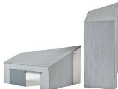
↑ The models of modern works buildings are clad in corrugated material and painted various shades of grey using Tamiya acrylic paint. Points to note are the angled roof lines which allow the buildings to sit at an angle to the backdrop and where the building sub-assemblies fit together.
