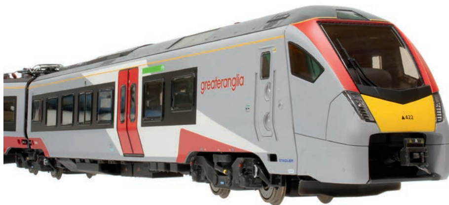
↑ One of the driving cabs of Class 755/4 unit No. 755422 showing its working front coupling and large curved windscreen.
