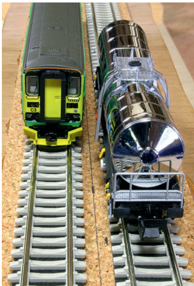
↑ Track laying is complete, ready for it to be painted. The sleepers of flexible track can be painted at the work bench if desired, but not the rails if it is to be curved at any point. Paint will impair its flexibility!
