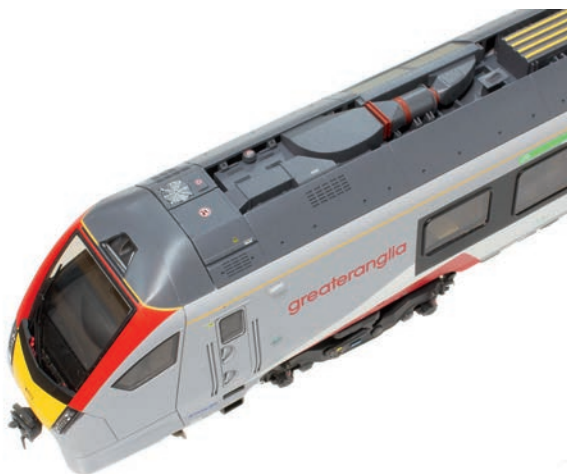
↑ The roof of 'Flirt' vehicles is flat with side panels to protect the array of equipment modules for the electrical systems and air conditioning. On the model, cabling is a mix of moulded conduit and separate details. All of the larger items of roof equipment is applied as separate modules and fittings.
