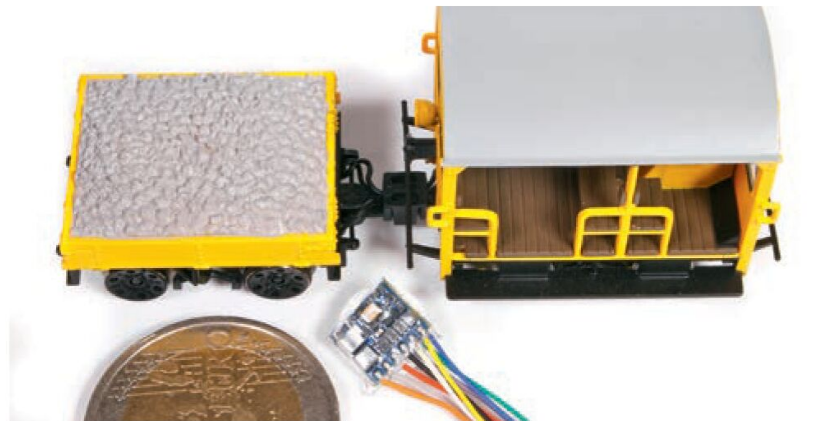
↑ The smaller the model, the greater the challenge of finding and fitting a suitable decoder. The Bachmann 'OO' gauge Wickham Trolley has no DCC interface which requires a hard wire installation of a decoder. The logical place for it is in the trailer.
