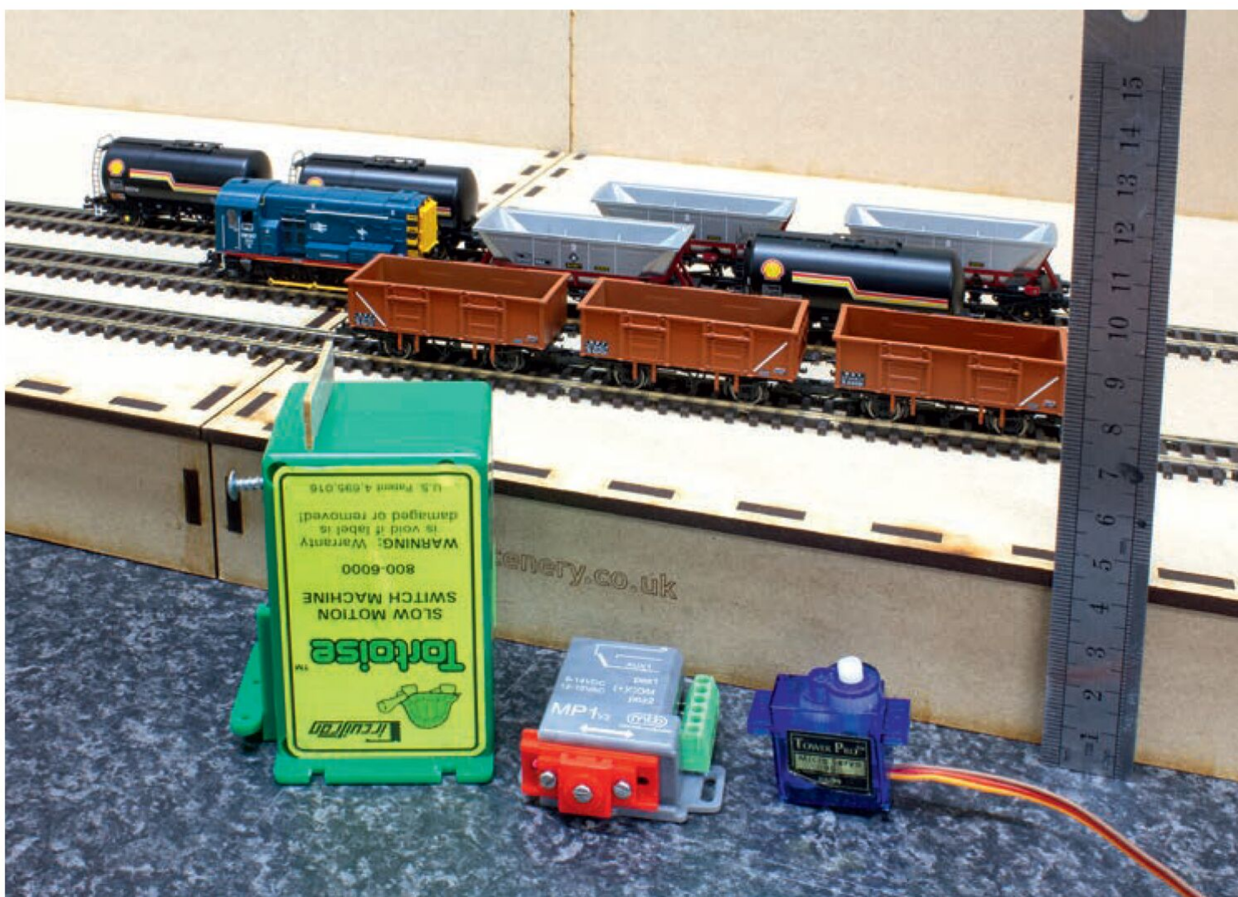
↑ The low 40mm plinth which supports the baseboard top is deep enough for small point machines like the MTB range, servos and solenoid motors. A deeper fascia will be needed if the larger Circuitron Tortoise point motors are to be used, even when placed on their sides.
