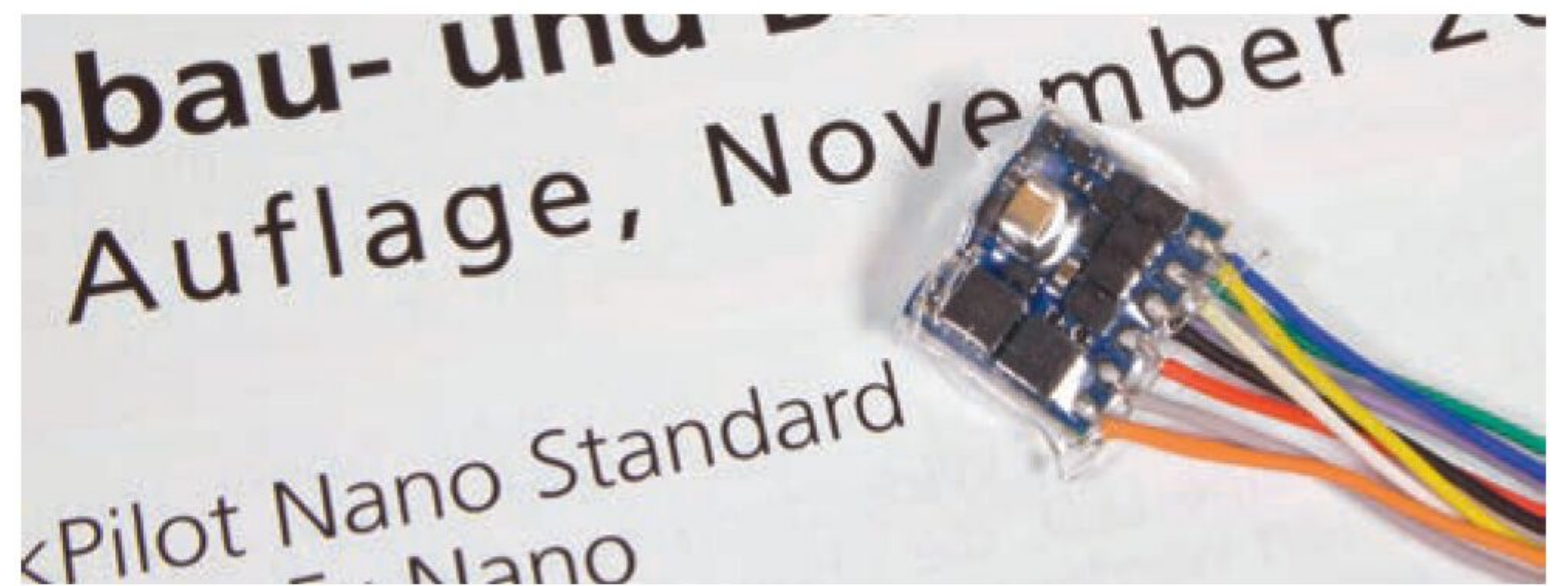
↑ Tiny decoders are also available for the smallest of locomotives with good power ratings and durability, but they can be expensive! The ESU Nano 'Standard' is feature-rich double-sided measuring 8mm by 7mm by 2.4mm with one high spot of 2.8mm. It is available as a wired decoder (shown) or with a NEM-651 6-pin interface.
