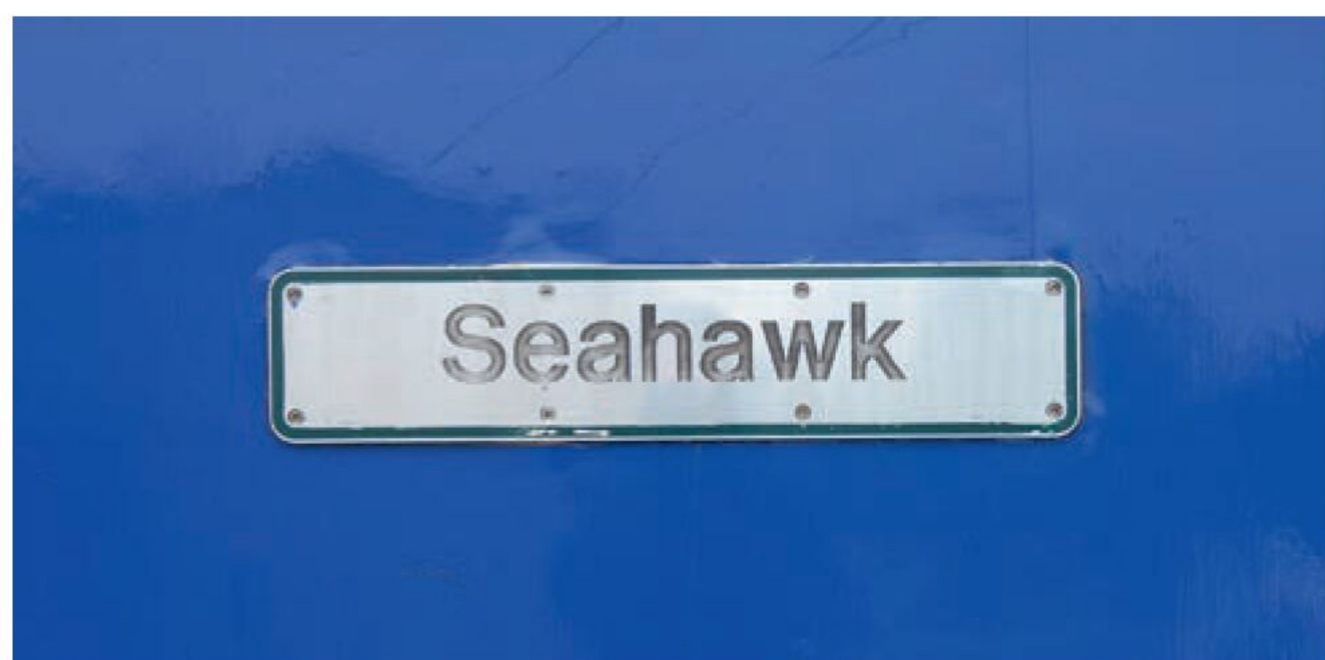
↑ Not all modern traction nameplates are of cast metal. You will find names applied as vinyls and the InterCity version was a slim design made from polished metal. They survived on HST power cars and electric locomotives long after privatisation. This is the nameplate applied to Great Western Class 43 HST power car No. 43191.
