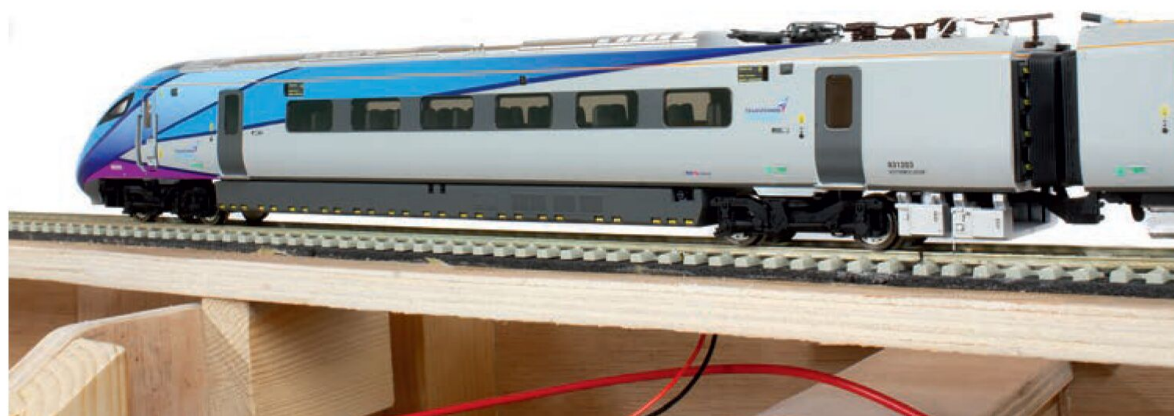
↑ The DPTS vehicle or Coach A. Note the tinted flush glazing, pantographs and neatly printed passenger information screens which display details of a Newcastle-Edinburgh Waverley service.
