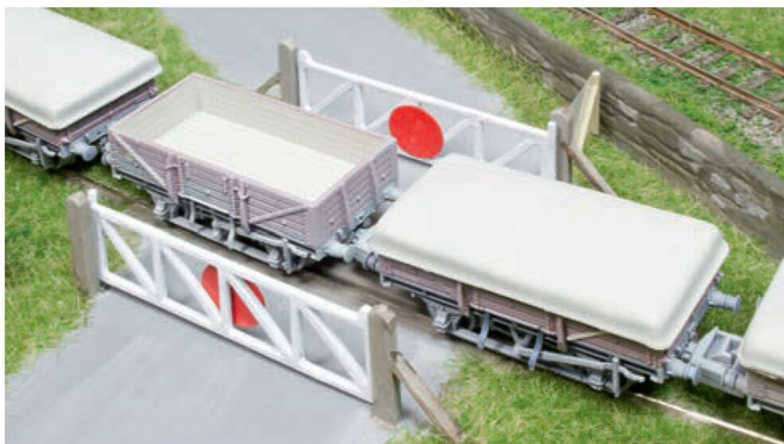
↑ The level crossing gates are worked manually using angled levers located on the underside of the baseboard.
