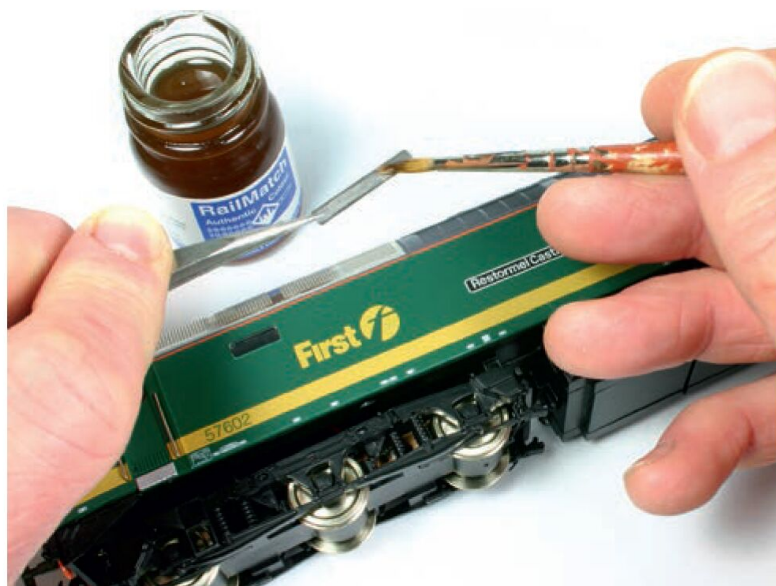
↑ Both enamel and acrylic varnish makes the best adhesive for applying nameplates, number plates and plaques.
