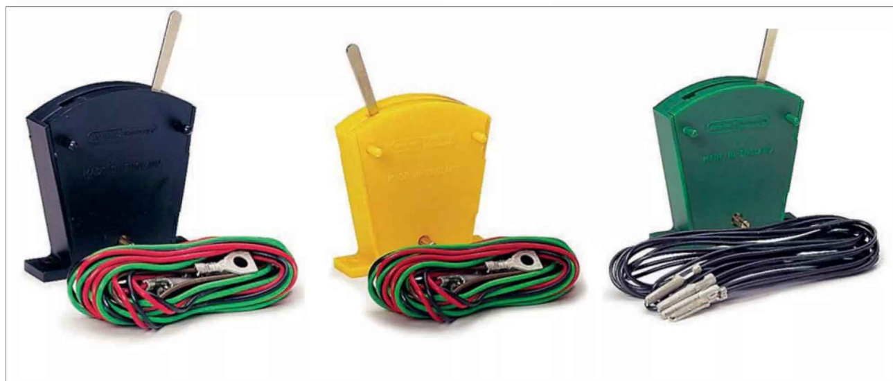
Three Hornby lever switches. Left to right: Black R044 passing contact point switch. Yellow R046 lever switch with On/On contacts – ideal for switching two aspect colour light signals etc. R047 Green lever offering On/Off switching – ideal for track feed isolating sections or controlling building lighting. Pictures © Hornby Hobbies Ltd
