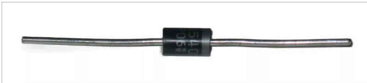
A typical diode. The silver banded end is the Cathode (negative) connection.
