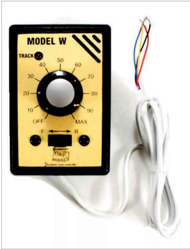
Hand-held controller. This is the Gaugemaster model W. It will be fitted with a four pin DIN plug. A mating four-way chassis socket is fitted into the panel and connects the controller to its power supply and takes the two track feed wires onto the rails.
