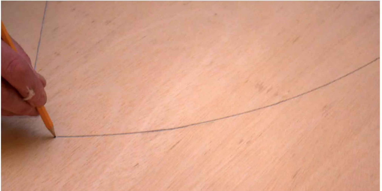
Stage 1: Where a curve is required draw the centre line of the track onto the baseboard using a pin, string and pencil. The length of string between the pin and pencil is equal to the radius of the curved track.
