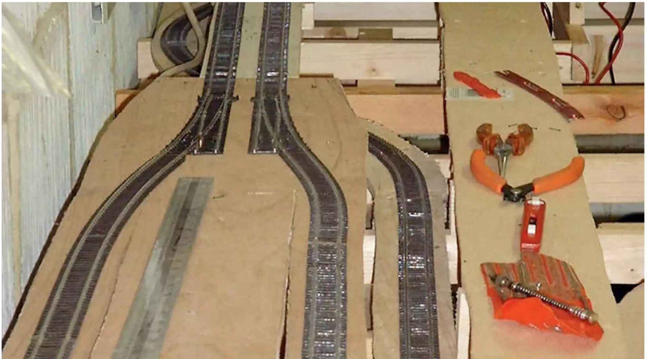
Stage 1: Track laying beginning to take place. Note the tools used – including a steel rule to give a straight edge. A Tracksetta gauge ensures the correct radius or curve is maintained when using flexible track. A track spacing gauge (by Peco), long curved nosed pliers, Xuron rail cutters, craft knife, Archimedean drill with drill bit fitted and a set of needle files will also come in handy. Where the steel rule is laying is the start of the slope leading up to the terminus station which is to be at a higher level.
