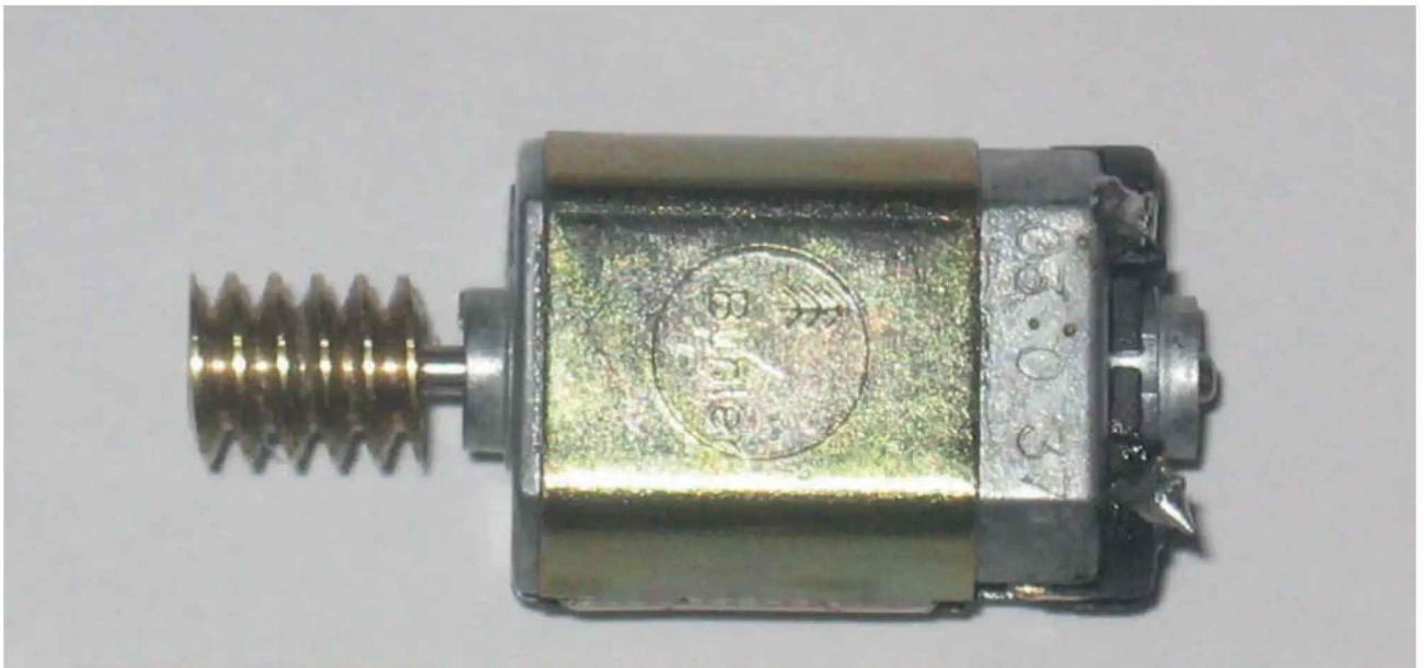
A typical 'Can' style motor which is totally unserviceable by the user.
