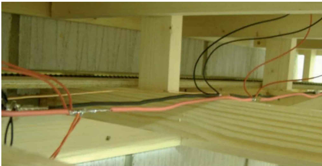
A typical DCC bus running around under the layout, wired in red and black insulated wire. Though the actual colour of the wires insulation doesn't matter, so long as they are two different colours. The droppers from the tracks above can be seen connecting onto the bus wires. In the background can be seen a bare 1.5mm 2 copper wire. This is the common return wire for everything on the layout that is not DCC operated e.g. road and station platform lighting, colour light signals.
