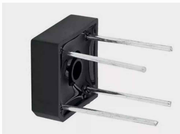
A bridge rectifier. The chamfered corner on the body of the bridge rectifier is the DC positive connection and is denoted by the engraved + symbol.
