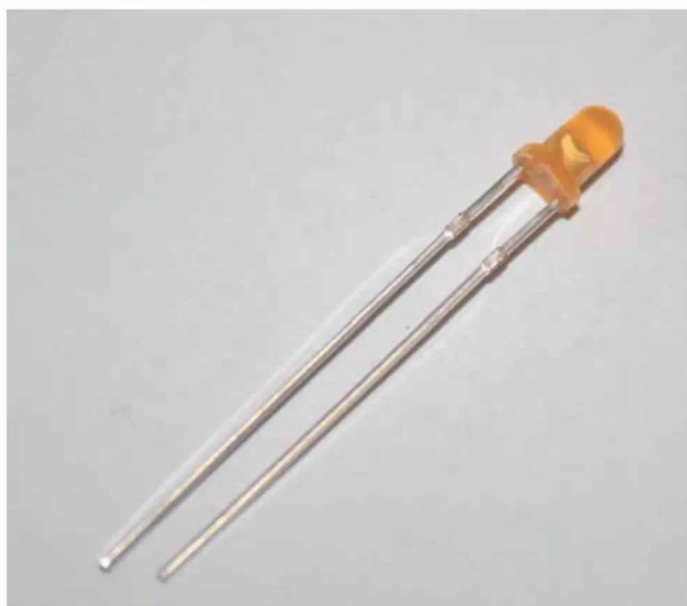
A typical yellow 3mm-diameter LED. The longer lead is the positive or anode connection.
