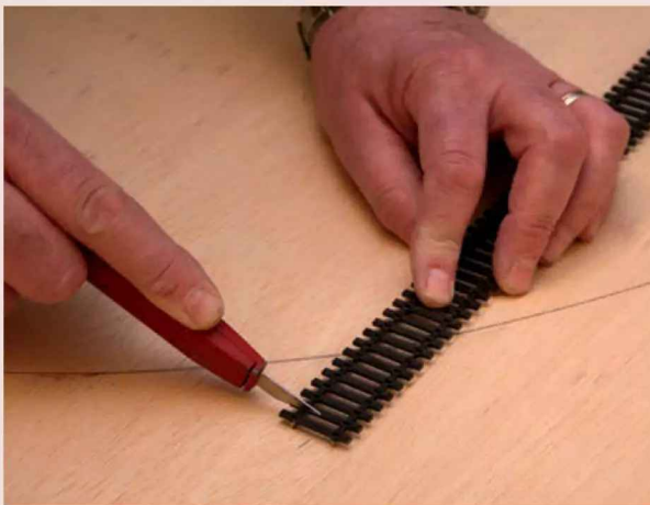
Stage 2: The last one or two sleepers are removed by cutting through the soft plastic webbing on the underside of the track. The removed sleepers are retained.
