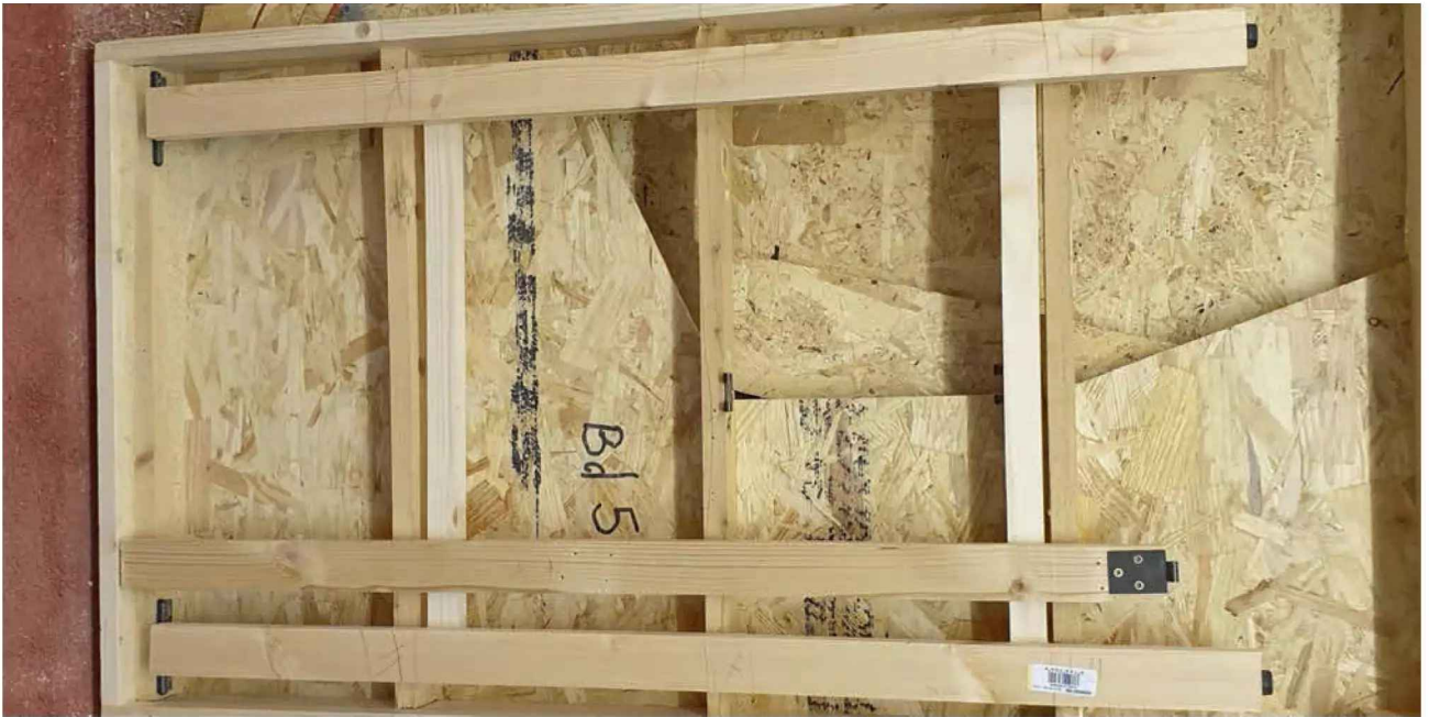
A baseboard with its support legs folded up and the central bracing stay laying in place. Note this particular board only has legs at one end as the other end locks onto and sort of 'piggybacks' to the next board.
