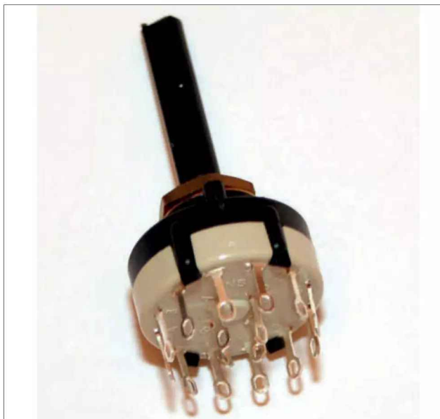
A four-pole three-way rotary switch. The four central tags (Poles) are the common connections and are connected to their respective outer tags (Ways); in this case one of three, depending on the rotary shaft's position.
