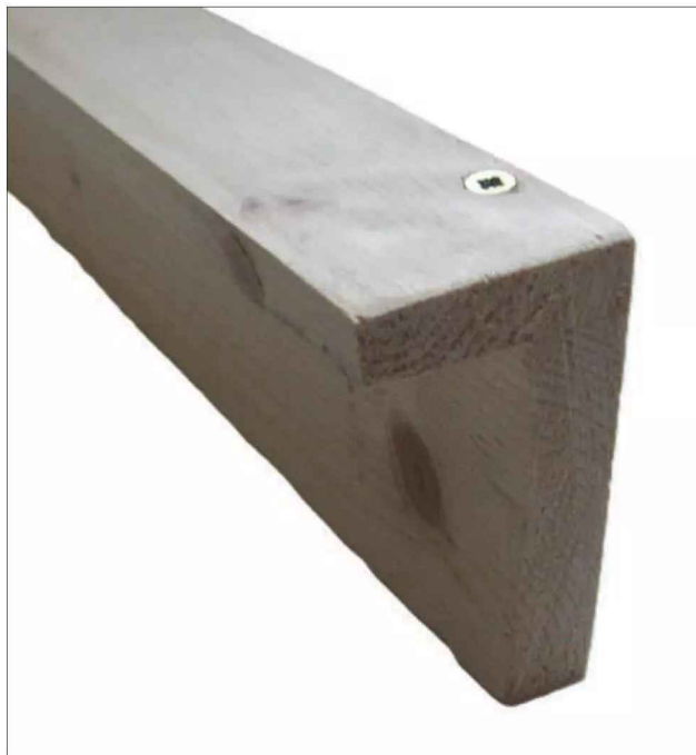
The basic L-girder shape of the timber. The timber shown is all PSE with the upright section being 69 x 18mm while the top section is 44 x 12mm woodworking PVA glued and screwed to the upright.
