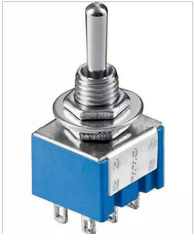
A Double Pole Double Throw Centre Off (DPDT Centre Off) switch. This switch is spring-loaded (or biased) to the central Off position, but looks similar to the DPDT switch, except the toggle lever is held centrally by the internal spring and the toggle cannot lock over permanently into one of the two On positions. This switch type, or its single pole equivalent, is ideal for operating solenoid point motors where a momentary pulse of power is only required to move the motor over. The switch offers (On)-Off-(On) selection. The bracketed items indicate that the switch cannot remain in that position.
