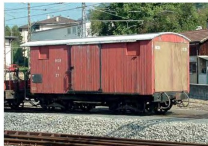
Above and below X 21 had the distinction of being the oldest extant van on the MOB, having been built by SIG in 1901. It was earmarked for transport de bourreuses (tamperers), becoming X 101 in 1965 and X 21 fourteen years later. In both 2007 and 2009 it was to be seen in Chernex works yard. Due to its historic significance it was passed to the Blonay-Chamby in 2013.
