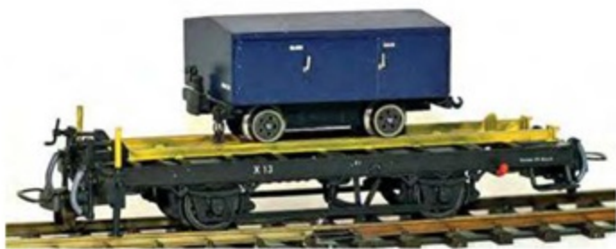
Above X 13 was a four-wheel flat used for transporting bogies, formerly Ek 607, transferred to service stock in 1973 and scrapped in 1990. Friho produced a model, supplied carrying Glion-Naye wagon Z 16.
