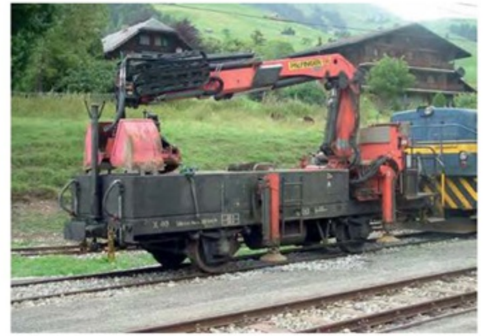
Left and right Heavy duty crane wagon X 40 can lift loads of up to 5.8 tonnes with its Palfinger crane powered by a Deutz diesel engine; four outriggers are provided for stability. In July 2009 the crane truck was seen coupled to Gm4/4 diesel locomotive No.2003.
