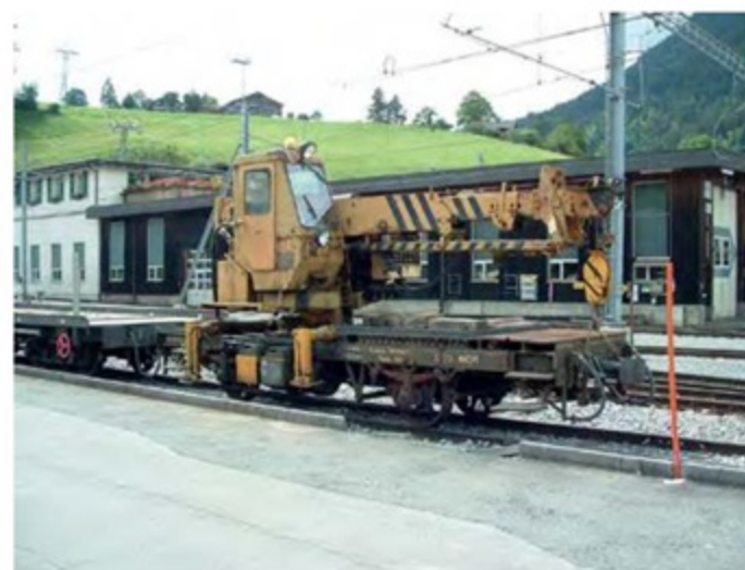
Left and right Since an Austin Western crane was mounted on the chassis of Ek 614 in 1989, the resultant X 23 has proved a reliable workhorse. Seen at Zweisimmen in September 2010.
