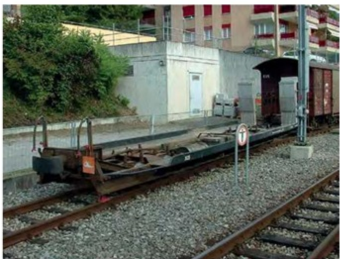
Below left and right X 25 is mounted on a pair of the original standard gauge transporter bogies which had formerly been used on cement silo wagon Uace-k 883. It was rebuilt as a low-floor bogie wagon designed with substantial ramps for roll on/roll-off loading of road vehicles. The photograph of the empty vehicle taken at Chernex in September 2007 shows that all the pipes and tanks are exposed so they would present quite a challenge to model in detail. X 25 was spotted again at both Schonried and Zweisimmen in July 2009 carrying an excavator.
