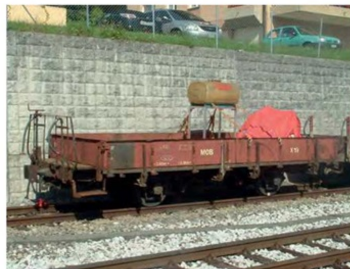
Above Low steel side open wagon X 19 was originally Kk 752. MOB describe its use as transports fraiseurs , for carrying milling equipment. It was stabled at Chernex station in July 2009. It was withdrawn in 2014. Friho listed a model in 2004.
