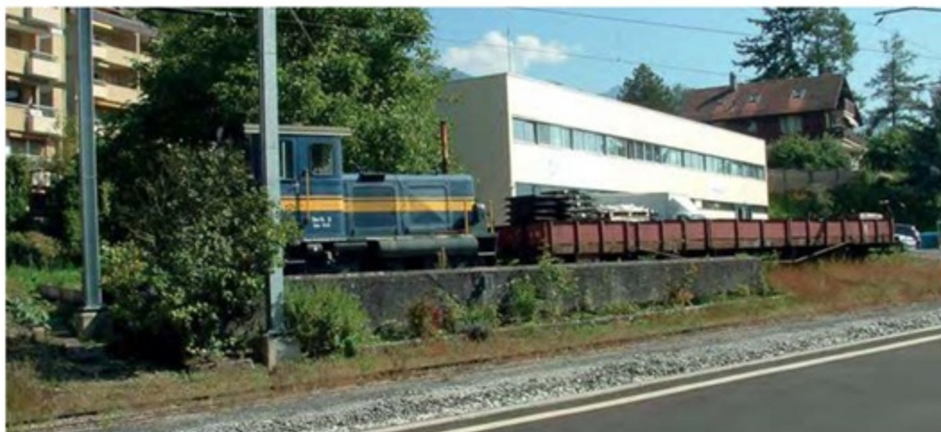
Above Built in 1914 as Rko 825, X 15 was transferred to service stock in 1976/7. Despite being suitable for long (14.5m) loads, it is listed as a flat wagon for ballast, although when seen parked at Fontanivent in September 2007 (above right) it was being used for track components. The model (right) is by Friho.
