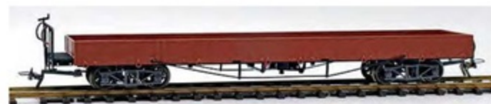
Above Built in 1914 as Rko 825, X 15 was transferred to service stock in 1976/7. Despite being suitable for long (14.5m) loads, it is listed as a flat wagon for ballast, although when seen parked at Fontanivent in September 2007 (above right) it was being used for track components. The model (right) is by Friho.
