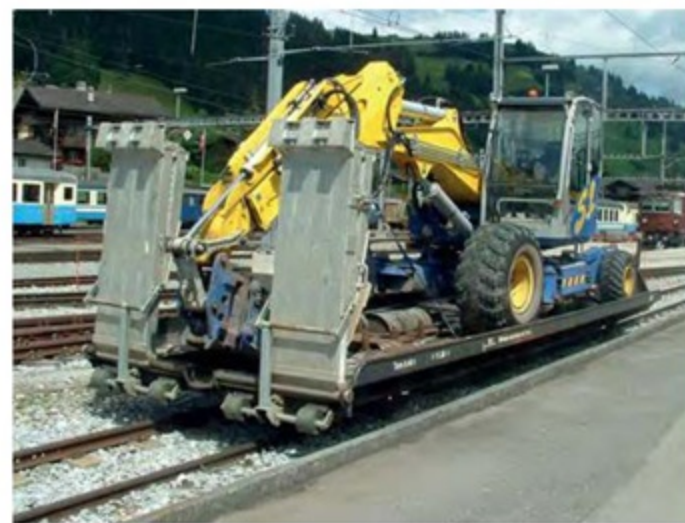
Below left and right X 25 is mounted on a pair of the original standard gauge transporter bogies which had formerly been used on cement silo wagon Uace-k 883. It was rebuilt as a low-floor bogie wagon designed with substantial ramps for roll on/roll-off loading of road vehicles. The photograph of the empty vehicle taken at Chernex in September 2007 shows that all the pipes and tanks are exposed so they would present quite a challenge to model in detail. X 25 was spotted again at both Schonried and Zweisimmen in July 2009 carrying an excavator.
