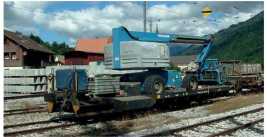
Above and right X 41 was built in 1986 using an original truck transporteur (Ua 851) for standard gauge wagons. Here at Montbovon in September 2010 it carries a road mounted access platform. It was withdrawn in 2013.
