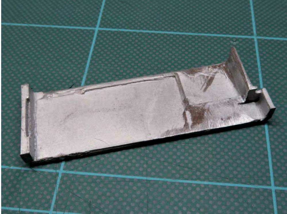
The inside locating strips need to be reduced.
