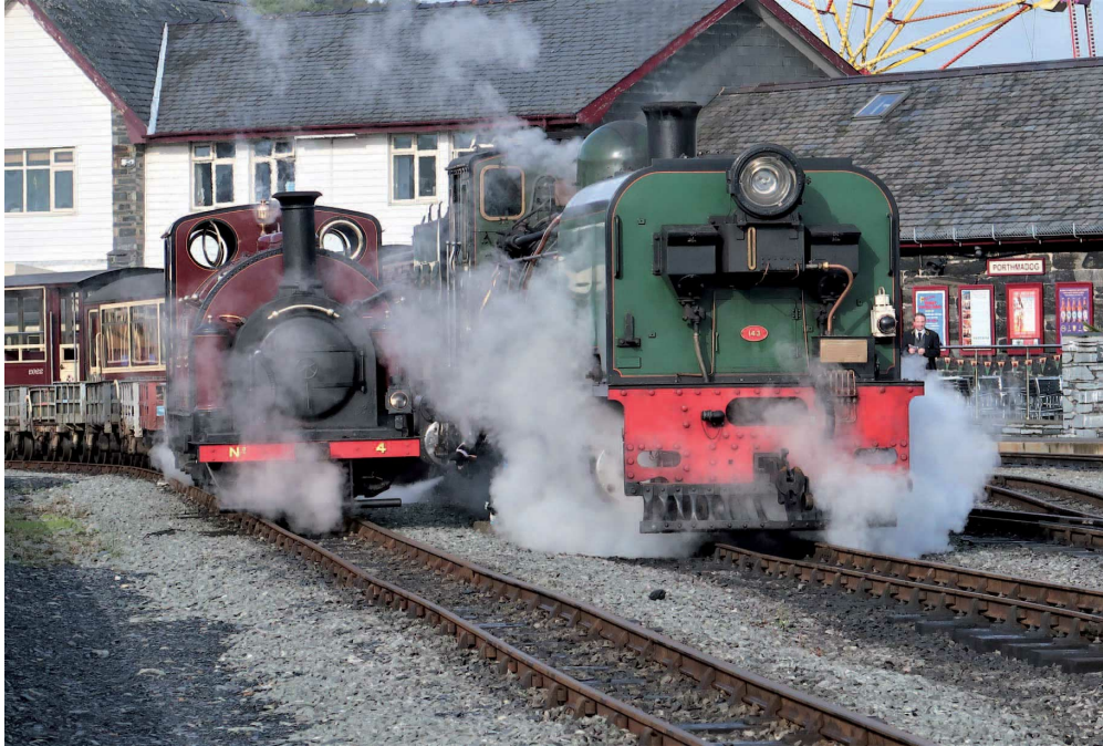
The different loading gauges are apparent here, with both locomotives running on 1ft 11½in track despite the obvious size difference.
