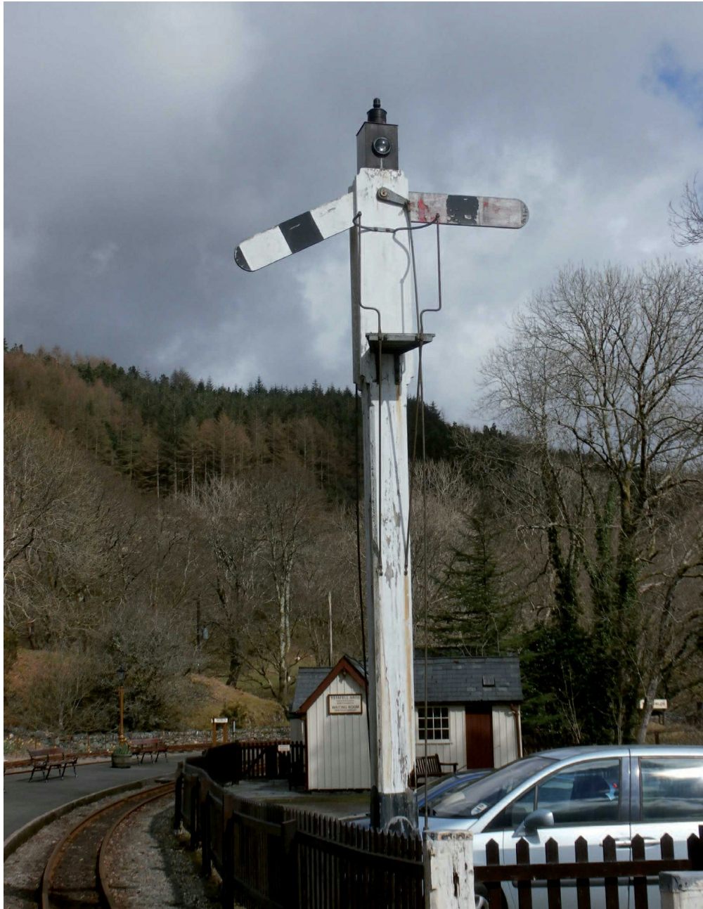
Double-arm, split-post semaphore at Tan-y-Bwlch station.
