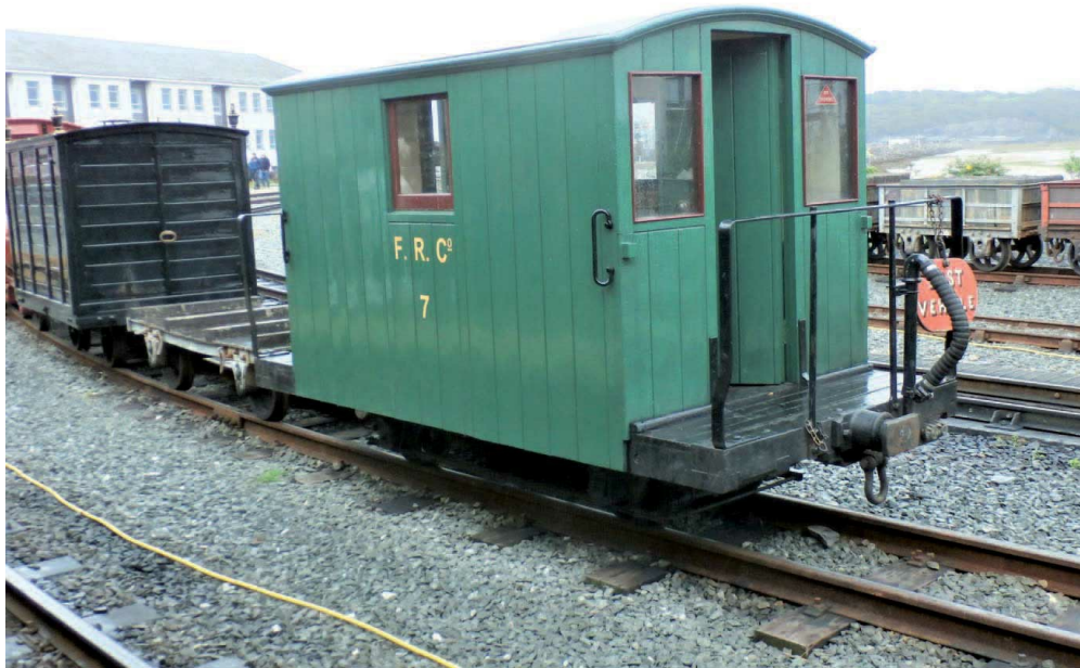
The prototype (rebuilt) FR brake van stands at Porthmadog Harbour behind a demonstration goods train.
