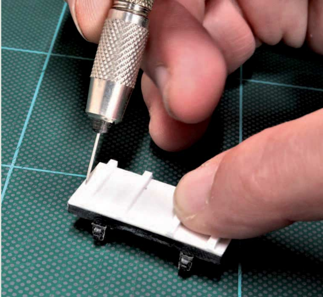
Dummy rivets can be formed using a needle in a pin chuck.
