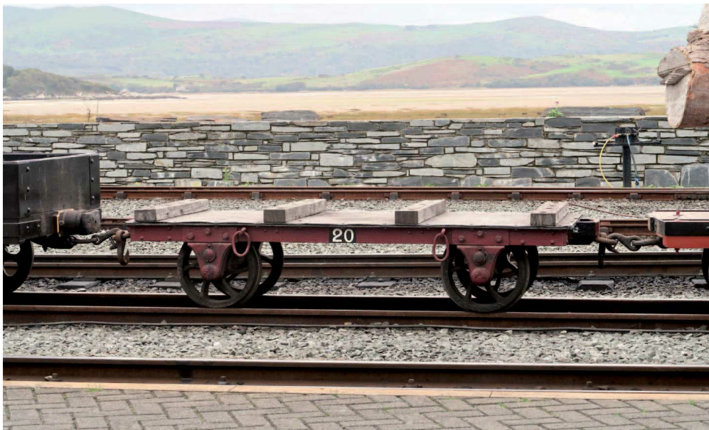
Prototype slab wagon. Note the shape of the retaining rings.
