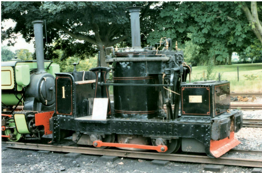
Small vertical-boilered 0-4-0 locomotives, built by De Winton, often worked the quarries. A few of these were saved and still exist on preservation lines.
