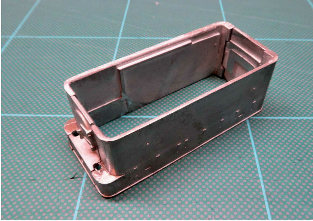
The main body parts showing the almost smooth inside surfaces to allow for the new floor and Kato chassis to be fitted.
