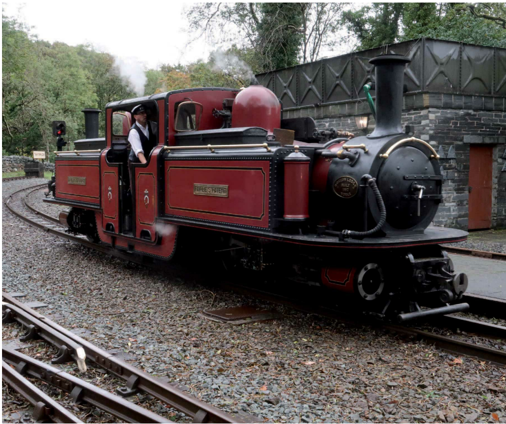
The Fairlie double engines were developed to add power without adding width and height.
