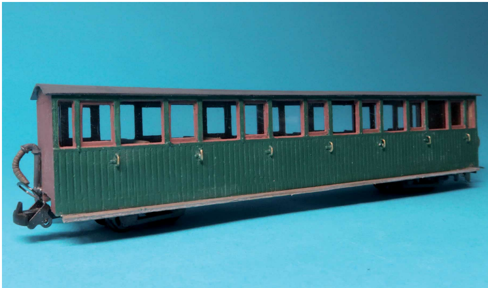
The completed coach with roof and vacuum pipes added.
