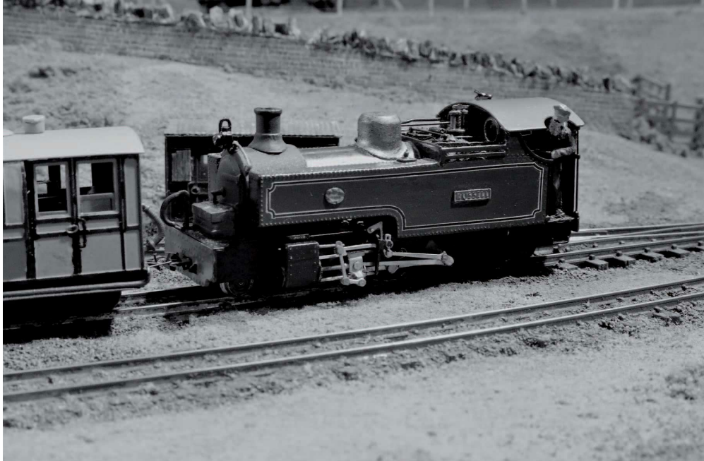
Matthew Kean's model of the WHR Russell, which was cut down in height to fit the Festiniog's tight loading gauge.
