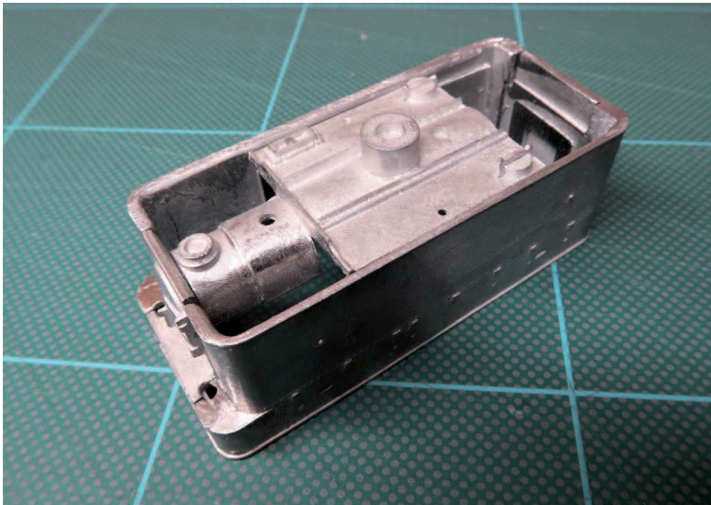
The main body parts assembled, with the tank top part being trial-fitted.
