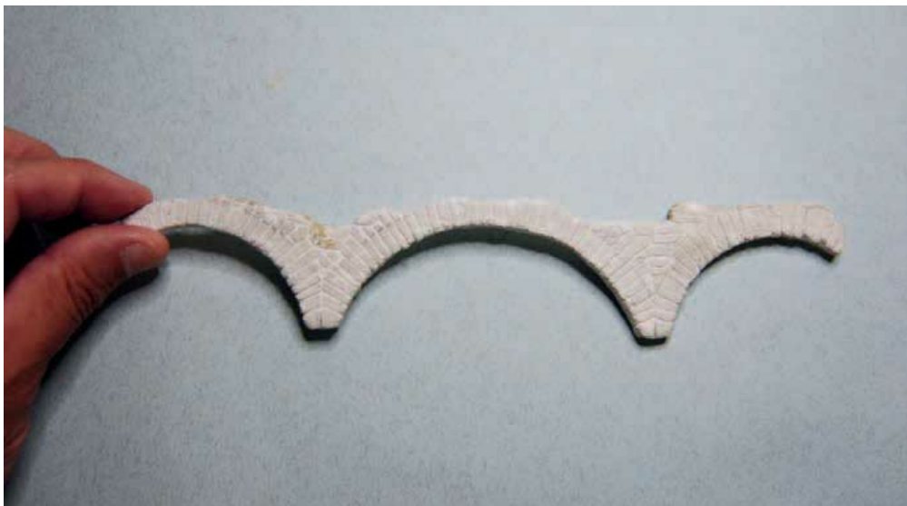
All the arch voussoirs have been scribed, along with the rubble stone infill.
