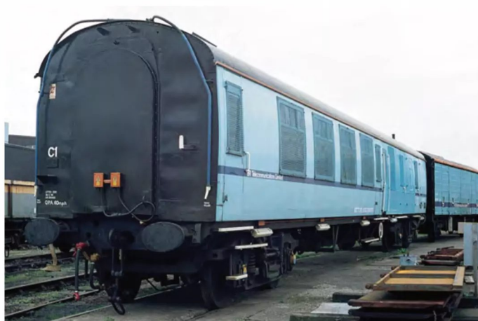
ABOVE: Most of the Mk.1 staff and generator coaches would go on to receive the Project Mercury blue livery and then transfer to the BRT fleet. However, only three appear to have seen much further use with BDC977165/66/68 being supplemented by two generator vans converted from VDAs. Now coded QPA after conversion from vacuum to air brakes, BDC977166 (ex BSK 35419) is seen at Chester wagon repair depot on April 4, 1997 in the company of ZXA generator van BDC210382. BRT adopted the ownership prefix of 'B' for its rolling stock, hence 'BDC', but this was even used on the coaches when they should have become 'BDB'. The Mk.1 is also now fitted with anti-vandal mesh screens over all the windows. David Ratcliffe
