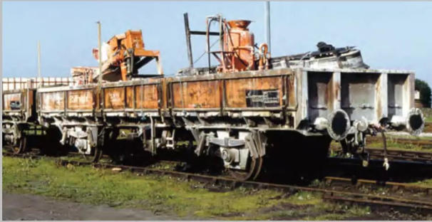
ABOVE: A filthy DC460164 was the centrepiece of what was seemingly a cement mixing train at Blackburn on May 17, 1992, the wagon still being in Railfreight red with yellow-backed Pike lettering. Of note are the wooden poles to allow rudimentary electric lights to be strung up. Accompanying it were three more Pike, DC460089/278/327, these all being in the same livery but slightly cleaner and with lighting poles also fitted. These were variously carrying un-sheeted gravel, what was likely sand and cement bags under tarpaulins and a rectangular tank, doubtless as a water supply. Trevor Mann
