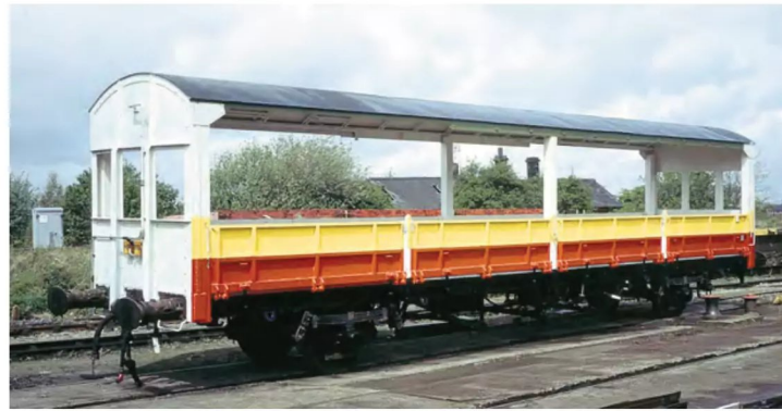
ABOVE: As their stores use petered out in favour of road movements, some of the ferry vans were converted into ZDX general material carriers. These retained their ends, albeit modified, and roof but the sides were completely replaced by four drop doors. The wagons were also fitted with integral lighting. KDB787167 is seen part way through conversion at Carlisle Currock in May 1992 with its paintwork yet to be completed and lettering applied David Ratcliffe
