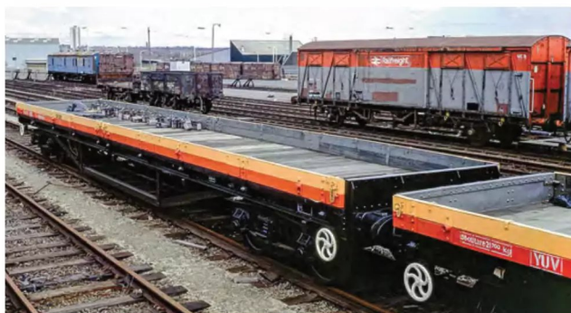
ABOVE: The former vacuum-braked Boplate wagons tended to be used in the recovery of scrap materials from worksites or S&T depots. However, when recorded at Tyneside Central Freight Depot in March 1991, YUV KDB948059 was seemingly an odd choice of wagon to be carrying numerous scrap batteries recovered from lineside equipment. David Ratcliffe
