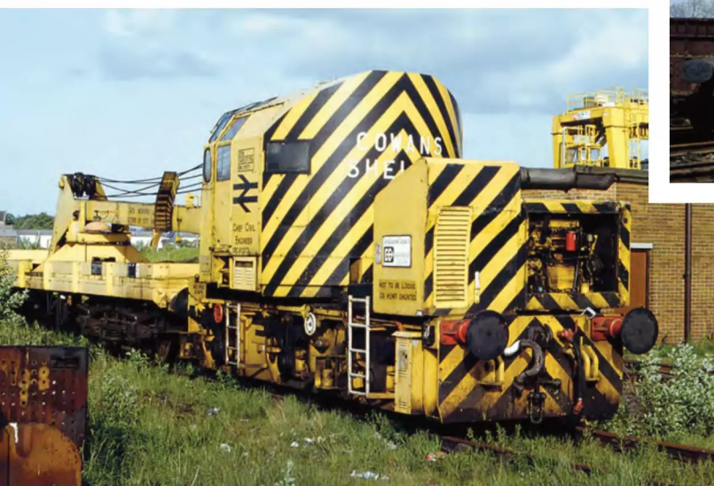
ABOVE: Another Taylor Hubbard product but this time a light duty diesel electric type, DM1764 (later DRT81264) was a unique crane. Built in 1960, it was the first experiment into using a telescopic jib as BR looked to develop a new group of cranes that could work under overhead electrification. Although innovative, it was limited to lifting just 6½ tons. Seen at Watford Junction on July 7, 1979, it had Plate wagon DE250526 as a runner and would be scrapped in 1988. Simon Bendall Collection
