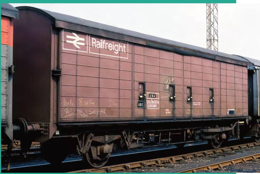
BELOW: During 1983, over 30 VCA vans that were no longer required for tinplate traffic were reassigned to the M&EE as the type's wide central door aperture suited the engineers. Still in its original Railfreight maroon scheme but now recoded ZRA, newly transferred ADC200390 was at Cardiff Tidal on June 17, 1983. Simon Bendall Collection
