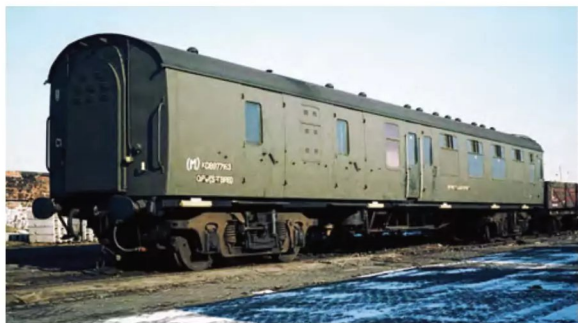
ABOVE: To power the lighting, each Project Mercury train included a staff and generator coach such as QPW KDB977163 seen at Ardwick West in February 1986. Seven converted Mk.1 coaches, KDB977162-68, were allocated to the project and finished in olive green, although by 1991 at least one of the coaches had been repainted in Satlink red and yellow. David Ratcliffe
