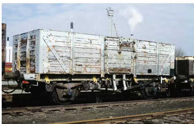
ABOVE: At least two 21-ton Ferry Highs were repainted in the Rail Stores livery, ADB715013 and ADB715027 also being recoded as ZGA following removal of their vacuum brake equipment. The latter was at Warrington Arpley in April 2000, having gained an erroneous 'M' prefix to its number. David Ratcliffe
