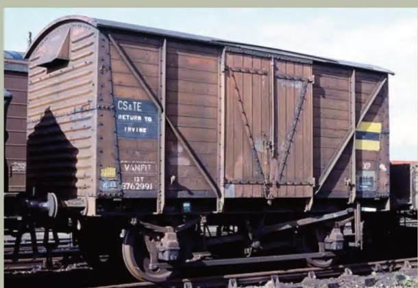
ABOVE: Another 1/208 van, KDB762991 was recorded at Motherwell on September 28, 1981, this displaying the yellow and black stripes of the Scottish S&TE. It is also lettered for return to Irvine but carries no TOPS code, it still having its Vanfit lettering despite the other branding changes.
