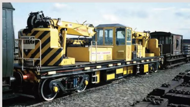
ABOVE: Built in 1977, DRP78211 was the first of the Plasser & Theurer TJC-60 relayers with 13 more following by 1980. It is seen at St Helens Shaw Street during April 1984 and still exists today in the ownership of Track Engineering Ltd, where it is available for hire. Several others remain in main line use. David Ratcliffe
