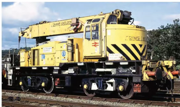
ABOVE: The Cowans Sheldon version of the telescopic jib crane is illustrated by DRC81539 at Carnforth Bottom End Sidings in March 1989. There were 14 examples delivered in 1978/79 as DRC81533-46, these seeing particular use in the north of England and Scotland whereas the Plasser type was more common in the southern half of the country. David Ratcliffe
