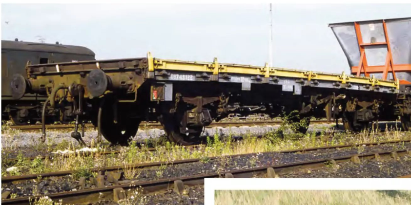
LEFT: The Carfit C required no alterations at all for their Bream role beyond cosmetic concerns. Coded ZEX due to its dual brakes, DB748122 displays the full grey and yellow look at Toton Yard on September 20, 1986. Trevor Mann
