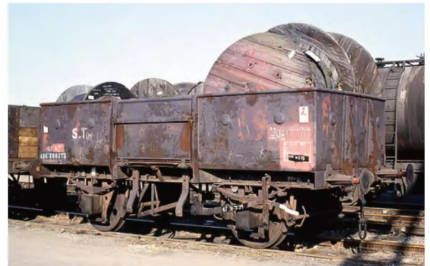
ABOVE: Much use was also made of the vacuum-braked 13-ton Highfits, be they wooden or steel bodied and BR or pre-nationalisation builds. Carrying a diverse load of cable drums, KDE296273 soaks up the sun at Cambridge on August 28, 1979. Simon Bendall Collection
