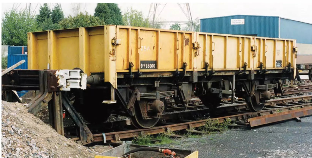
LEFT: Salmon prototype DB996699 is seen at Scunthorpe freight depot on October 9, 1995, while being loaded with sections of point and crossing rail. As these are over-length, runners are present at both ends while the new rails are notably painted white in an effort to help with heat deflection during hot weather. The livery is the original engineers' grey and yellow, although the latter is restricted to a thin stripe along the top edge. During 1998, its TOPS code would briefly become YLA before the new FZA identity was adopted. David Ratcliffe
