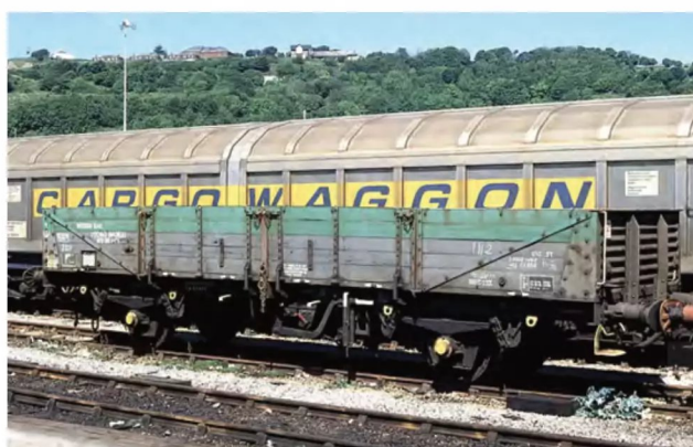
ABOVE: Until the final sailing of the cross-channel train ferry in December 1995, a handful of Ferry Tubes were used to carry spare wagon parts to and from the continent. Dual-braked ZDX 21 70 6094 053-3 had been repainted in Rail Stores livery when spotted at Dover in May 1989. Trevor Mann
