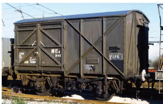
BELOW: Still in olive green livery, ZRB Palvan ADB781864 was en route from Cardiff Cathays to Carlisle Currock when recorded at Walton Old Junction, Warrington, in August 1987. The most obvious sign of the upgrading of these vintage vans was the new suspension linkages and rearranged brake equipment. Trevor Mann
