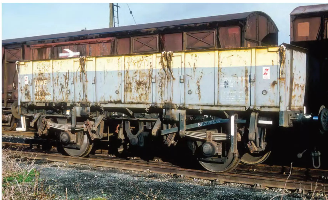
LEFT: The three Hake were built in 1981 using the frames of unfitted Grampus dating from 1956, these receiving new bodywork on top and similarly modernised air brakes and suspension below. On February 6, 1988, DB986208, then coded ZDA, was recorded at Hoo Junction, shortly before it was transferred away from the former Southern Region to work in Scotland. Paul Bartlett
