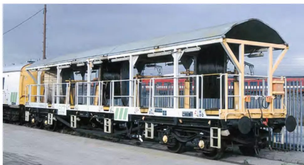
ABOVE: The YVA cable drum carriers followed their S&T sisters in having an open framework to support electric lighting. Unlike these earlier examples, the BRT batch also gained a roof as demonstrated by BDC950210 at Leeds Whitehall Road in November 1996, this carrying drums of new cables. David Ratcliffe
