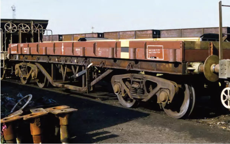
RIGHT: Another modified Bogie Bolster E, KDB924203 had been fitted with a HAP hydraulic jib for use by the S&TE to unload concrete troughing and presumably also pick up used and damaged troughs. Seen at Brent Yard, Cricklewood, on October 13, 1979, it was still in use in the early 1990s albeit repainted. The lettering is somewhat confused as, although correctly prefixed KDB, the wagon was still carrying its BEV TOPS code from its revenue earning days. Trevor Mann
