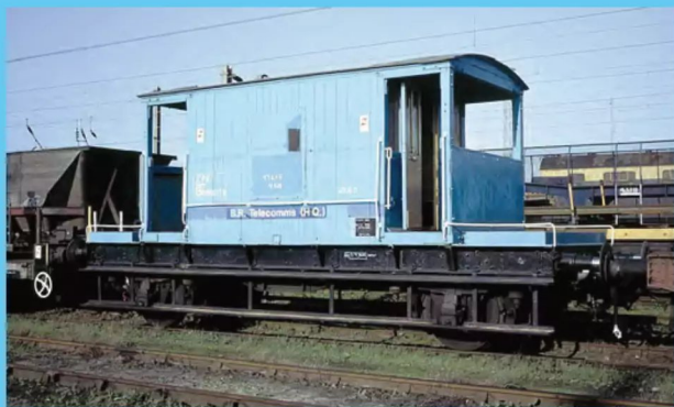
ABOVE: Like a number of other brake vans assigned to the S&T Engineers, KDB950718 had been modified into a staff van for use by Project Mercury personnel when heading to and at worksites. Seen at Warrington Arpley in May 1992 and now coded ZPR, this also included a more elaborate livery with the addition of a dark blue band. By this date, BR Telecomms (HQ) branding had also been applied. David Ratcliffe
