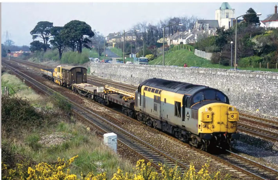
LEFT: Railfreight Red Stripe-liveried 47339 is seen approaching Stockport on October 15, 1988, with one of the distinctly unusual Thomas Smith 18-ton diesel hydraulic cranes in tow. Built in 1970, DRS81502 was another variant on the telescopic jib design but had a full width operator's cabin at the opposite end to the jib. Only two were built and they were not a success, being found to be unstable both in use and transit. On this occasion, the working also featured a Salmon with recovered track, another of the LNER ballast brakes as a mess van and a BR standard brake van. The runner behind the crane is also a rarity, this being DB710253, one of two experimental Conflat D prototypes now transferred to departmental use as a ZSV.
