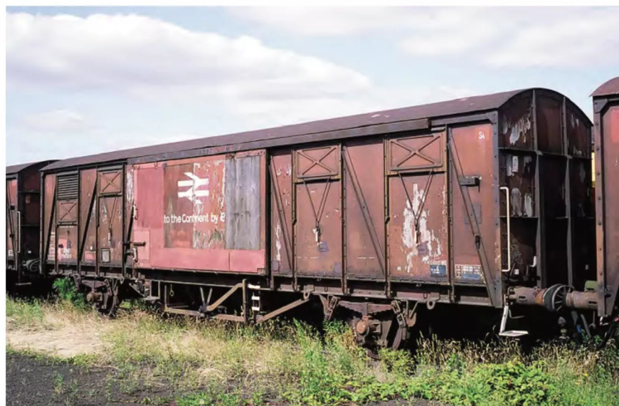
ABOVE: Much use was also made of the vacuum-braked 13-ton Highfits, be they wooden or steel bodied and BR or pre-nationalisation builds. Carrying a diverse load of cable drums, KDE296273 soaks up the sun at Cambridge on August 28, 1979. Simon Bendall Collection
