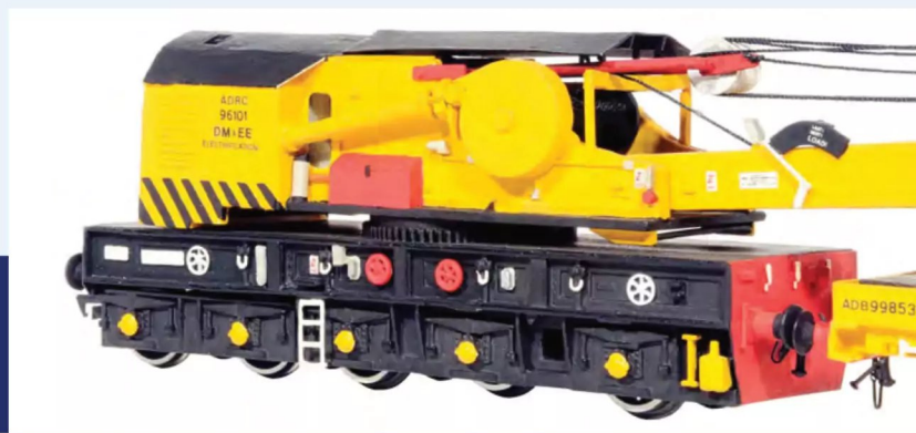
RIGHT: The main section of the crane incorporates parts of the Hornby model such as the main frame but a lot of it is made from scratch. This includes the substantial side frames, which feature a three-axle rigid section and two-axle bogie at the rear as per the real crane.
