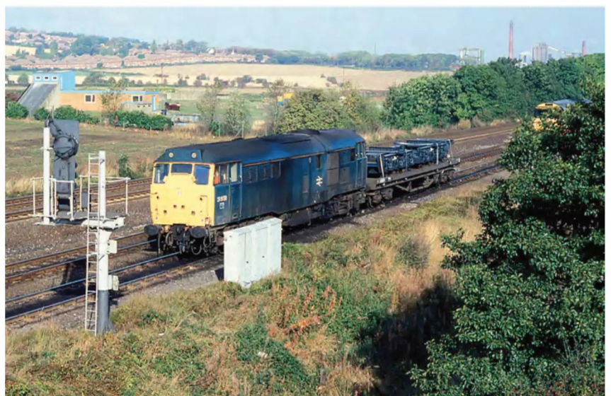
ABOVE: Immingham's 31558 awaits the road at Tupton, south of Chesterfield, and the passing of the Class 58 that is emerging from behind the bushes in the summer of 1990. In tow is an air-braked Bogie Bolster D carrying two of the Pollen wagons on modified wooden blocks and strapped to the deck. This may well be one of the modified Brill prior to being recoded as YXA and receiving a repaint. Simon Bendall Collection
