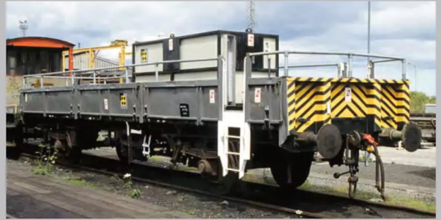
ABOVE: SPA 460717 stands at Blyth Cambois TMD in July 1993 following conversion to a weedkilling wagon for use on the freight-only Blyth & Tyne route. With the conversion having been funded by Trainload Coal, it was still officially a revenue earning wagon even if its purpose was not. At this stage, its number panel had yet to be applied to the smart sub-sector colours. Mark Saunders
