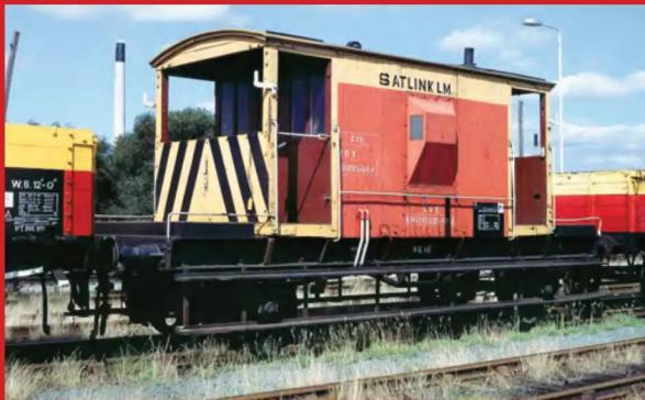
ABOVE: Repainted in Satlink colours but otherwise unaltered, 20-ton ferry van KDB787285 was at Radyr during September 1991 and recoded as a ZRX. Like the former VDA vans, these were used to move stores to and from S&T depots, providing both weather protection and security. David Ratcliffe
