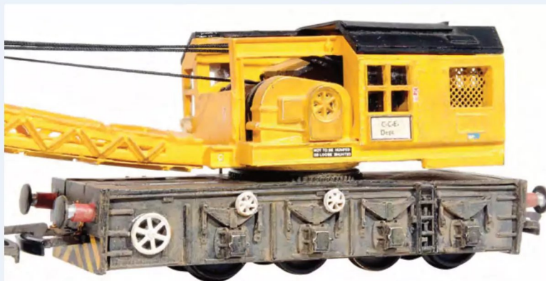
A close-up of the crane showing the scratchbuilt sides to the chassis and lower bufferbeams, these being grafted to the remainder of the plastic kit. The crane body pushes into place on the chassis.
