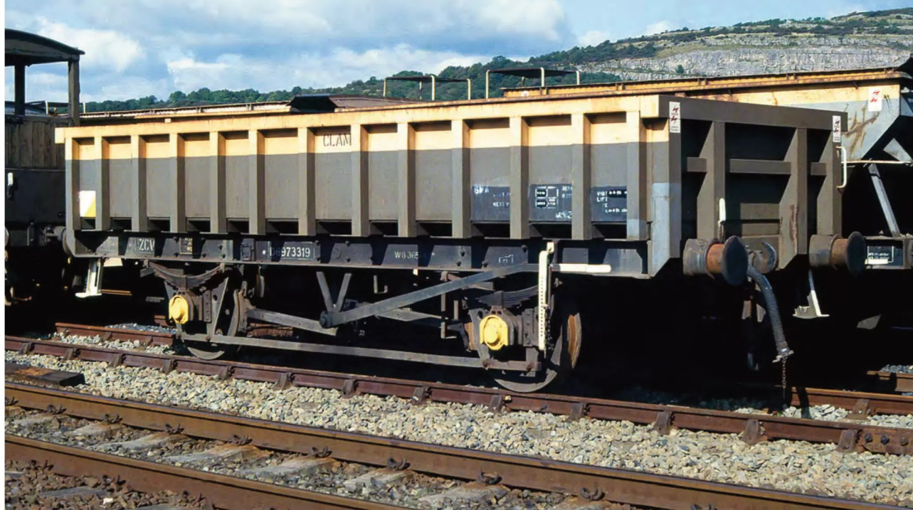
In contrast, RFS-converted DB973319 has its numbering details applied directly to the solebar, this having employed the underframe of HTV B427182. Seen at Carnforth on September 26, 1993, the re-positioned vacuum cylinder is hidden in the area of shadow between the left-hand wheel and the central 'V' hanger. Trevor Mann
