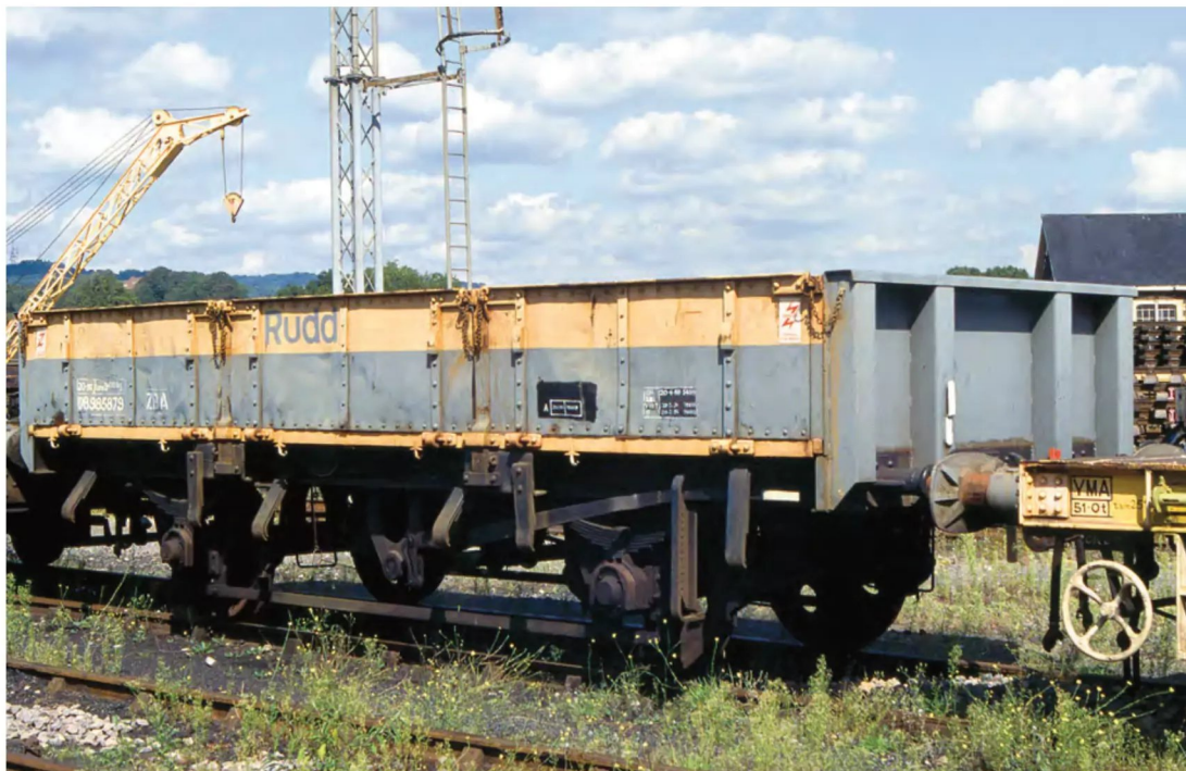
LEFT: The most common version of the Grampus to Rudd conversion just saw the ends rebuilt and air brakes fitted. On August 25, 1991, DB985978 was found residing in Radyr Yard. The thin yellow stripe along the solebar was a common feature of the conversions and may have been a form of visual identification. Trevor Mann
