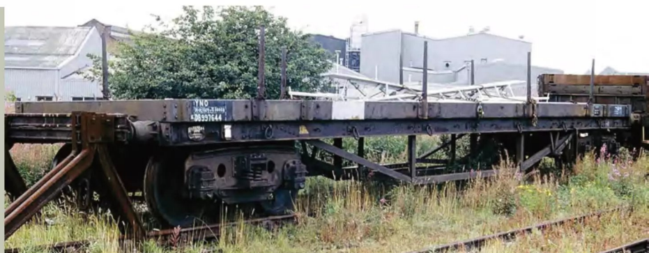
RIGHT: Another copy of a revenue-earning design were the 69 Bogie Bolster C wagons built specially for the S&TE fleet between 1952 and 1954 as part of diagram 1/471. Coded Prawn, they took the numbers DB997600-47 and DB997649-69, allocations from new being to the London Midland, Eastern and Western regions. YNO KDB997644 was loaded with a set of crossing barriers when seen at Bamber Bridge permanent way depot on August 14, 1981. One final design built for the S&TE in 1954 were two diagram 1/490 Boplates, these being coded Whelk and numbered DB997400/01. Sent new to Scotland, photographs are exceptionally rare despite the duo lasting until 1981! Trevor Mann
