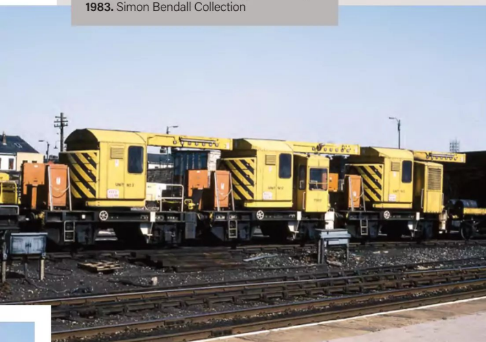
ABOVE: The Smiths-built track relayers undoubtedly had a presence with their sturdy underframes and sizeable counterweights on the back of the cranes. These were also the first of the self-propelled track relayers, DRS78203 dating from 1965. Seen at Beighton on June 23, 1985, it was scrapped in 1999 after passing to Balfour Beatty ownership. Trevor Mann
