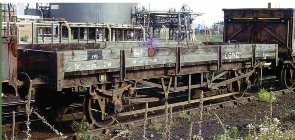
LEFT: During 1955, Wolverton built six 12-ton open wagons to diagram 1/619 for the S&TE which had wooden dropsides and fixed steel ends. No codename was allocated to DB997300-05 but all were assigned to the Scottish Region where they were used as miscellaneous material and spoil carriers. ZDO KDB997302 is seen at Rutherglen permanent way depot on August 18, 1981. Trevor Mann
