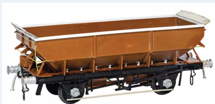
ABOVE: With the model ready for painting, the Tope shows off the alterations and enhancements made to the Parkside HTV kit. The white 'C' sections representing the floor support ends can be seen along the hopper side as can the new top capping. On the end, the way the two handrails meet is also shown.
