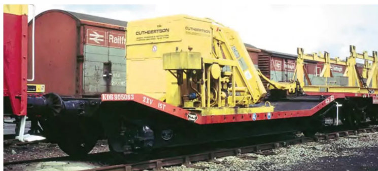
ABOVE: Carrying the same Cuthbertson contractors lettering, KDB905083 was also to be found at Carlisle Currock in May 1992. This had begun life as a 15-ton Lowmac WV to diagram 2/248 before being fitted with an Atlas hydraulic arm and diesel engine. It is believed this was used as a trenching unit with what appears to be a manual roller also chained to the deck. To the right is a Conflat A that has been converted into a cable drum carrier with the addition of a substantial support framework. David Ratcliffe
