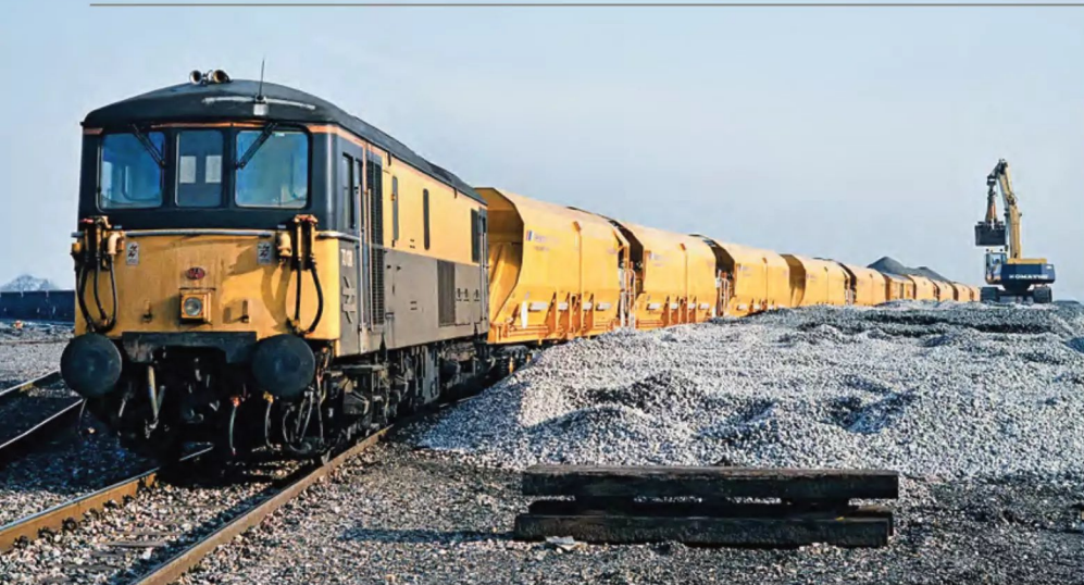
LEFT: Network SouthEast's Skako auto-ballasting train is seen at Hoo Junction on February 1, 1993, with 73138 on the front during a demonstration of the set's capabilities following delivery. The ten YDA Octopus hoppers, numbered DR92213-22, were built on the frames of Clyde Cement presflos, while the generator van DC210306 was extensively altered from a VDA and can be seen in the middle of the formation. The train was highly innovative for its time and allowed for remote-controlled discharge of new ballast and also precision laying around conductor rails, something that was difficult to achieve using manually-controlled hopper doors. Today, the Skako is owned by DB Cargo and based at Carlisle Yard.
