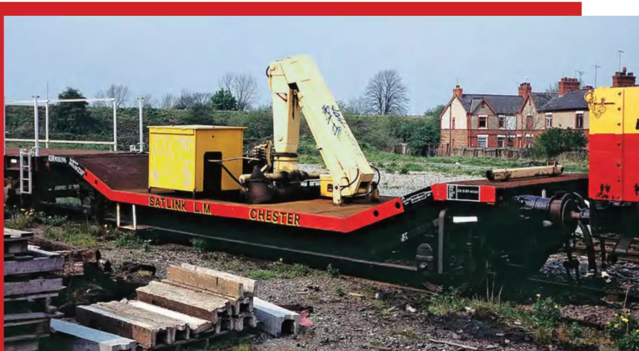
ABOVE: Former Flatrol KDB900414 was the epitome of a specialist S&T wagon, having been converted to carry two cement mixers. When first modified some years prior to its Satlink repaint, it worked with four Plate wagons, two being marshalled on either side. Those nearest to the Flatrol formed a continuation of the sloping access ramps with safety handrails while the outer pair were used as access wagons and also carried supplies. When seen at Radyr Yard on October 13, 1991, these support wagons had been dispensed with. However, still accompanying the YXP was former GWR milk tank KDW2952, this also carrying Satlink livery as a water supply. Hywel Thomas
