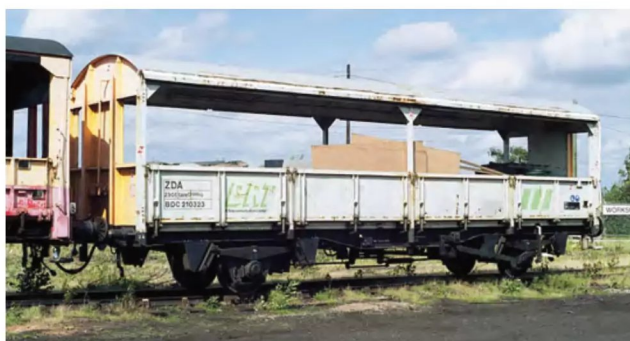
ABOVE: Converted from a VDA van at Doncaster Works during 1994, ZDA BDC210323 was recorded at Ditton in August 1998 when carrying waste sheets of plywood and miscellaneous packaging material. David Ratcliffe
