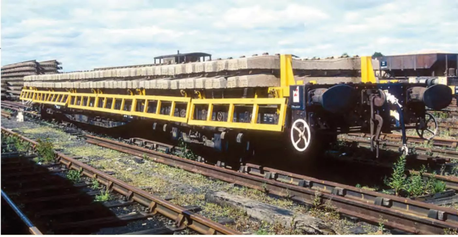
RIGHT: Bearing some similarities to the Chub, two ferry-fitted Carfit C flat wagons were rebuilt at New Cross Gate in late 1982 with three-plank sides and ends. The sides incorporated a centrally-positioned and wide drop door and was seemingly an attempt to repurpose the useful dual-braked underframes. Never given a fish name, DB748147 is seen at Woking pre-assembly depot on January 8, 1990, carrying a TOPS code of ZEX and loaded with assorted rubbish. Its sister wagon, DB748126, is off to the right and was more appropriately lettered as a ZXX. Roger Silsbury
