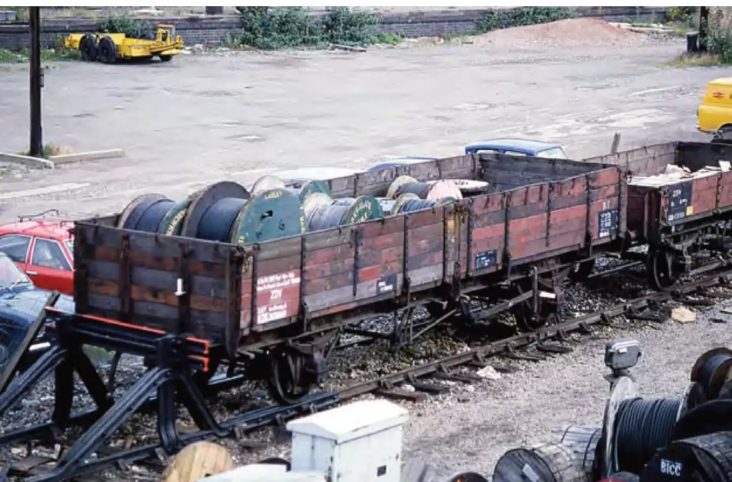
ABOVE: The LNER-designed tube wagons were much liked by the S&TE due to their length and pair of drop doors which, although heavy, gave unrestricted access for loading. In contrast, the LMS design, which had been preferred by BR, was not favoured as they only had a small central door. Much used for carrying cable troughing, they could also move cable drums as shown by KDE301569 at Newport S&T sidings on July 13, 1980. The Medfit alongside, which is Civil Engineers allocated, is loaded with an assortment of cardboard boxes, including a particularly large one and squashed empties. Simon Bendall Collection
