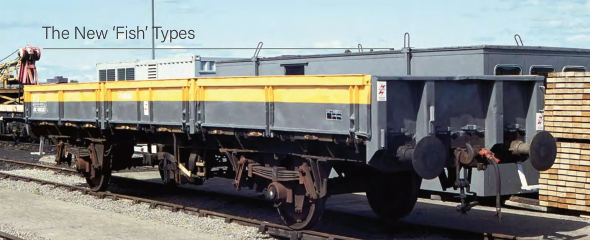
LEFT: The Seahare fleet had become quite significant in the final years of BR with considerable inroads made into the number of ZAA Pike. The steel strips along the top of the sealed doors can be seen on DC460387 at Tees Yard on May 4, 1993. Trevor Mann
