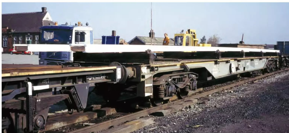
LEFT: Salmon prototype DB996699 is seen at Scunthorpe freight depot on October 9, 1995, while being loaded with sections of point and crossing rail. As these are over-length, runners are present at both ends while the new rails are notably painted white in an effort to help with heat deflection during hot weather. The livery is the original engineers' grey and yellow, although the latter is restricted to a thin stripe along the top edge. During 1998, its TOPS code would briefly become YLA before the new FZA identity was adopted. David Ratcliffe
