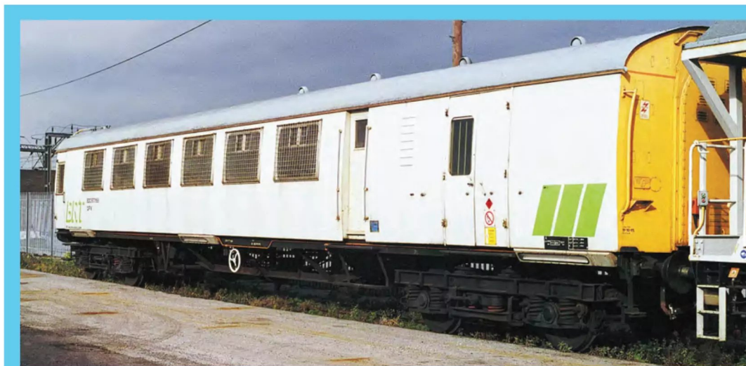
ABOVE: The YVA cable drum carriers followed their S&T sisters in having an open framework to support electric lighting. Unlike these earlier examples, the BRT batch also gained a roof as demonstrated by BDC950210 at Leeds Whitehall Road in November 1996, this carrying drums of new cables. David Ratcliffe
