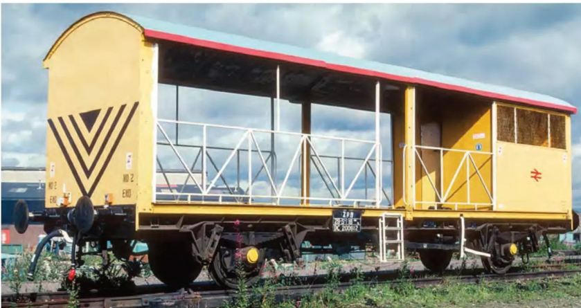
LEFT: The summer of 1991 saw two air-braked vans converted into generator wagons at Polmadie for use with Sealion and Seacow ballast hoppers modified with electric lighting. These lost their sides with a compartment provided at one end to house the generator set and its fuel tank. Also fitted with a through vacuum-pipe, ex-VBA DC200612 and former VDA DC200875 were recoded as ZXB although, when the former was photographed at Mossend on August 13, 1991, it was incorrectly lettered ZRB. Neither appears to have seen much, if any, use in their intended role and were withdrawn by the mid-1990s. Paul Bartlett
