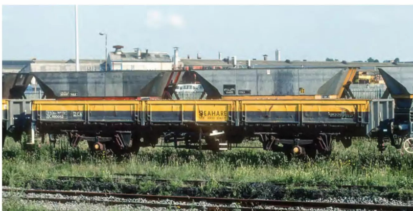
ABOVE: The initial Seahare conversions were very obviously marked up as to the status of their doors, DC460082 displaying a large version of the name at Washwood Heath on July 6, 1991, along with 'Side doors sealed' underneath. This style of branding could still be seen for years afterwards as the wagons were typically not repainted again, the branding just getting lost under rust. Paul Bartlett
