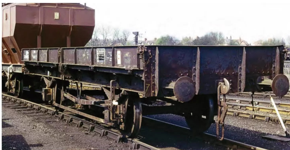
RIGHT: The two-plank 14-ton Whiting were a GWR design for S&T use that was perpetuated by British Railways to diagram 1/622. Built in three groups between 1952 and 1957, construction of the 50 wagons was split between Swindon and Wolverton with the numbers being DB997700-46 and DB995250-52, this trio being the last built. Normally found on the Western Region, ZVO DB997728 had migrated to Broughton Lane, Sheffield, by October 1983 to await scrapping. The faded lettering includes the Ew allocation and 'Empty to Reading WR' lettering. Trevor Mann
