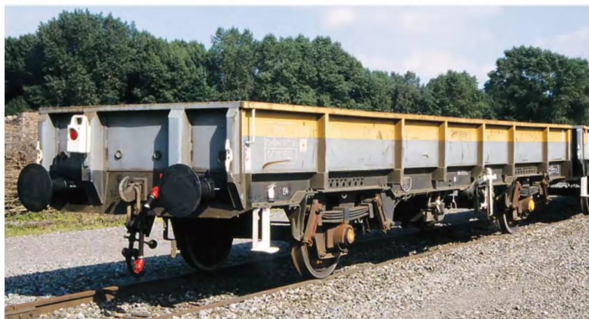
ABOVE: The six rib body preferred by RFS Engineering is illustrated by DC110522 at Cockshute Sidings, Stoke, on August 1, 1998, it being in EWS ownership by this date. The end fittings clearly show that this was the original OBA end cut down and modified. Trevor Mann
