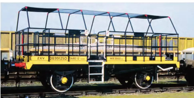
ABOVE: Another conversion that proved of little value was that of ZCV Crab DB991250 into a ZCV propelling control vehicle. Completed at Ashford plant depot in the summer of 1994, this was intended as a riding vehicle for the shunter whilst controlling propelling movements by radio instead of walking alongside the moving train. Built for use within engineering possessions, the wagon was also equipped with a brake valve for use in an emergency. With most stock on the Southern being air-braked by this date, it was of limited use; a second conversion involving a more appropriate Rudd never coming to fruition. Seemingly deemed operationally inconvenient, it languished at Hoo Junction for several years, where it is seen on April 9, 1996. Trevor Mann
