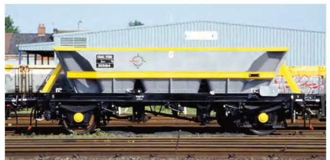
ABOVE: Outshopped from Burton wagon works at the beginning of privatisation were three HAA hoppers converted into a new type of ballast wagon dubbed Coalfish. Funded by Trainload Freight West, later to become Transrail, the work involved cutting down the hopper body in a similar manner to the Tope. Seemingly deemed an immediate failure, 353163, 353220 and 355164 were never trialled nor given a new TOPS code. The last of the trio is seen at Burton WRD on May 28, 1994. Phil Eames
