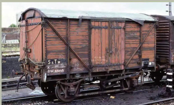
ABOVE: Also at Duddeston on the same day was KDW105669, this being a particularly distressed GWR Mogo with its end door restrained by rope and also in need of a new roof canvas. Built to carry motor cars, several found a role in S&T use, this one being lettered to return to Crewe.
