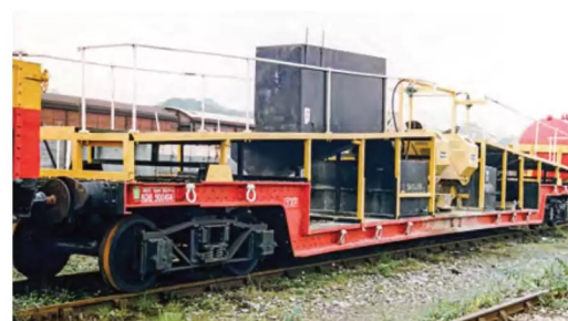
ABOVE: Former Flatrol KDB900414 was the epitome of a specialist S&T wagon, having been converted to carry two cement mixers. When first modified some years prior to its Satlink repaint, it worked with four Plate wagons, two being marshalled on either side. Those nearest to the Flatrol formed a continuation of the sloping access ramps with safety handrails while the outer pair were used as access wagons and also carried supplies. When seen at Radyr Yard on October 13, 1991, these support wagons had been dispensed with. However, still accompanying the YXP was former GWR milk tank KDW2952, this also carrying Satlink livery as a water supply. Hywel Thomas
