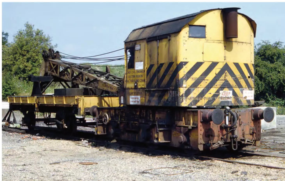
ABOVE: Another Grafton product but this time from 1954, DRG80118 was carrying its CEPS number at Hitchin permanent way depot on August 26, 1980. An Eastern crane throughout its life, the chimney for the boiler is in its inverted travel position. It was cut on Tyneside four years later. Trevor Mann
