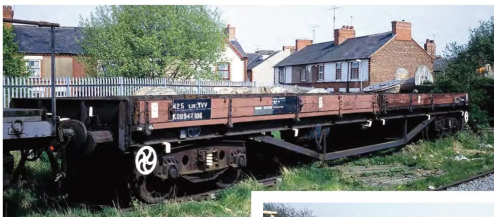
ABOVE: The S&TE also used a number of ex-revenue Boplates to convey lengthy items. Vacuum-braked YVV KDB948106 is seen in the S&T sidings at Chester on May 2, 1994, and is lettered 'Return to 59221 Leicester', the number being the TOPS location code. David Ratcliffe
