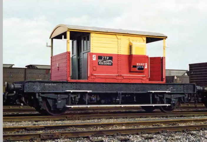
ABOVE & BELOW: In much the same way, Southern-design brake vans were also retained for personnel transport. On former Southern metals, the two-axle Pillbox design was quite common as typified by ZTP KDS56400 at Hoo Junction on February 12, 1995. Over two years later, YTW Queen Mary KDS56305 is seen at Warrington Arpley during May 1997. Although now in EWS ownership, it had performed a similar role earlier in the decade. Ian Cuthbertson/David Ratcliffe
