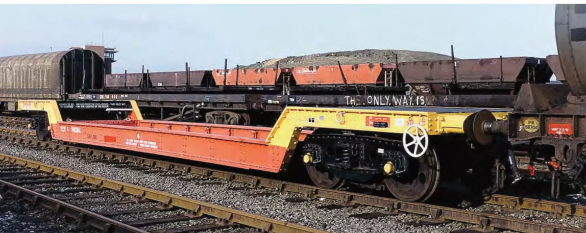
ABOVE & RIGHT: The Weltrols were a useful addition to the S&T fleet, duties including carrying scrap material, such as signals, away from worksites while they could also be used to move portable buildings. When seen at Tees Yard in February 1992, dual-piped KDB900935 was sporting full Satlink livery while vacuum-piped sister KDB900937 was only in all-over signal red at Radyr in August 1991. David Ratcliffe
