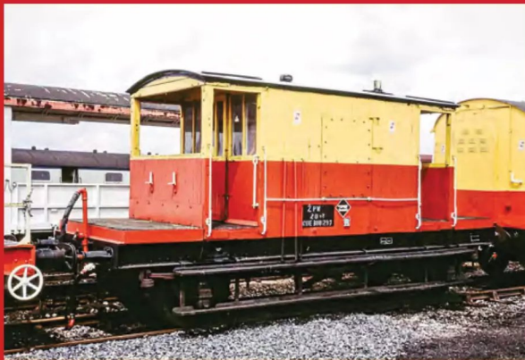
BOTH ABOVE: The brake vans owned by the S&T Engineers were not used in their traditional role by this time, instead serving as personnel carriers. When seen at Ellesmere Port in July 1992, ZTR KDB954164 had received no obvious modifications for this role but its positioning within the middle of the rake of wagons confirms its new purpose. Veteran LNER brake van KDE300297 was more obviously altered at Carlisle Currock in September 1995, having seen its duckets removed and plated over. Also recoded as ZPW, it still retained tall vacuum pipes. David Ratcliffe
