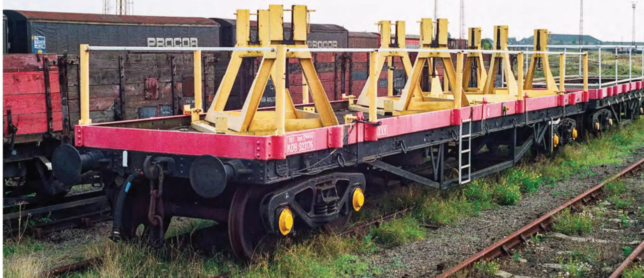
ABOVE: Apart from the YVA cable drum carrier conversions of BDA bolster wagons, various vacuum-braked flat wagons were also modified for the same purpose. Typical of the breed is former Bogie Bolster C KDB923176, the YVV being recorded at Whitemoor Yard in September 1993. Also visible is YRW KDB923962, which was originally a Bogie Bolster E. This has been fitted all round with safety handrails for use as a mobile work platform, for example it could be positioned under signal gantries to improve access rather than staff having to work from ground level. David Ratcliffe
