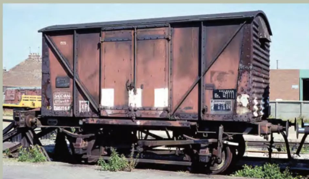
ABOVE: In contrast, you would be hard pressed to tell that shock van KDB853768 was even in S&T use if it were not for the 'KD' prefix added in front of the wagon number. Built to diagram 1/218, all the other markings were as per revenue use when seen at King's Lynn on August 28, 1979.
