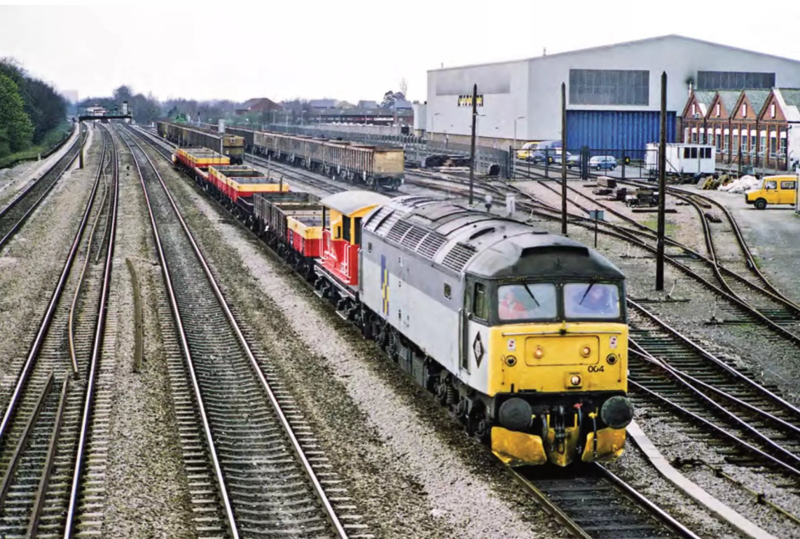
ABOVE: The former vacuum-braked Boplate wagons tended to be used in the recovery of scrap materials from worksites or S&T depots. However, when recorded at Tyneside Central Freight Depot in March 1991, YUV KDB948059 was seemingly an odd choice of wagon to be carrying numerous scrap batteries recovered from lineside equipment. David Ratcliffe
