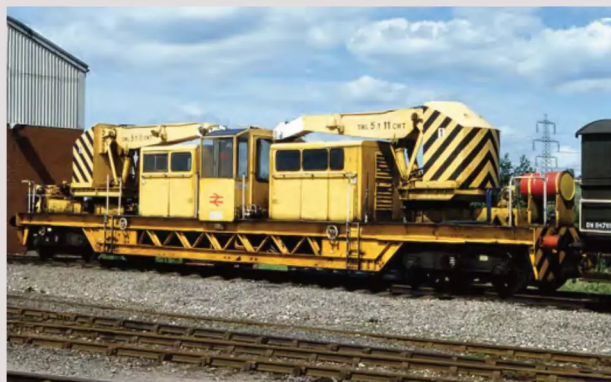
ABOVE: The Smiths-built track relayers undoubtedly had a presence with their sturdy underframes and sizeable counterweights on the back of the cranes. These were also the first of the self-propelled track relayers, DRS78203 dating from 1965. Seen at Beighton on June 23, 1985, it was scrapped in 1999 after passing to Balfour Beatty ownership. Trevor Mann
