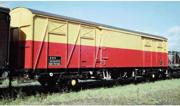
ABOVE: Repainted in Satlink colours but otherwise unaltered, 20-ton ferry van KDB787285 was at Radyr during September 1991 and recoded as a ZRX. Like the former VDA vans, these were used to move stores to and from S&T depots, providing both weather protection and security. David Ratcliffe
