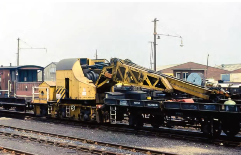
ABOVE: Another Taylor Hubbard product but this time a light duty diesel electric type, DM1764 (later DRT81264) was a unique crane. Built in 1960, it was the first experiment into using a telescopic jib as BR looked to develop a new group of cranes that could work under overhead electrification. Although innovative, it was limited to lifting just 6½ tons. Seen at Watford Junction on July 7, 1979, it had Plate wagon DE250526 as a runner and would be scrapped in 1988. Simon Bendall Collection
