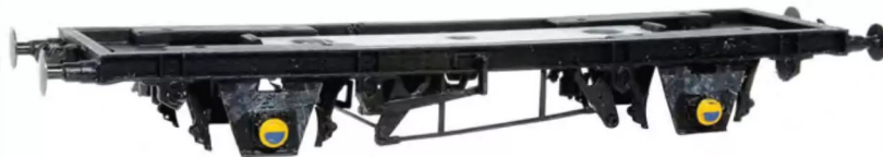
The Bachmann chassis is pictured following the removal of the moulded springs. While initially messy, the scars will be covered by the new castings.
