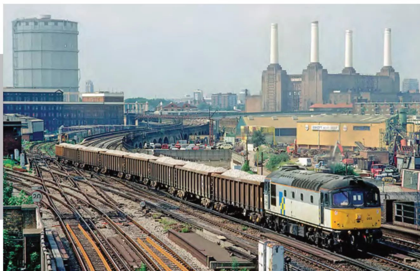
RIGHT: An early deployment of the high capacity bogie box wagons was to deliver the vast quantities of ballast needed for the construction of the Channel Tunnel terminal at Cheriton, Dollands Moor freight yard and all the new connecting lines. On July 16, 1992, 33053 approaches Wandsworth Road with the 6068 Temple Mills-Hoo Junction for onward transfer, this featuring eight JNA and KEA boxes. Such wagons would be trialled on possession work by BR and later Mainline Freight during the middle of the decade, but they proved unsuitable.
