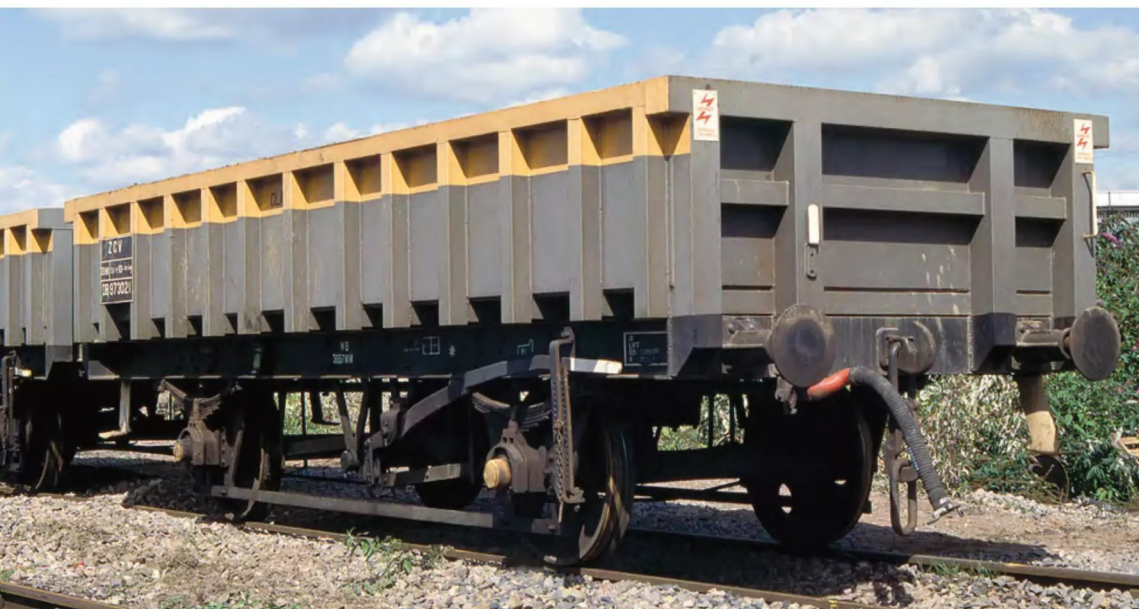
LEFT: The ZCV Clam conversions saw a new box body added to the existing vacuum-braked underframe. DB973021, which was rebuilt from B432845 by Powell Duffryn, is seen at Radyr on August 25, 1991, and shows the separate number plate employed on the wagons converted by the company. Trevor Mann
