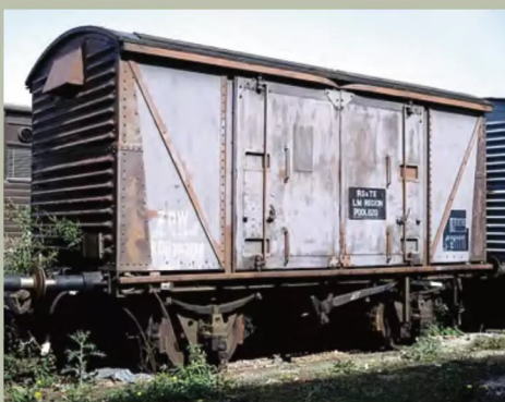
ABOVE: In contrast, you would be hard pressed to tell that shock van KDB853768 was even in S&T use if it were not for the 'KD' prefix added in front of the wagon number. Built to diagram 1/218, all the other markings were as per revenue use when seen at King's Lynn on August 28, 1979.
