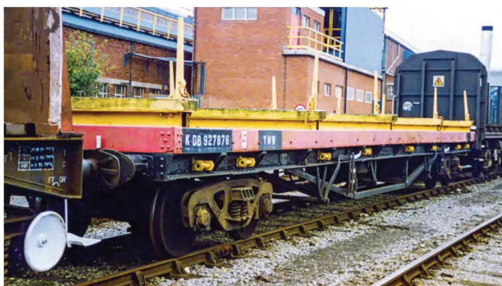
LEFT: Not all of the Bogie Bolster D wagons were converted to air brake and became BDAs, One such example was KDB927876, which was taken into S&T use for carrying assorted long loads, becoming a YNW. However, when seen at Allied Steel and Wire's Tremorfa Works in Cardiff on October 24, 1993, it was back in revenue-earning traffic but neither recorded nor repainted. Hywel Thomas
