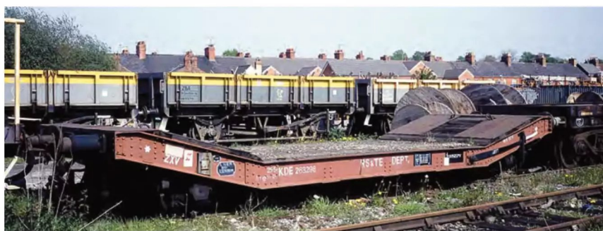
RIGHT: The S&TE retained a number of Lowmacs to carry bulky items. One of these, ZXV KDE263298, is pictured at Chester S&T sidings on May 2, 1994, this being a 25-ton rated Lowmac EP. David Ratcliffe
