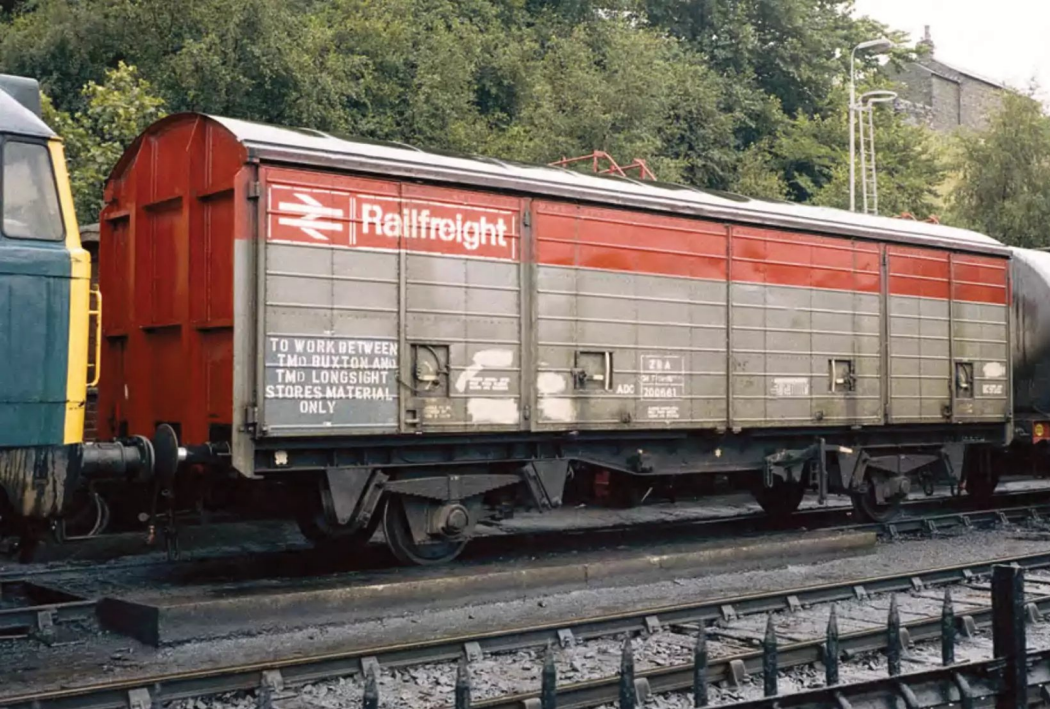
LEFT: While most of the air-braked vans in the M&EE fleet were in a nationwide pool, a handful were assigned to a specific circuit working. Once a VDA, ZRA ADC200661 was lettered 'To work between TMD Buxton and TMD Longsight. Stores material only' when found at Buxton in July 1985. David Ratcliffe
