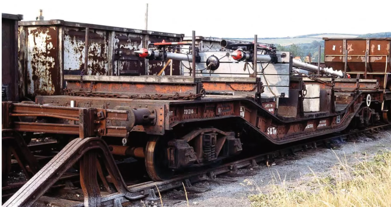
ABOVE: Former Warwell KDM721216 had been rebuilt as a Bogie Bolster B in 1949. Later assigned to the S&TE, it was recorded at Burry Port in August 1981 while carrying a new double bracket semaphore signal, complete with arms in place. The wagon is lettered 'Empty to Neath'. Trevor Mann
