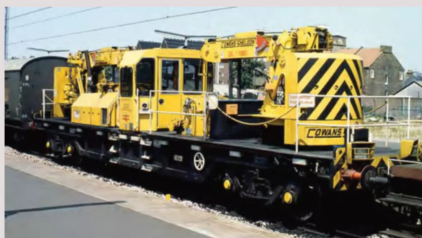
ABOVE: Cowans Sheldon also provided 14 track relayers to BR in 1980 with DRC78236 recorded at Bedford in July 1983. Very similar in design to the Plasser version but with more bulk, it was scrapped in 2007 after seeing use with Centrac, GTRM and Carillion. Two sister machines remain in use with Colas Rail. Simon Bendall Collection
