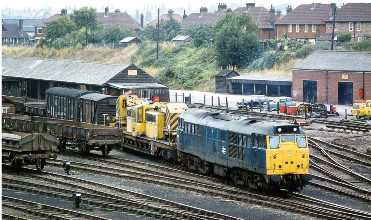
ABOVE: During September 1981, 31245 awaits departure from Ipswich engineers' yard with one of the imposing Thomas Smith track relayers in tow, this being a self-propelled example. Accompanying it is a 12-ton van along with a Southern Railway-design Parcels and Miscellaneous Van (PMV) which has been converted into a staff van.
