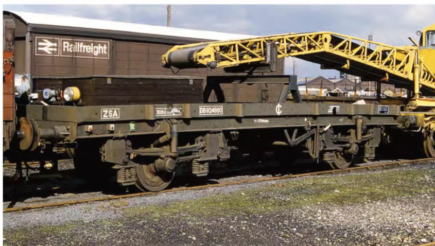
LEFT: The other two Bogie Bolster E wagons rebuilt as part of the project did not qualify for the Pollock name, these becoming runner wagons instead. ZSA DB924860 is seen at York Leeman Road on August 20, 1985, when in use as a support wagon for the conveyor of Plasser & Theurer unloading station DR88201. This machine worked with a ballast cleaner and the Skate skip-carrying wagons as a spoil handling system. Notably, the wagon still retains its stanchion pockets down the sides and the leading end is fitted with headlights and a warning klaxon. It was condemned in August 1994 and scrapped the following year. Trevor Mann
