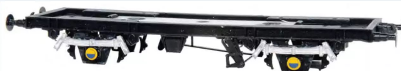
The new S Kits parabolic springs are seen glued in position and awaiting a coat of paint.
