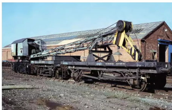
ABOVE: Recorded at Northampton engineers' yard on October 21, 1979, DRT81033 (DM1433) was built by Taylor Hubbard in 1958 and allocated to Watford for much of its life. Both runners are repurposed ex revenue stock with the nearest, TDM311891, being an ex LMS double bolster, while TDB917090 was built by BR as a single bolster wagon. Simon Bendall Collection
