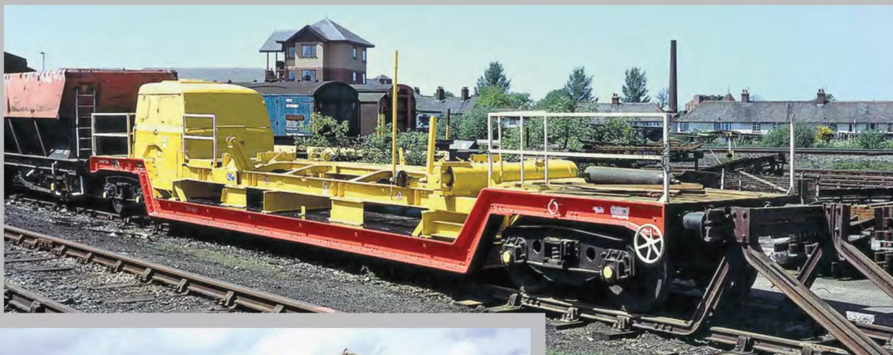
ABOVE & LEFT: One of several specialist conversions for S&T use was Flatrol MDD KDB900429, which had been converted to a 'Mole' wagon, complete with a former lorry cab! The contraption was seen at Carlisle Currock in May 1990 after receiving Satlink colours. Two years later in June 1992 and at the same location, it had been joined in a supporting role by ZGV Highfit KDB477209. David Ratcliffe
