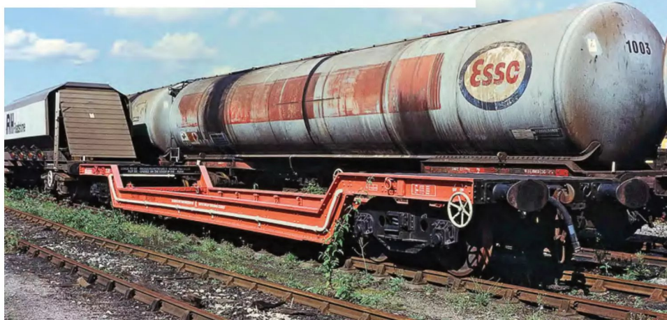
ABOVE & RIGHT: The Weltrols were a useful addition to the S&T fleet, duties including carrying scrap material, such as signals, away from worksites while they could also be used to move portable buildings. When seen at Tees Yard in February 1992, dual-piped KDB900935 was sporting full Satlink livery while vacuum-piped sister KDB900937 was only in all-over signal red at Radyr in August 1991. David Ratcliffe
