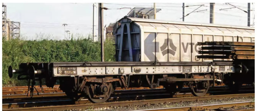
ABOVE: The former Plate wagon chassis that was DB935416 shows off its modified suspension and air brakes at Walton Old Junction, Warrington, on June 18, 1989. This had been modernised for its previous role of carrying coal containers while the grey look was standard for these ZEB. Trevor Mann
