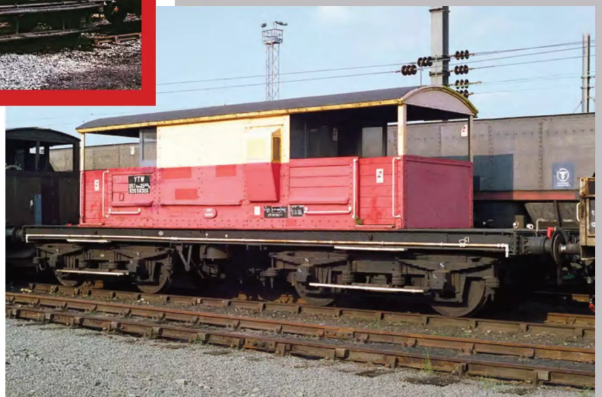
ABOVE & BELOW: In much the same way, Southern-design brake vans were also retained for personnel transport. On former Southern metals, the two-axle Pillbox design was quite common as typified by ZTP KDS56400 at Hoo Junction on February 12, 1995. Over two years later, YTW Queen Mary KDS56305 is seen at Warrington Arpley during May 1997. Although now in EWS ownership, it had performed a similar role earlier in the decade. Ian Cuthbertson/David Ratcliffe
