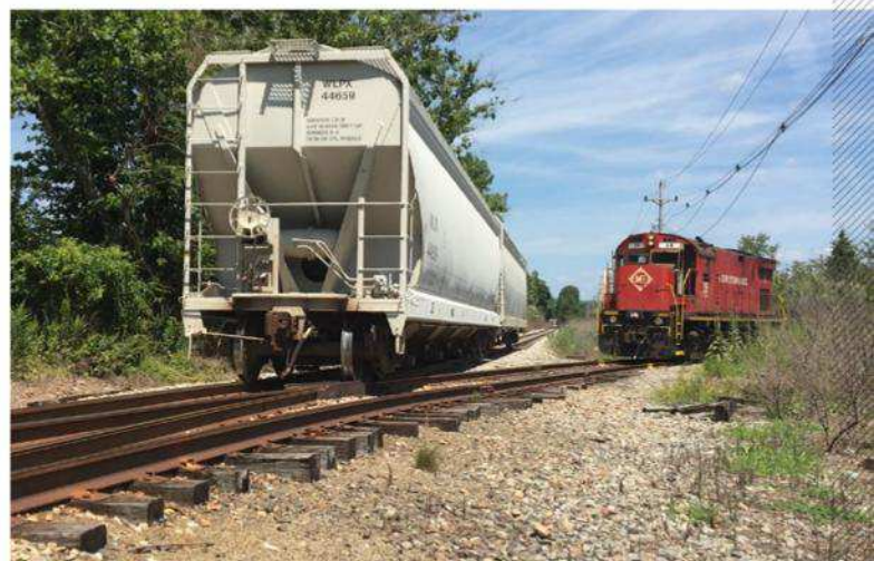
The crew gets around the train by making a gravity drop on the D&R Branch. The brakeman is riding the lead hopper.
