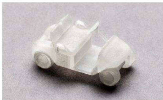
This is the 3-D cart straight from the printer and ready for painting and golfers.
