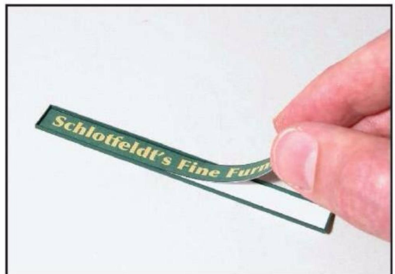
32 Use double-sided mounting tape to adhere the sign to the sign board.
