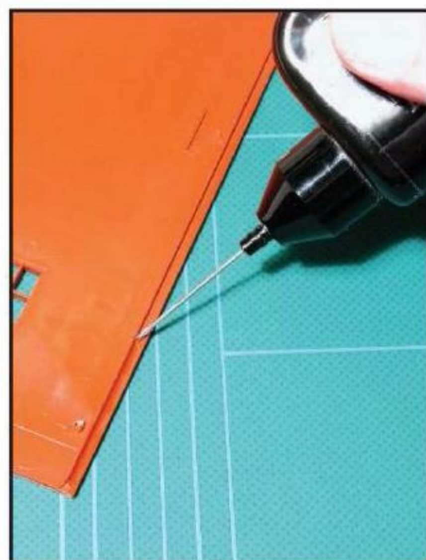
15 Apply thick plastic cement along the alignment lip inside one wall edge.
