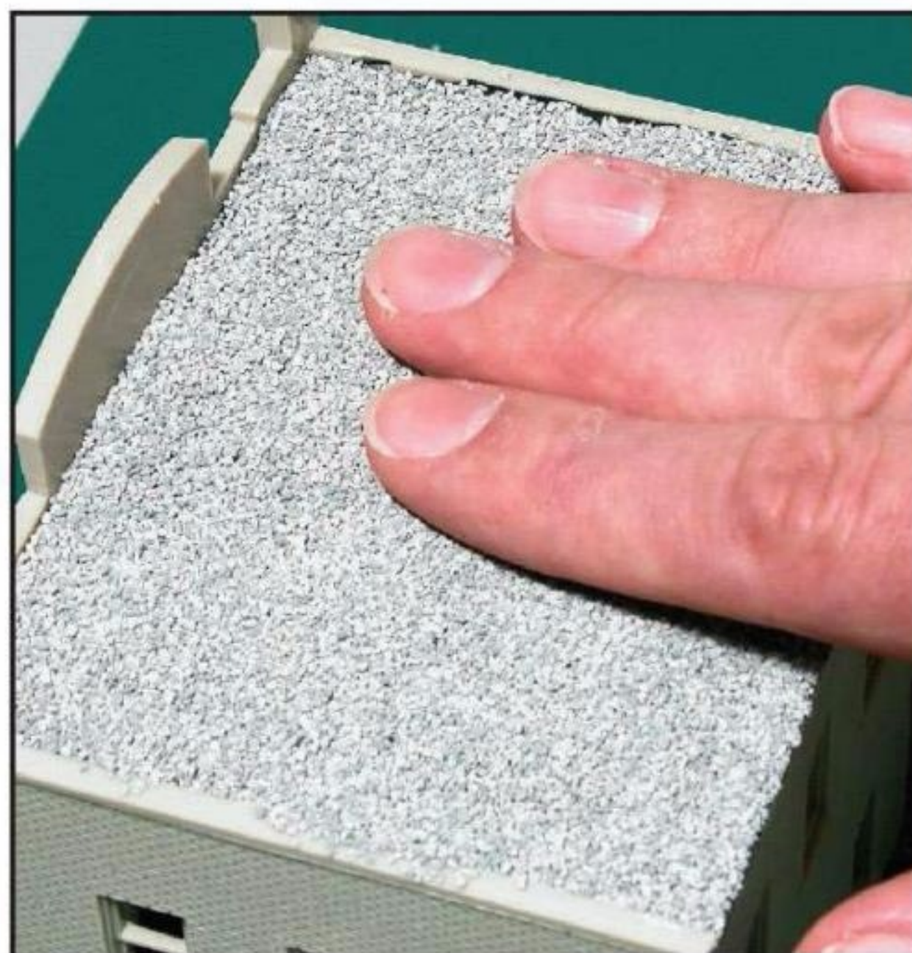
21 Press the ballast firmly into the paint before the paint dries.
