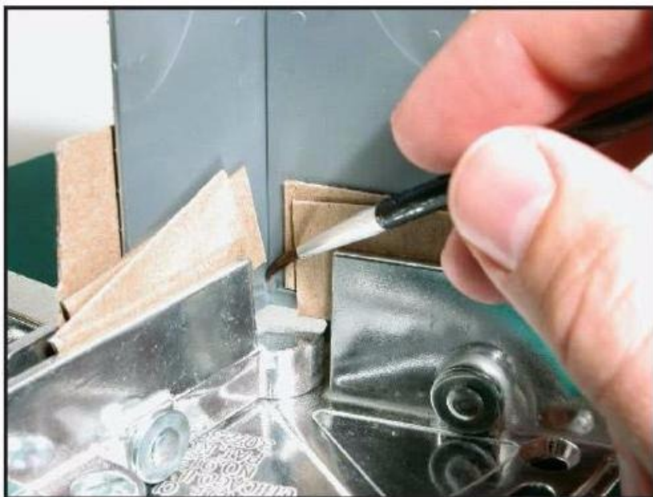
26 Pieces of cardboard protect the plastic roof from being marred by the jaws of the clamp. Apply glue to the rear of the joint.
