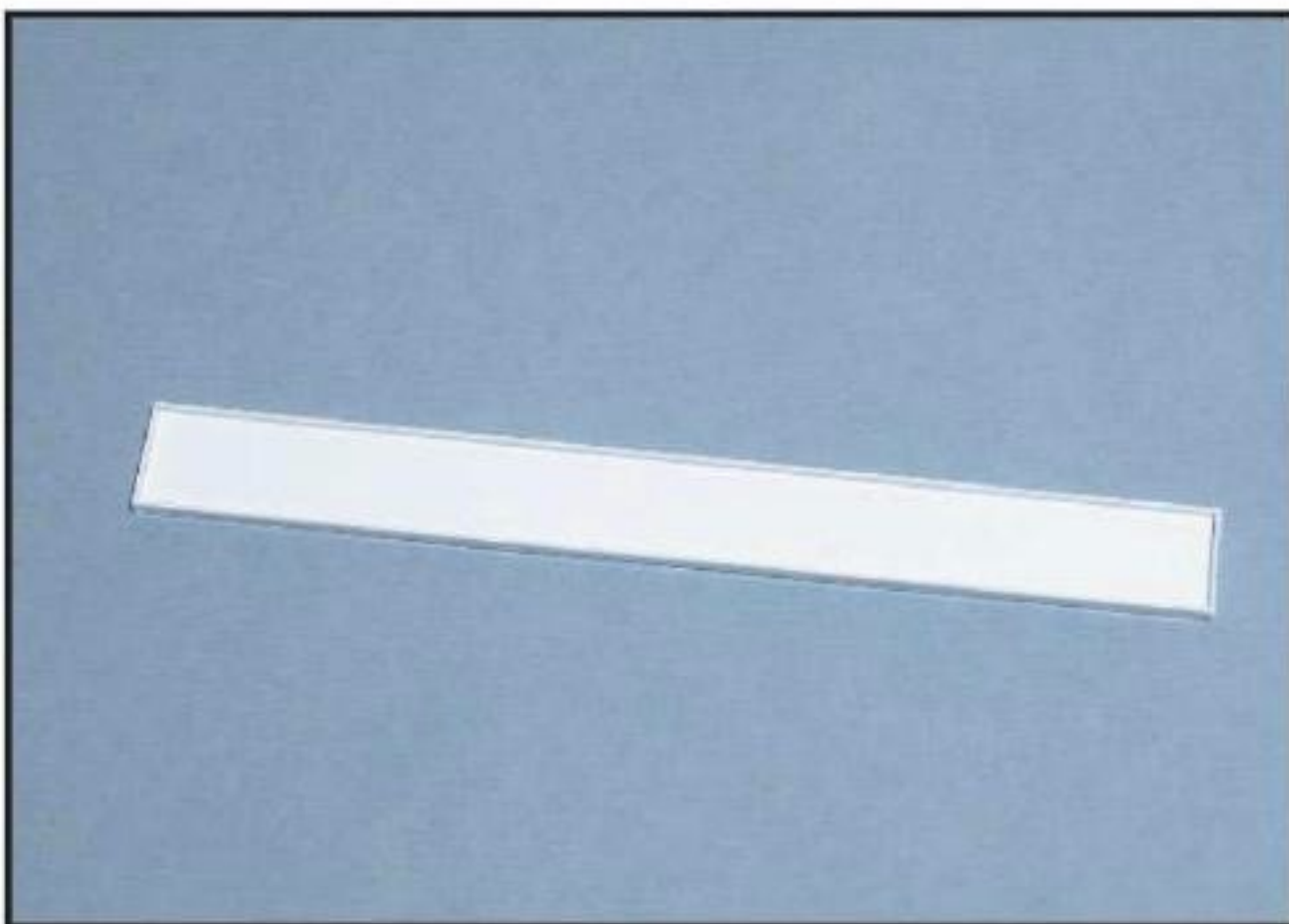
29 You can make storefront sign boards by placing styrene strip around the edges of styrene sheet.
