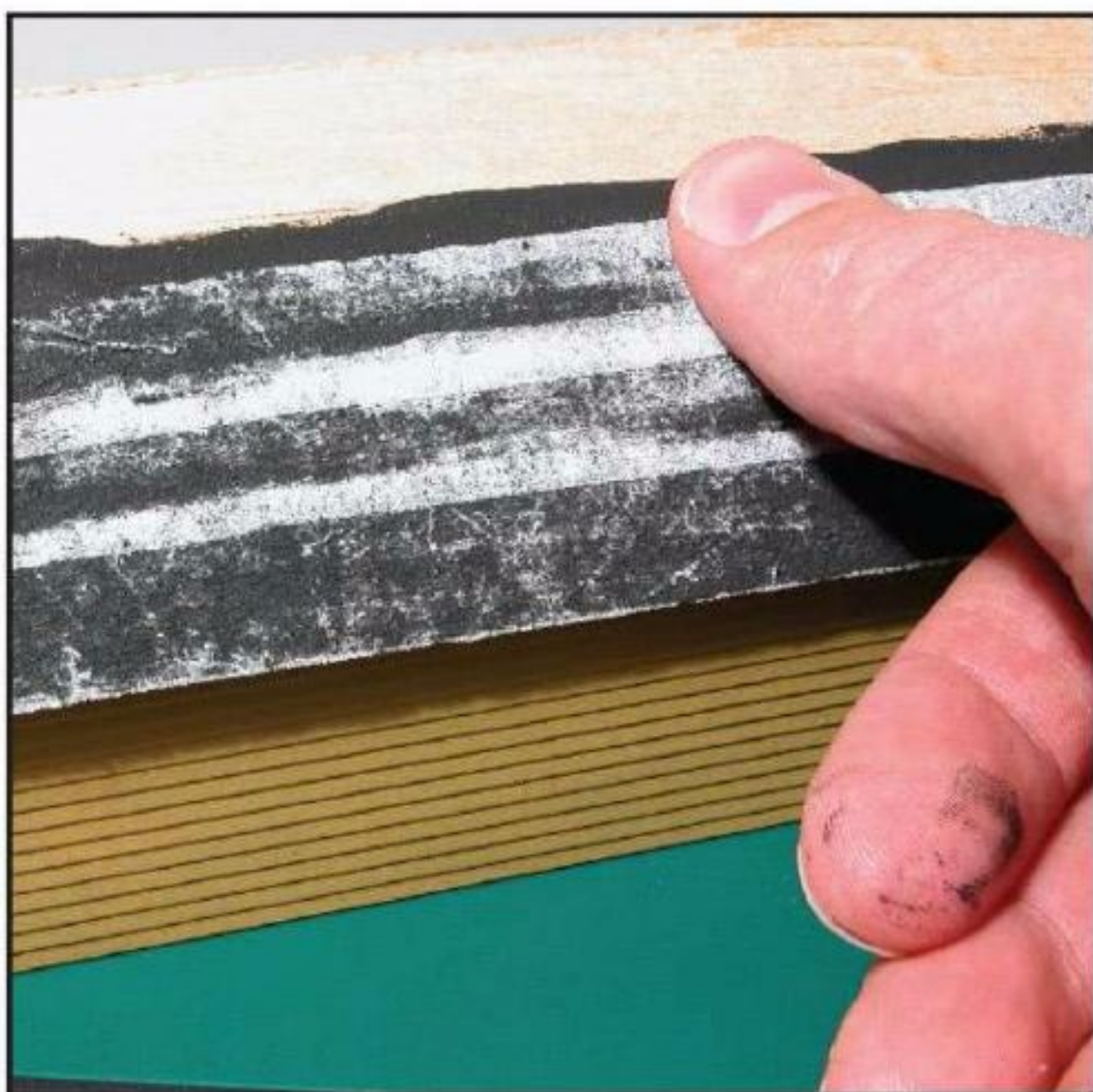
25 Press each strip lightly with your fingers to secure it in place
