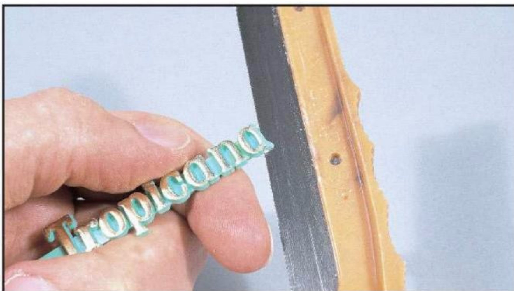
5 Letters can be cut from stir sticks with a razor saw and used on structure signs.
