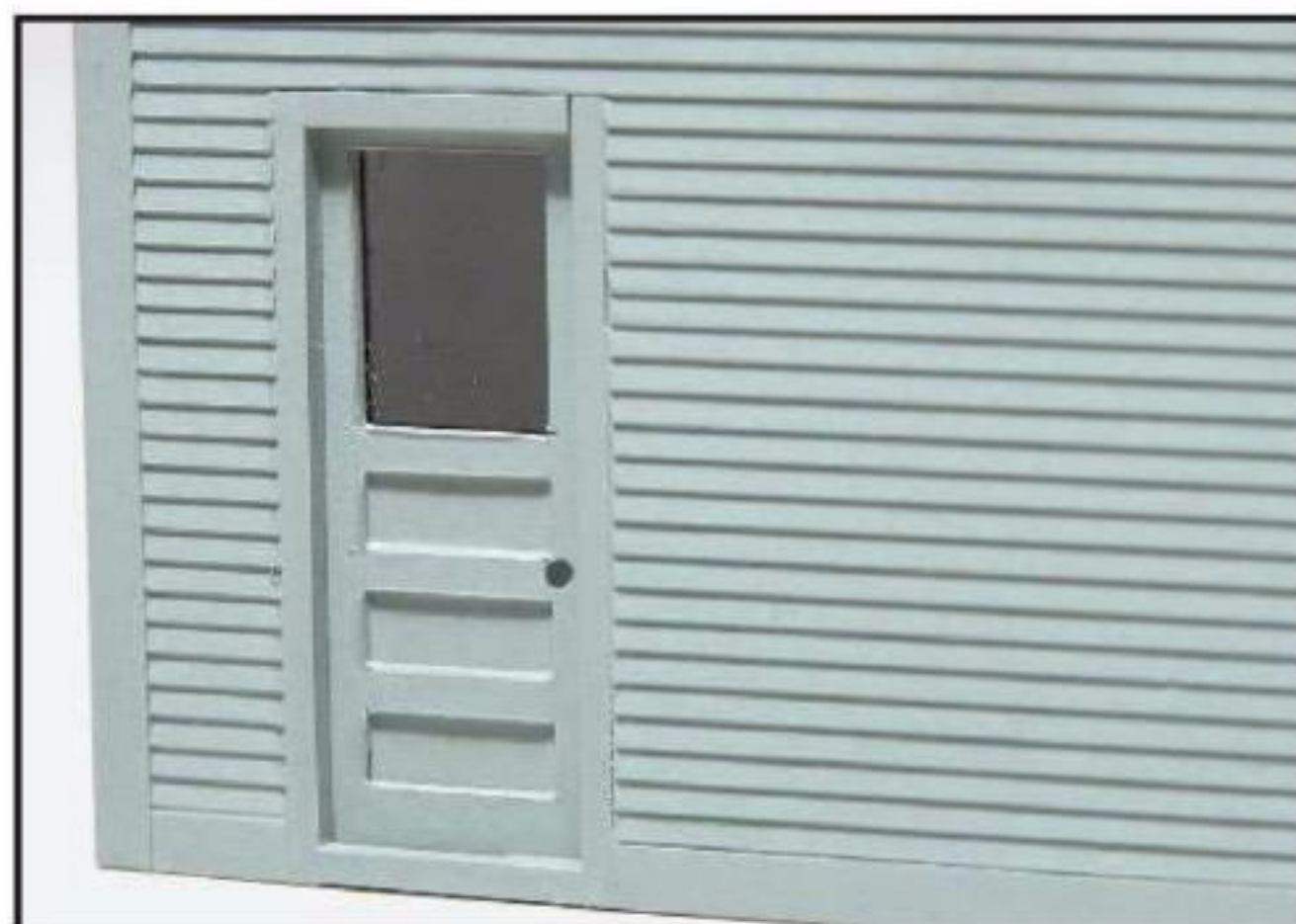
24 This panel door was made by layering two pieces of styrene after cutting the panel pattern in the top layer.
