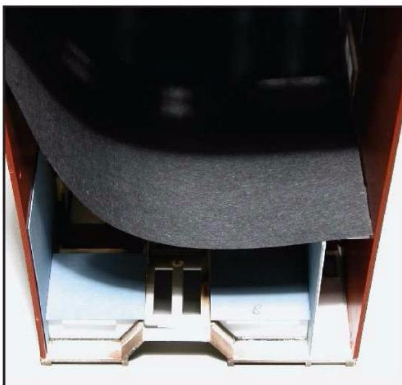
13 Add a view block behind each window well. This one, made from construction paper, prevents viewers from seeing through the structure's other windows.
