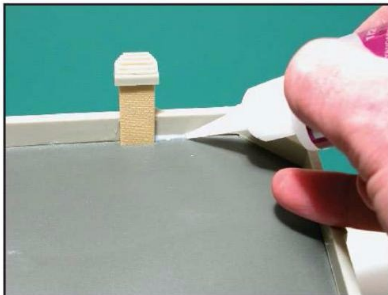
4 Fill any gaps around the roof with a bead of thick CA.
