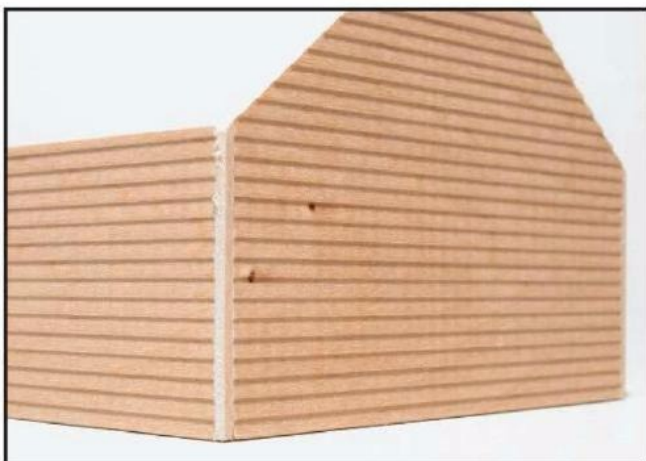
18 When finished, the corner post looks like corner trim boards.
