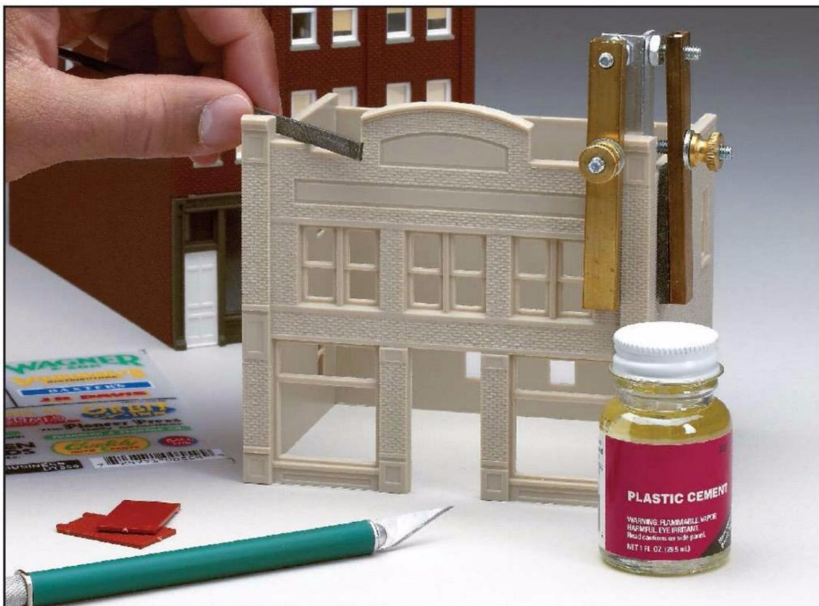
A few basic tools and glues are all you need to build most plastic structure kits, such as this HO scale Design Preservation Models brick storefront structure. Chapter 1 discusses building plastic kits like this one. Chapter 5 covers techniques for painting and finishing model structures.
