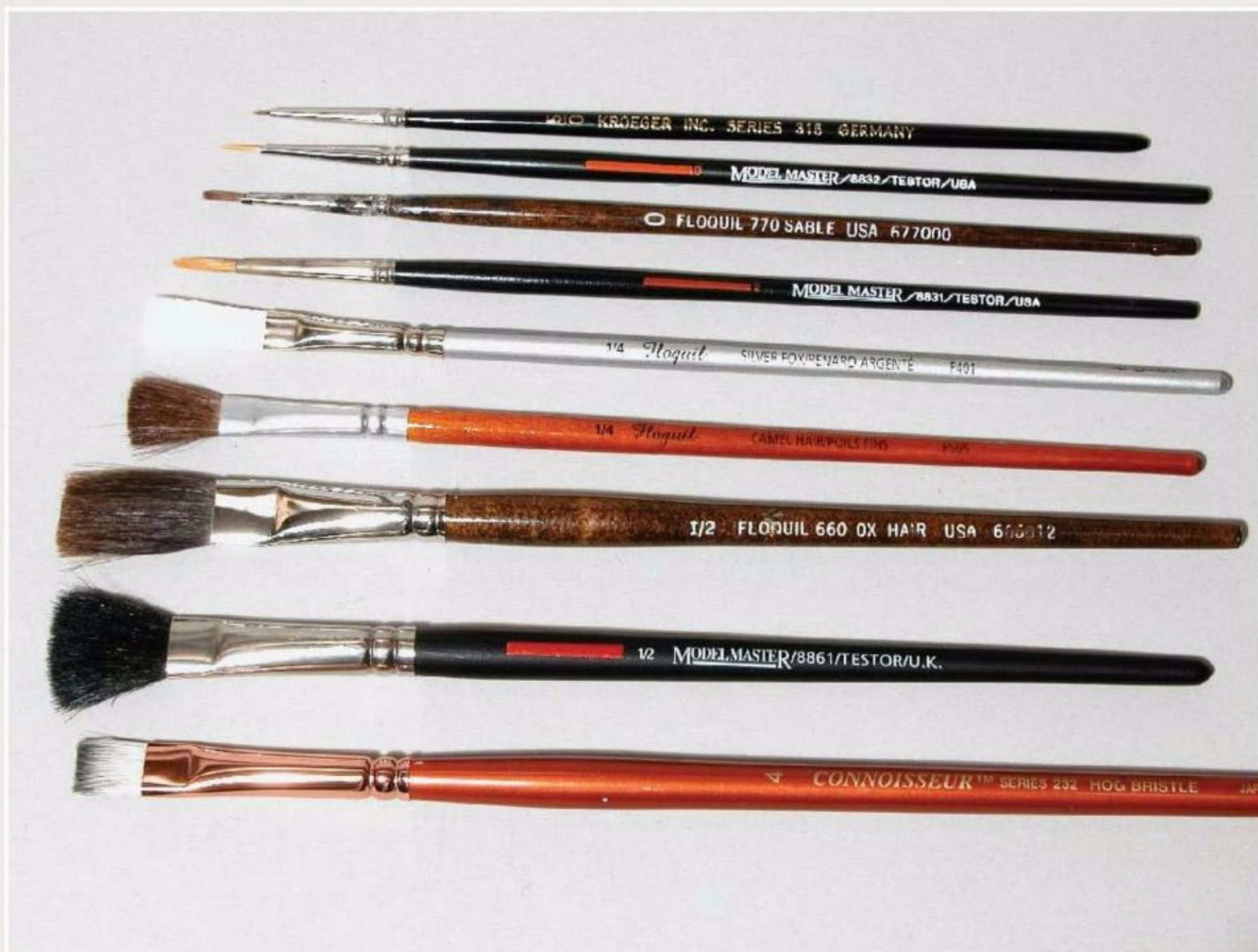
Paintbrushes the author finds useful include (from top) Kroeger No. 5/0 round sable, Model Master No. 0 round synthetic, Floquil No. 0 round sable, Model Master No. 2 round synthetic, Floquil 1/4" flat Silver Fox synthetic, Floquil 1/4" flat camel hair, Floquil 1/2" flat ox hair, Model Master 1/2" flat black sable, and Connoisseur 3/4" flat hog bristle.
