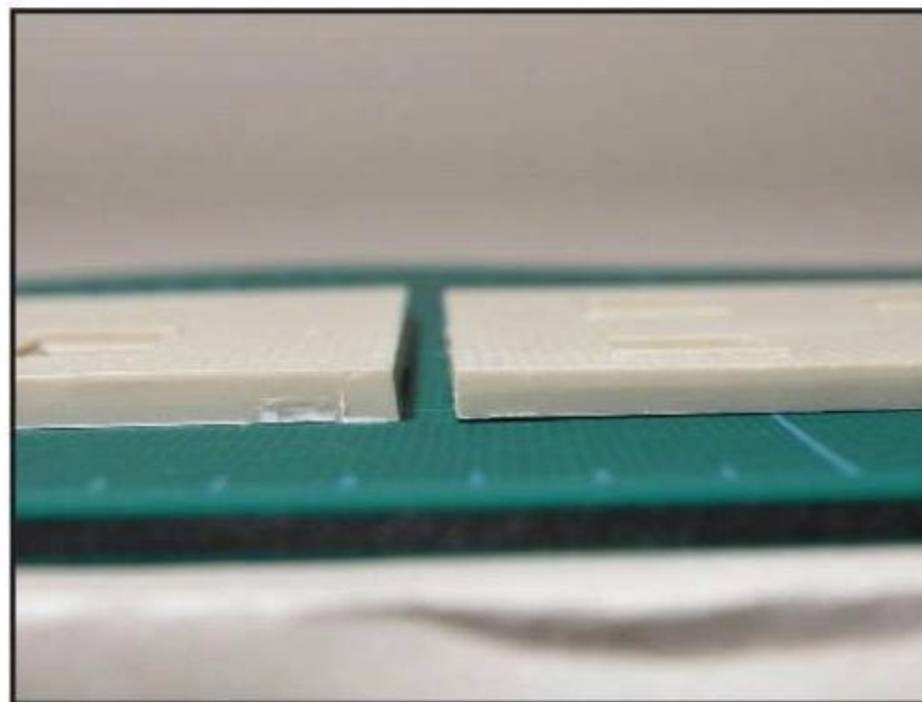
4 Make sure the mating edges of butt-jointed walls are square. The wall at right has been sanded and squared up; the wall at left has not.
