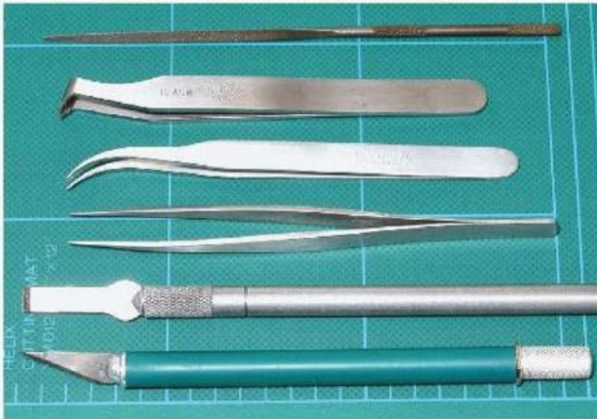
Handy tools include (top to bottom) needle files, sprue cutters, tweezers, and hobby knives with various blades.
