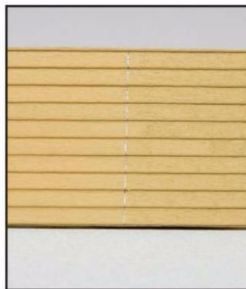
22 The paint on the left side is brighter because it was applied over a coat of primer. The wood grain is more prominent on the right, where Primer was not used.
