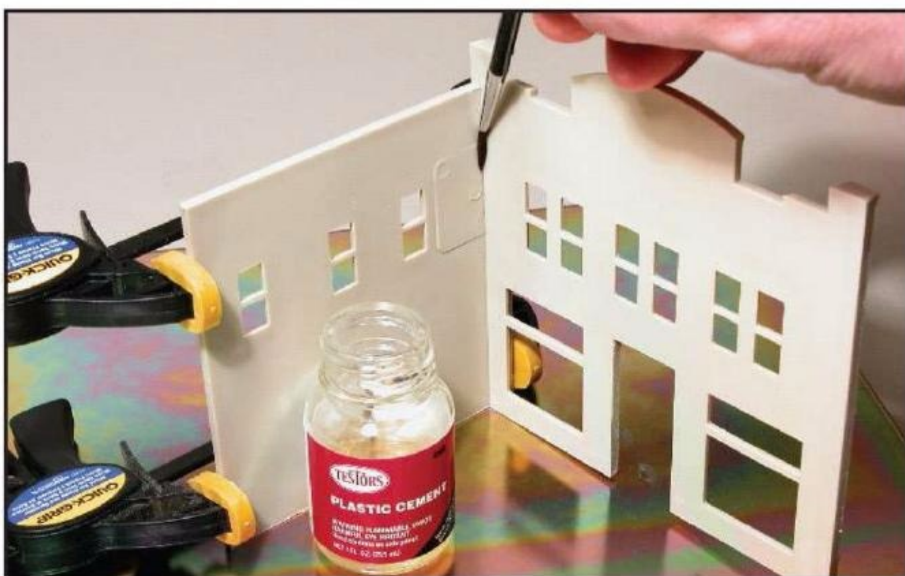
14 Apply liquid plastic cement to the rear of the joint with a paintbrush. Capillary action will pull the glue into the joint.
