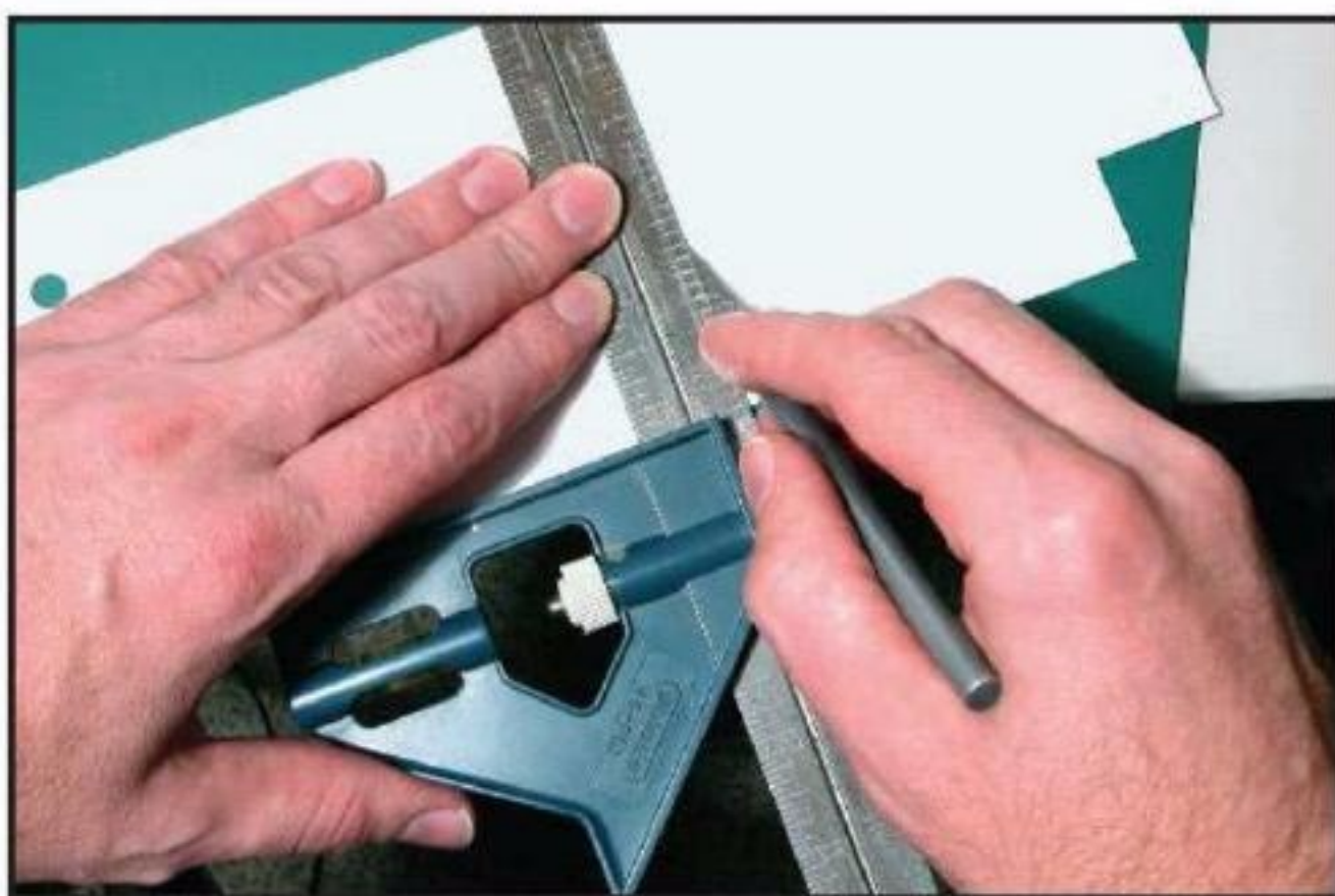
14 Using a combination square when cutting sheet material ensures a right-angle cut.
