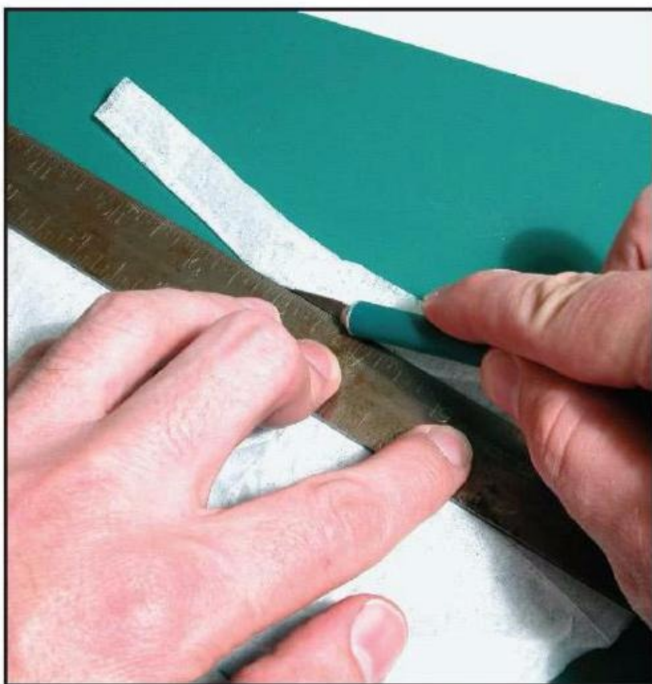
23 Hold tissue firmly with a heavy steel rule and cut it with a hobby knife, with the blade held at a low angle to the tissue.
