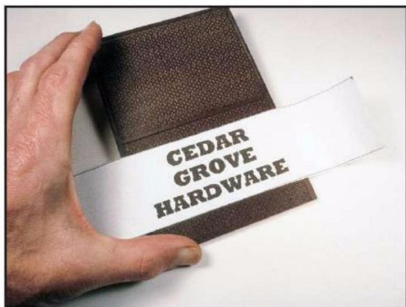
21 Lee Vande Visse made this stencil by printing out a sheet, then cutting out the letters with a hobby knife.
