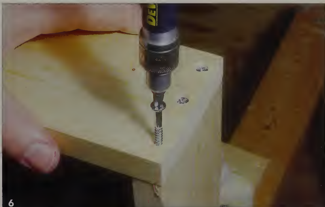
Screw the side to the end using drywall screws or 1 3/4" No. 8 wood screws.
