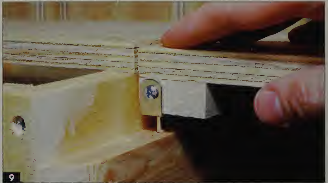
9 Carefully align the liftout and press it firmly in place.
