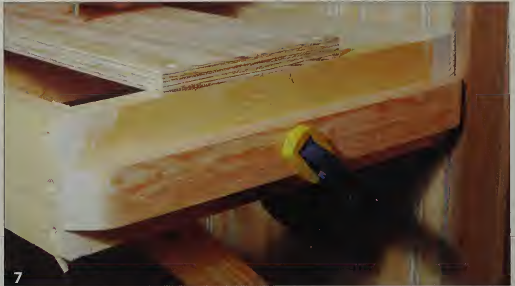
7 Clamp the 1 x 2 supports in place at each end of the benchwork. The ends have been rounded with a rasp and sanded.
