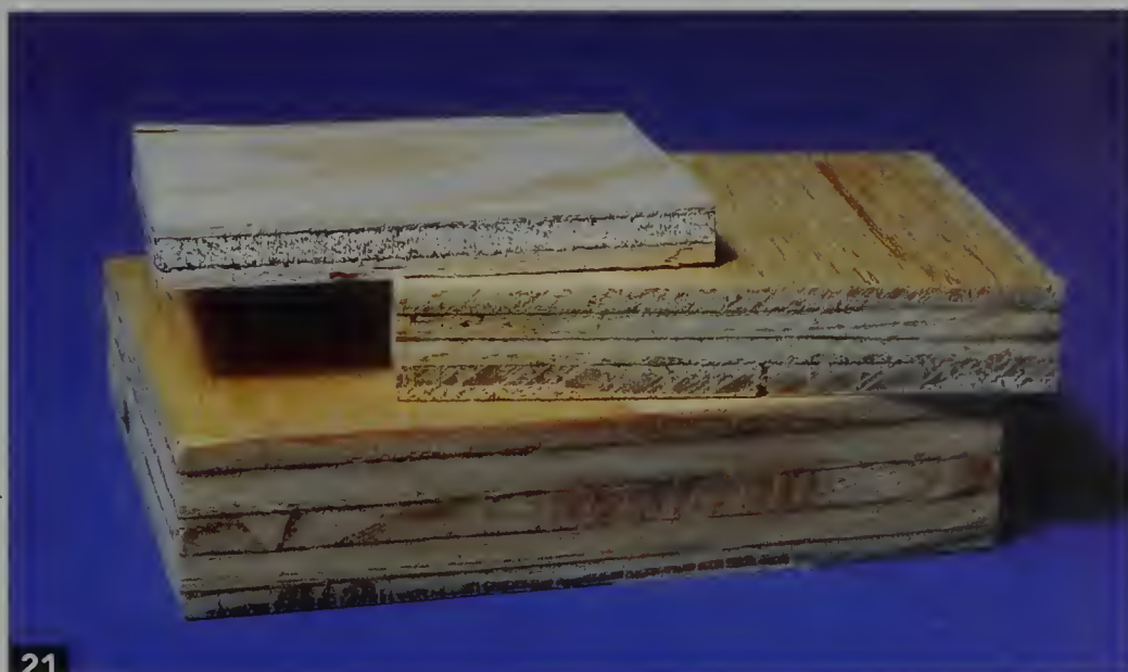
21 Plywood is made of three or more plies of wood glued and bonded together under high pressure. Shown here are standard 1/4", 1/2", and 3/4" pine or fir plywood.
