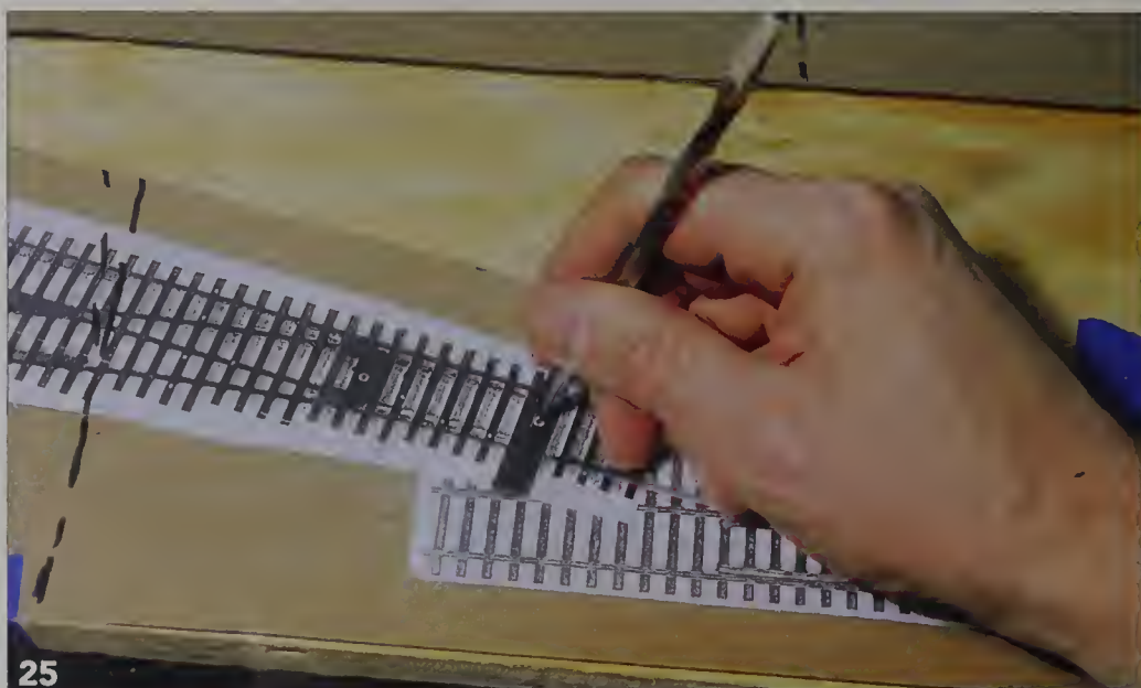
25 Mark turnout placement on the plywood by using a scribe or awl to poke an indentation at throw bar locations.
