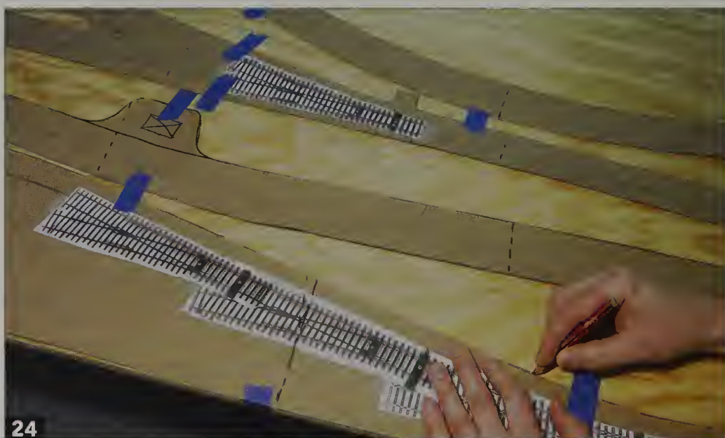
24 Tape the templates to the plywood. Outline them with a pencil or marker. Using photocopies ensures that there is room for the turnouts on the subroadbed.
