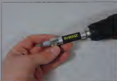
Quick-change reversible bits are very handy. This DeWalt bit has a collar that snaps in and out to release the head, which can be flopped end for end. The driver and drill bit are both replaceable, allowing you to change sizes and styles of bits as needed.
