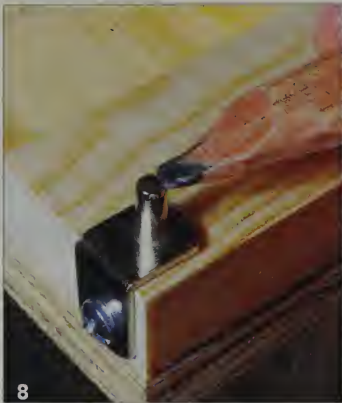
8 Mark the bottom of the each mounting pin with a pencil.
