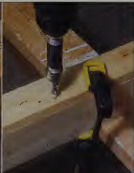
11 Spread glue on the top of the girder (in this case a 1 x 4) and then clamp the 1 x 2 flange on top. Secure the flange with drywall or wood screws every 12" or so.
