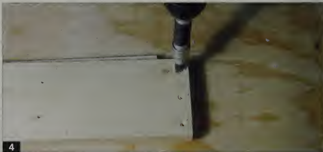
4 Drill three countersunk holes at the ends of each side 1 x 4 to attach the end pieces.
