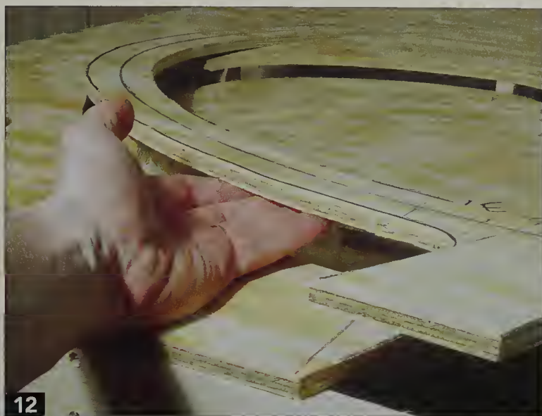
12 Once cut, the plywood subroadbed becomes very easy to move up and down.
