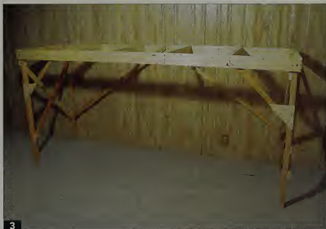
3 The first section is complete. The longer braces can be kept at the rear, providing better storage and undertable access from the front.
