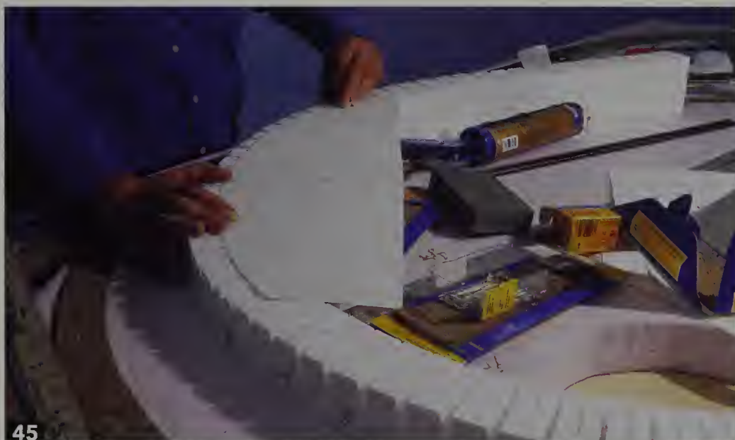
45 Curve templates can help determine riser locations. Test-fit track before gluing the risers in place.
