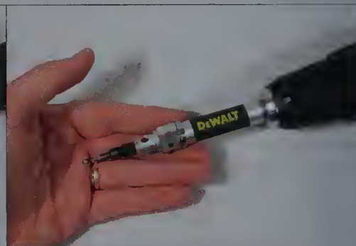
Quick-change reversible bits are very handy. This DeWalt bit has a collar that snaps in and out to release the head, which can be flopped end for end. The driver and drill bit are both replaceable, allowing you to change sizes and styles of bits as needed.
