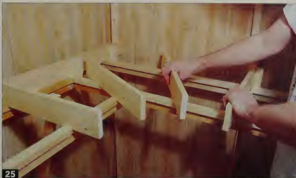
Joists can be positioned at almost any angle as needed around a corner, just like conventional L-girder benchwork.
