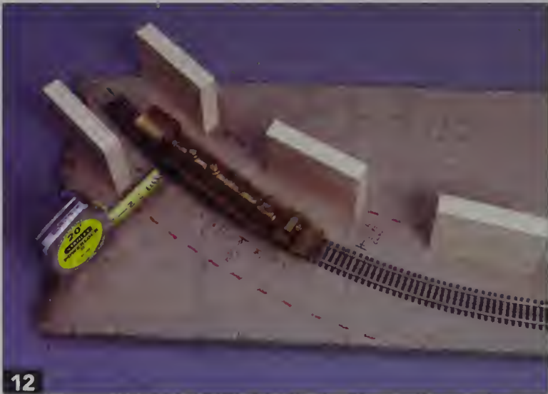
Before building his helix, Jeff Johnston checked the clearance needed for his equipment to clear spacer blocks at the required radius. This is especially important if you're building a double-track helix. Jeff Johnston
