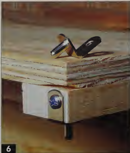
6 Screw a steel shelf mounting peg into each corner of the liftout section.
