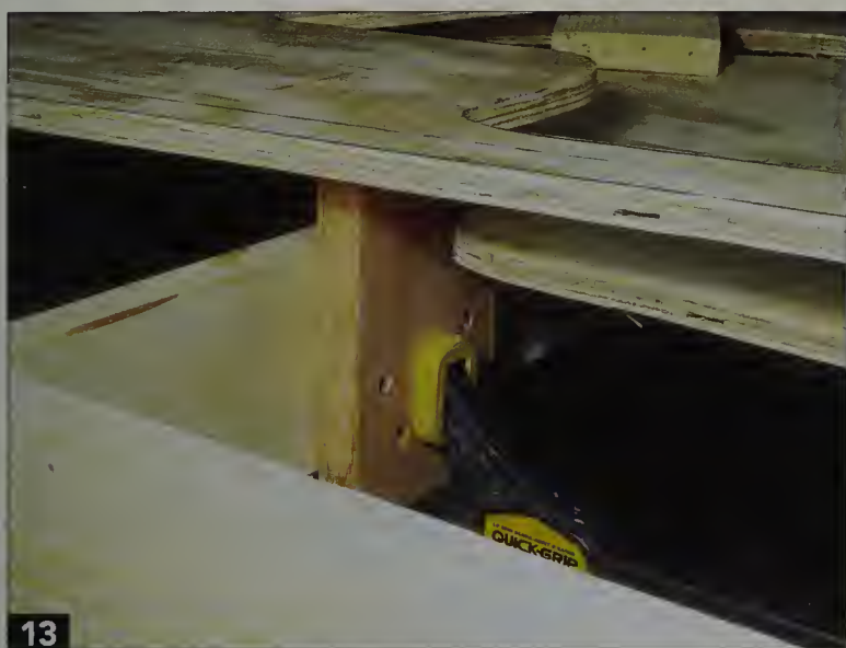
13 Clamp a riser in position at the subroadbed's highest elevation. Don't screw the riser or subroadbed into place.
