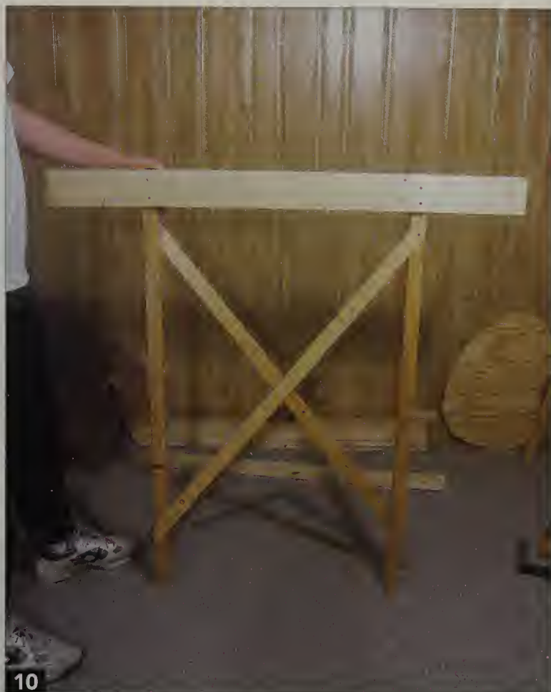
10 One leg assembly is complete and ready for the girders.
