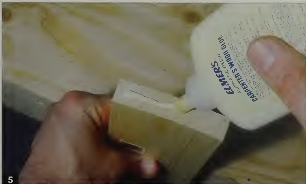
Run a bead of yellow carpenter's glue on the end of the end piece before screwing it in place.
