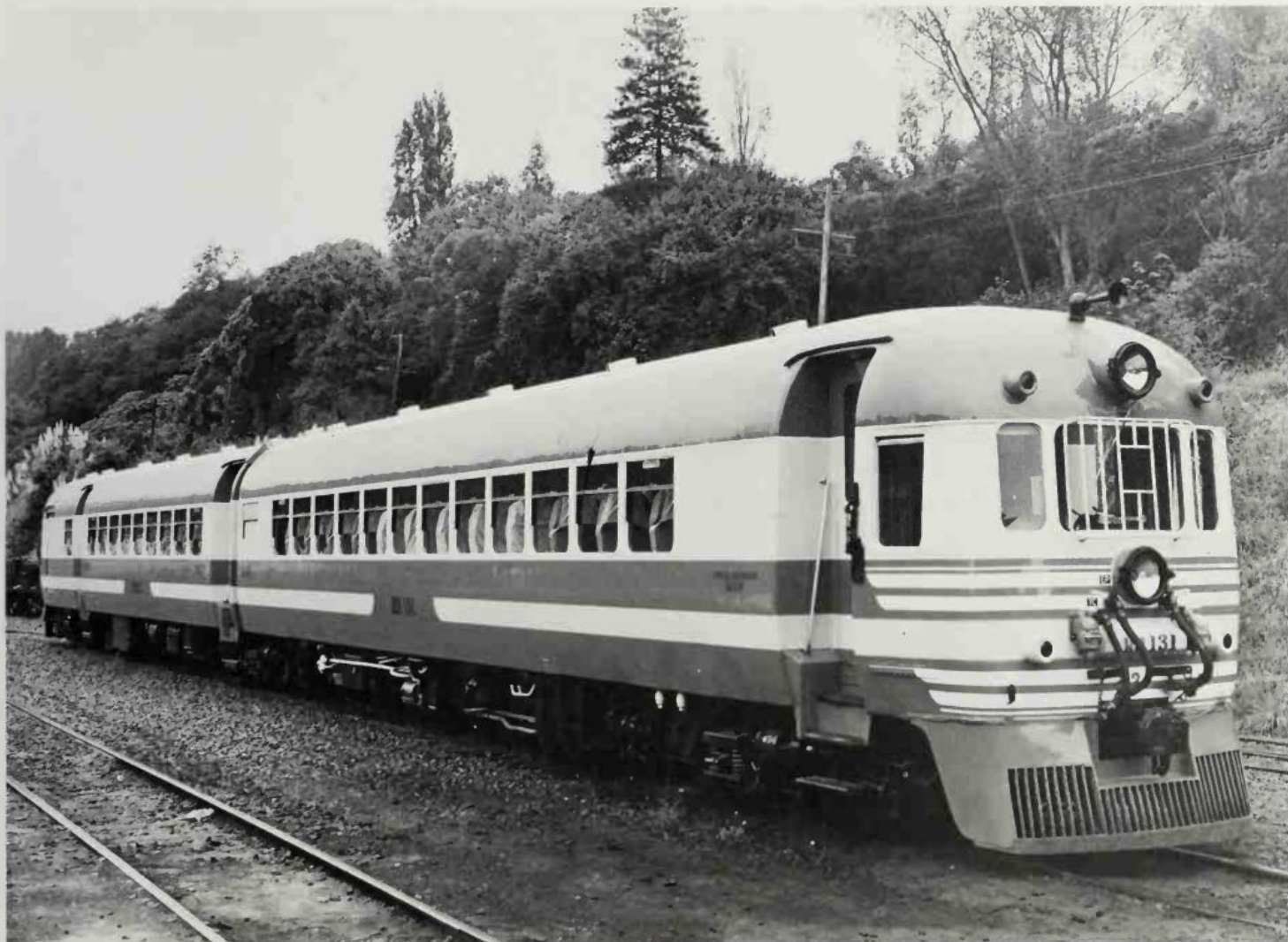
Above: A refurbished articulated two-car diesel train for the Hamilton-Auckland service.
