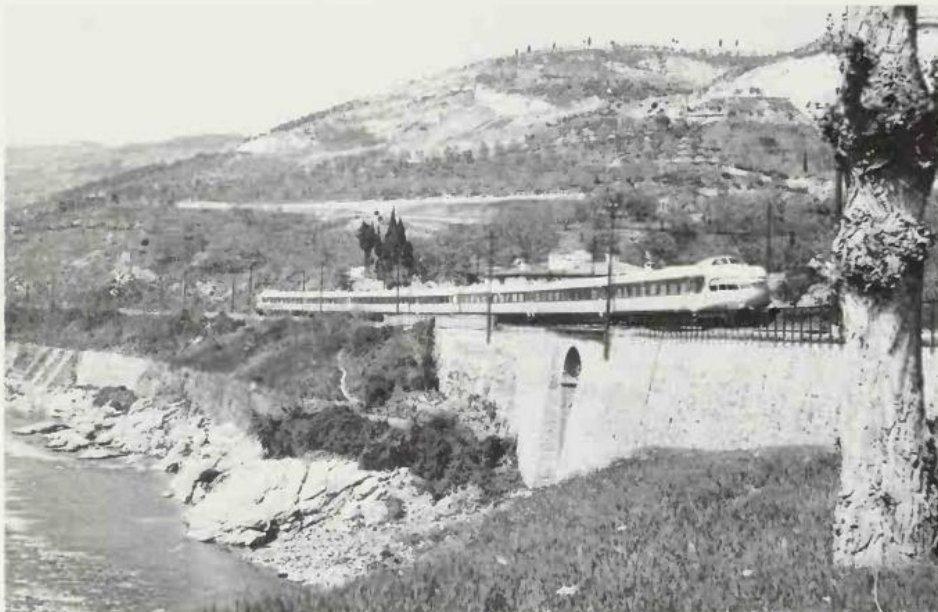
Above: The 'Settebello Express' is the Rome to Florence electric express train. The driver's cab is raised above roof level with an observation lounge below.
