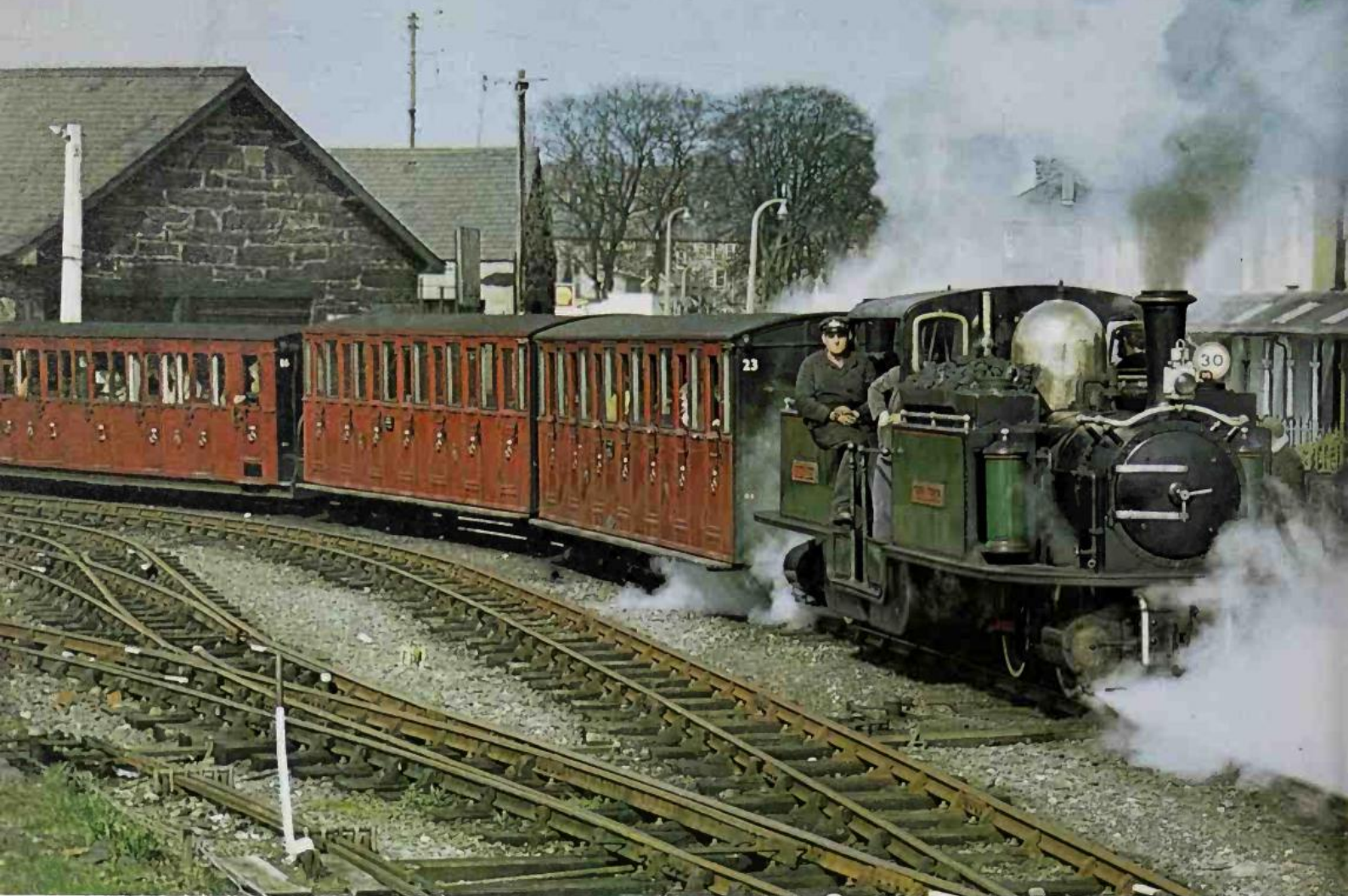
Above: A train leaves Porthmadog Harbour station hauled by Fairlie articulated locomotive along the narrow-gauge Festiniog Railway.
