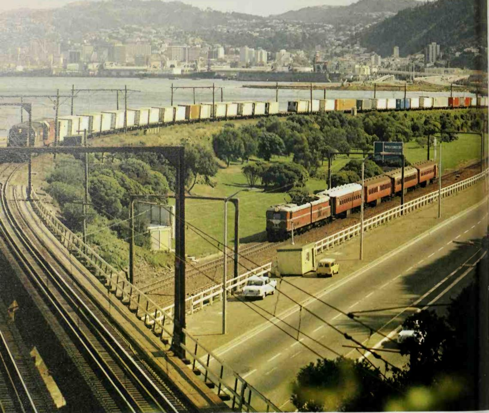
A northbound container freight train, hauled by two General Motors 'Da' class A1A-A1A diesel-electric locomotives, leaves Wellington, New Zealand while a local electric passenger train, hauled by English-Electric 'EW' class Bo-Bo-Bo diesel passes below.
