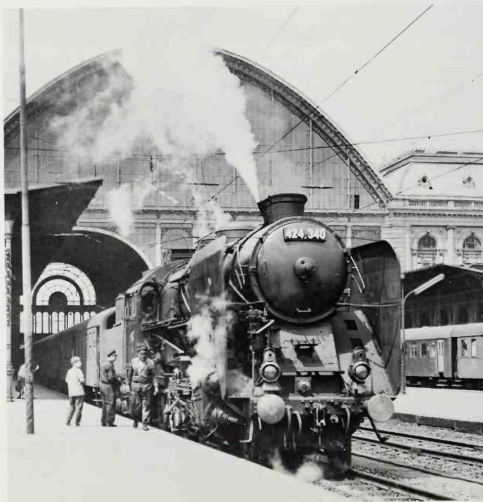
Right: A 424 class 4-8-0 locomotive with a fast train at Budapest East station in 1967.
