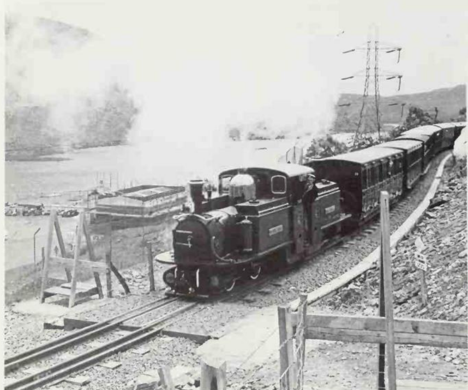
Above: Double Fairlie locomotive Merddin Emrys negotiates the new deviation line on the Festiniog Railway in June 1978. The old course of the line is now engulfed by the waters of the reservoir seen in this picture.
