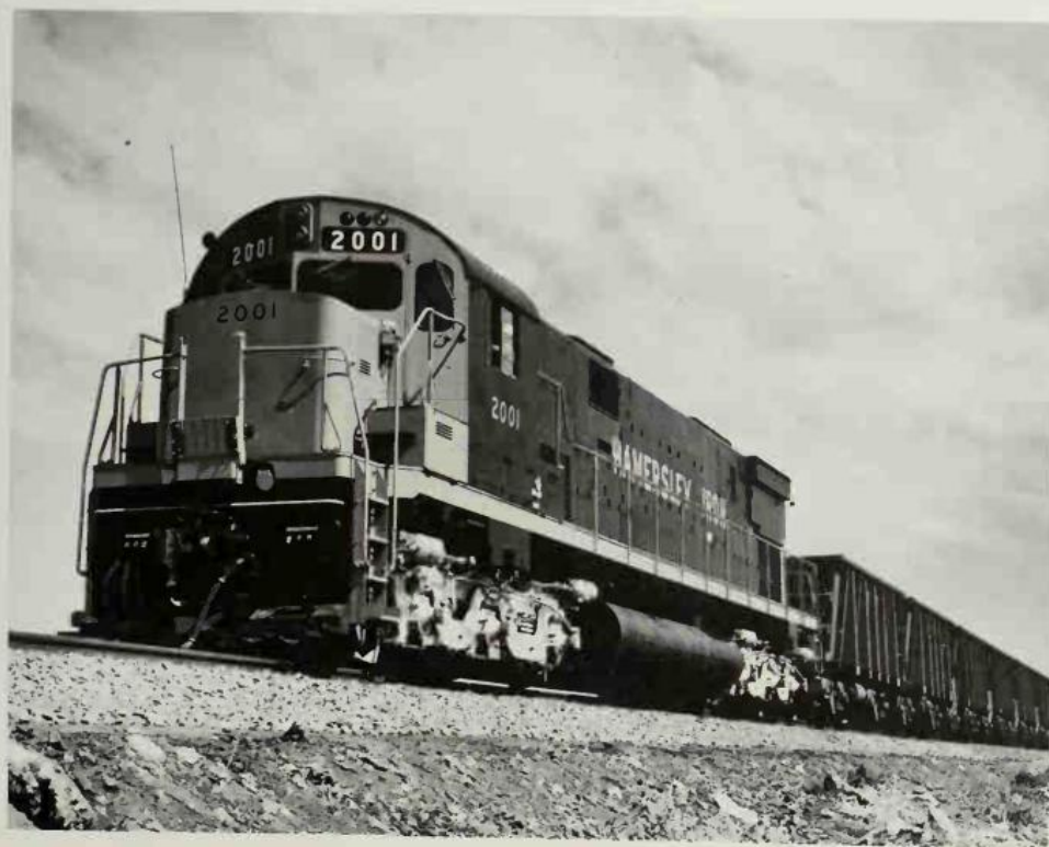
Left: The giant Mt Tom Price iron-ore train is made up of either 175 ore cars with two locomotives hauling, or 200 cars with three locomotives hauling. In the latter form it is 1.25 miles long and transports 20,000 tons of ore. It reaches speeds of 80 mph. This Hamersley Iron Ore train runs between Mt Tom Price in the north of Western Australia and the port of Dampier. The locomotives were made in Canada and the 100-ton capacity ore cars were made in Japan.
