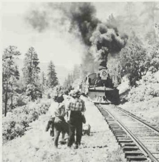
Below: The only section of the Rio Grande's once great network of 3 ft 6 in gauge track still to operate under its banner is the 45-mile Silverton branch out of Durango. Here one of the branch's Sports Models, 2-8-2 No 473 runs, decked out in fancy dress for a movie, alongside the Animas River.
