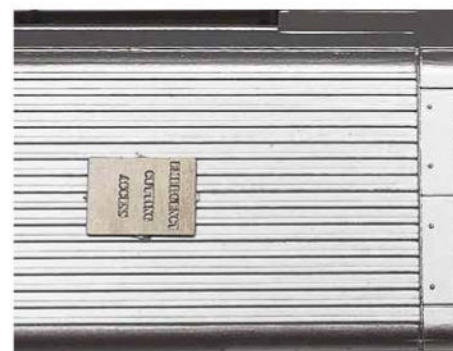
Tangara model fitted with emergency cutting access plate.
