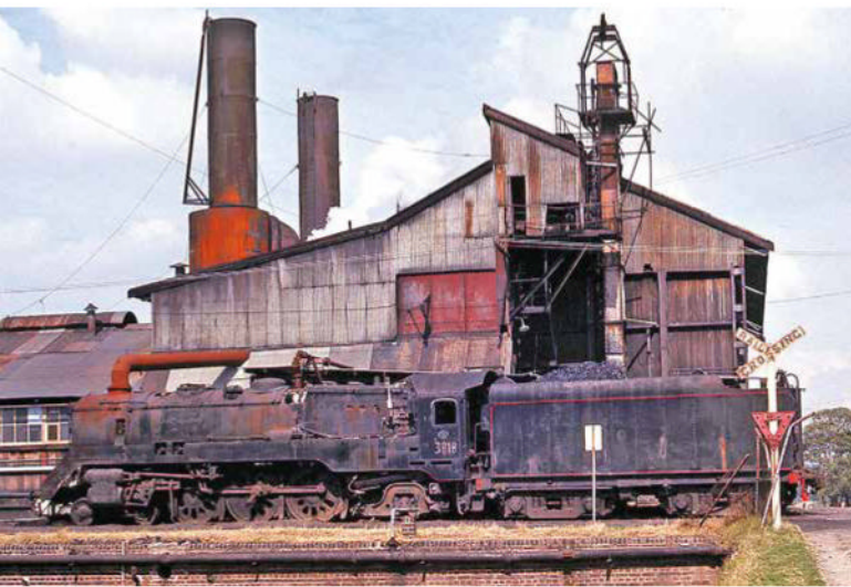
Locomotive No. 3818 in use as stationary boiler at the Homebush Abattoirs during the 1970s. Photo by late John Ward.
