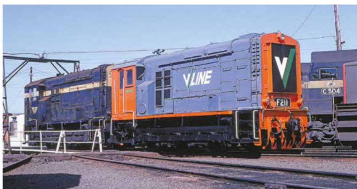
F class No. 211 Little Trimer in V/line livery and F212 in VR livery are stabled around the Dynon broad gauge turntable. Both members are fitted with a three-chime airhorn and had the buffers removed. F211 is fitted with a revised design headlight. Dynon 13th of Oct 1985.
