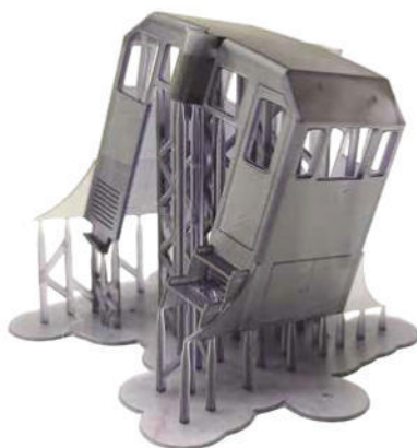
NSWGR NSWGR 79 Class, Australian National Railways DE class 3D printed cab.
