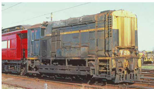
F class No. 216 (Ex SEC 2) at Newport 25th of May 1984 in a rather ratty SEC blue and gold livery, with a three-chime airhorn fitted to the cab roof, as well as a straight cowcatcher.
