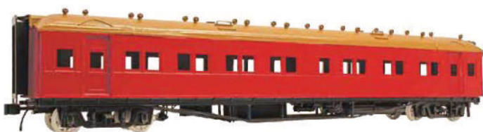
Painted pilot model 3D print of the VR W series coach.
