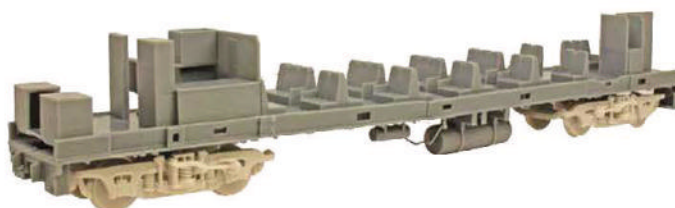
3D print of the frame and bogies of the H set series coaches.
