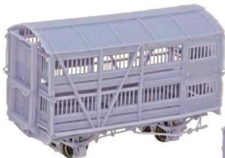
HON3½ Sfn four-wheel sheep van and Cfn four wheel cattle van unpainted kit shown, shunters steps and couplers not installed.
