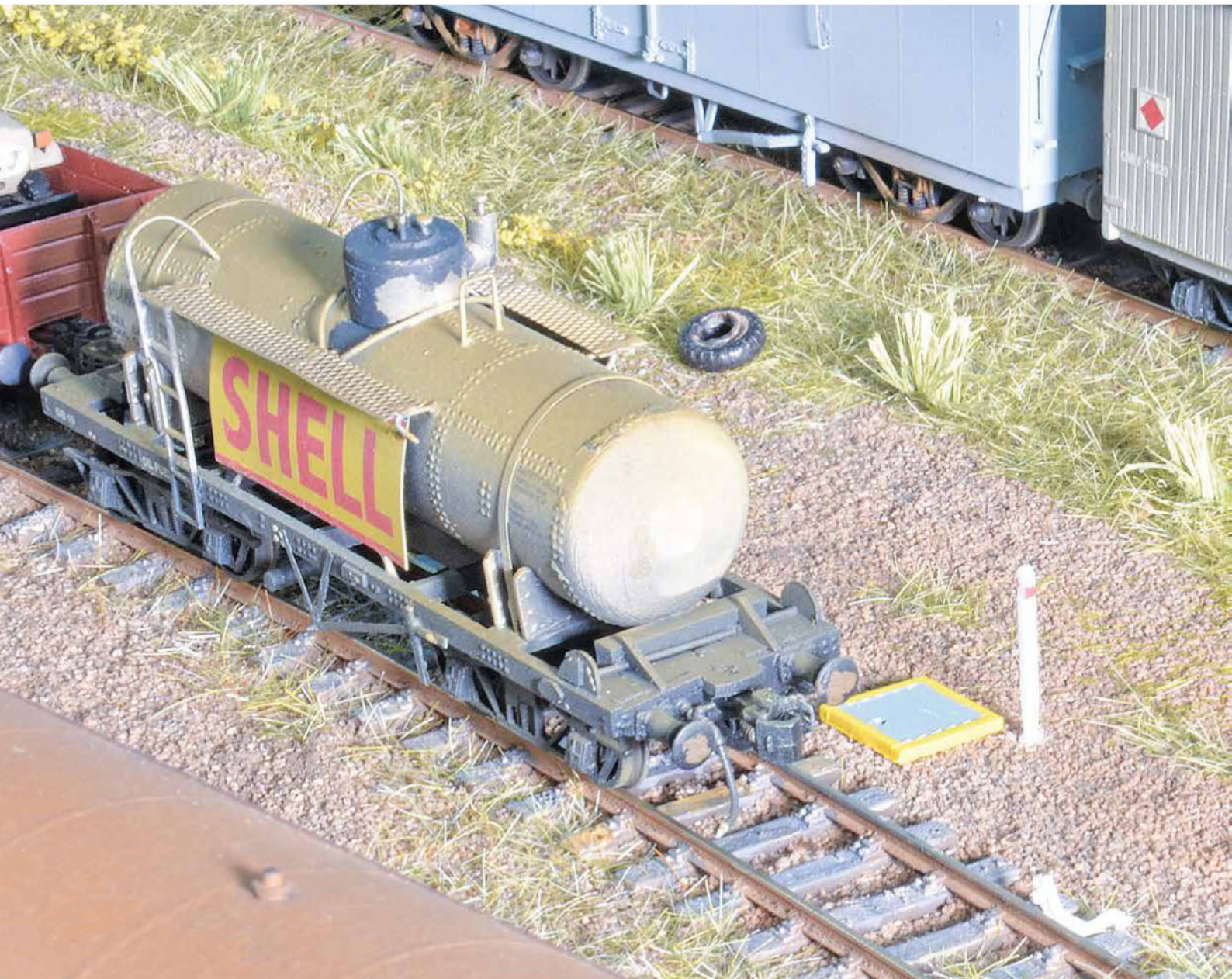
Not all fuel depots have a depot siding to unload their fuel. Some depots could be a block or two away from the railway line, so a pipeline connects the depot with the railway. The siding has a pit to couple a hose from the wagon to the pipeline. Sidings running off the main line are fitted with choke blocks, unlike the prototype to prevent runaway wagons coming out onto the main line, these are clearance markers.
