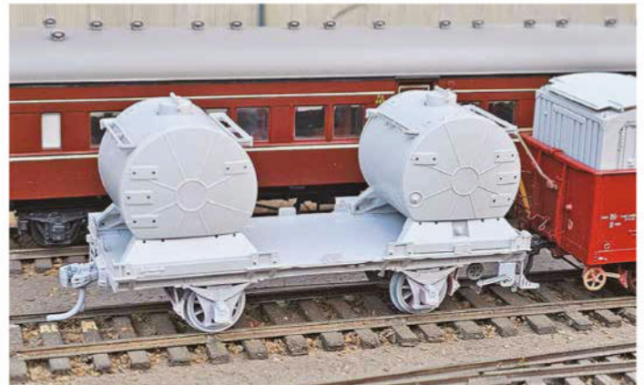
1st engineering example of the VR four-wheel KC LCL container wagon, and two Tallow tank containers.
