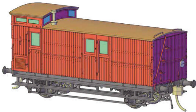
Digital rendering VR Z/ ZL timber-planked, four-wheel guards van with buffers.
