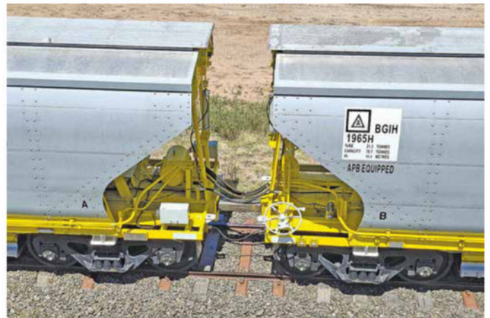
SSR BGIH No. 1964 and 1965H drawbar end detail, Rowena 17th of December 2025. Photo by Scott Fitzgerald.
