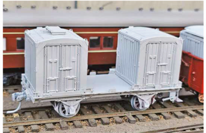
1st engineering example of the VR four-wheel KC LCL container wagon, and two LCL containers. Note the small door arrangement and vents.
