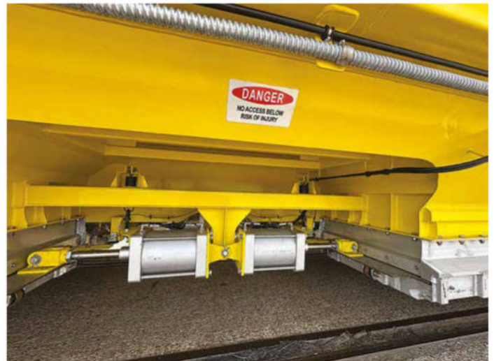
BGIH bottom door actuator detail. Photo Scott by Fitzgerald.
