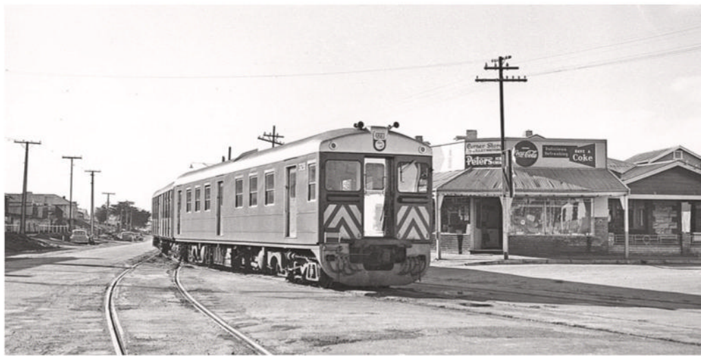
Doug Colquhoun photographed a Redhen set traversing the three-way turnout entering Henley Beach on the last day of operations on the 31st of August 1957. Photo from the NRM archives.
