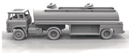
Digital rendering Bedford TK model prime mover two axle, with single axle milk tanker.
