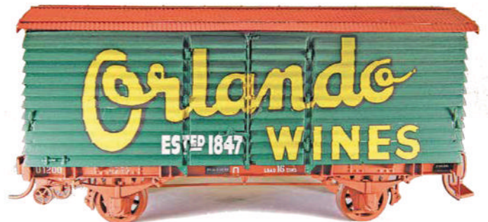
Andrew Maddicks' O scale (1:48) VR four-wheel U van is constructed from a Veteran Models kit. It is finished with Floquil zinc chromate primer and Humbrol Brunswick Green. The decal was supplied by Railways of Victoria.
