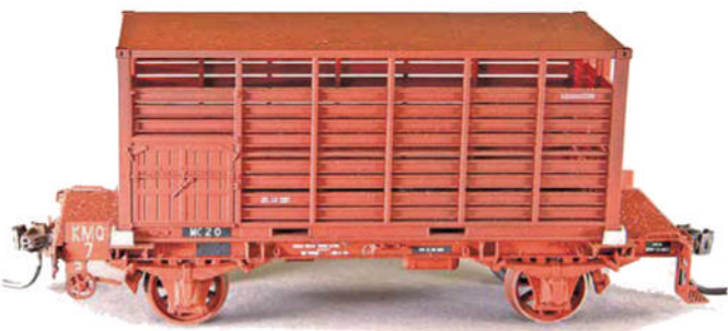
Denis Kahl's four-wheel container flat KMQ7 with livestock container MC20. The flat wagon is a Model Etch kit with the number plate relocated to match the prototype. The container is an SDS Models VR cattle container with some light weathering.
