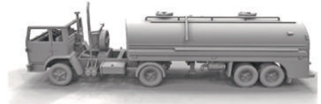
Digital rendering International ACCO prime mover two axle, with two axle milk tanker.
