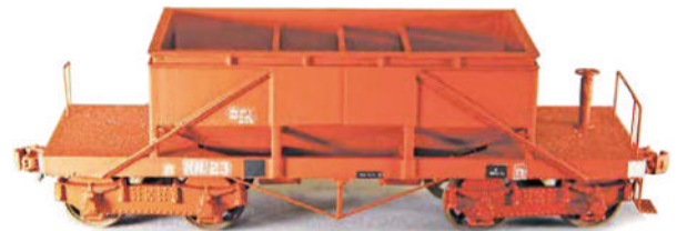
David O'Hare's model of NN 23 is a Pauls 3D print, with some sanding and filling. He added some extra etched brass details, such as the shunter's steps, handbrake and handrails. It is painted with custom spray paint from an automotive paint supplier.
