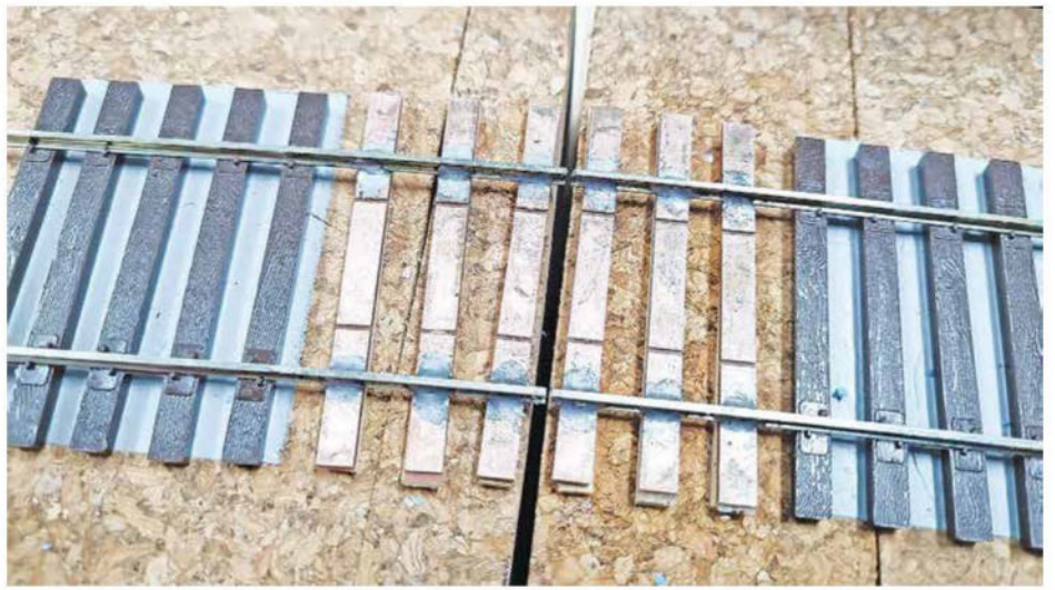
A close-up view of the join between the edge of the bridge (right) and the rest of the layout. The rails are soldered to three printed circuit board sleepers each side of the gap, which have been shimmed with strip wood to match the Micro-engineering code 100 flexible track either side. The shims are glued to the bottom of the circuit board sleepers with Pliobond* (a contact adhesive), and to the cork roadbed with PVA. Once everything is secured, the gap in the rails is cut with a rotary tool. *Pliobond, a product manufactured in USA, can be difficult to source from Australian retailers, I get my supply from Fast Tracks in Canada.
