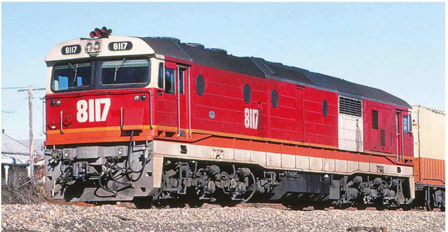
Locomotive 8117 at North Goulburn on 17th July 1984. 8117 has its mansard air intake grille plated over and a new body side intake installed, the new panel is painted in white undercoat, this panel mismatch might be a good modelling feature.
