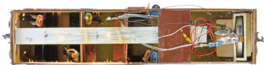
This van is fitted with a passenger compartment and red side lights powered from a button battery. A latching reed switch with a magnet turns the lights on and off when required.
