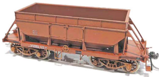
IDR Models painted pilot model of the VR VHWA ballast hopper wagon with spoke wheels and solid bearings.
