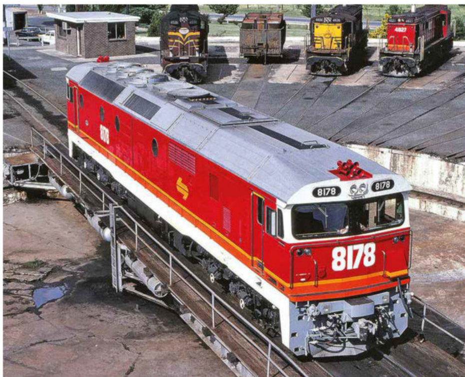
Locomotive 8178 at Goulburn Locomotive Depot on 25th December 1985. 8178's roof is still clean and the black walkway across the crown of the roof can be clearly seen. From 8128 onwards, the class were delivered with body side air intake grilles and four body side portholes. In the background are stabled 4531, 4826 and 4827.
