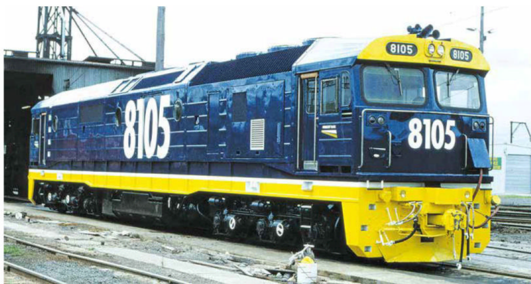
Locomotive 8105 at DELEC in March 1993 following CCO and repaint into the final 'FreightRail' simplified livery (deleting the grey and moving the yellow band down to cover the headstock and pilot). Clyde accomplished the CCO at their Kelso facility, in addition to the overhaul, two doors were added to the engine room body side panels. Both 8105 and 8107 had the air conditioner grille painted white.
