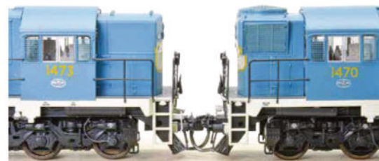
Locomotive 1473 is fitted with a No. 12 coupler box. 1470 is standard with a No. 16 coupler box. The difference is minimal.
