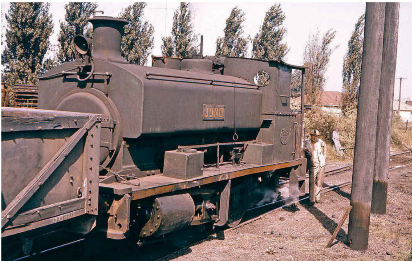
On the 22nd February 1961, Comsteel Shunter Juno, an Andrew Barclay 0-4-0 built in 1923 shunts the sidings. Photo late Weston Langford,
