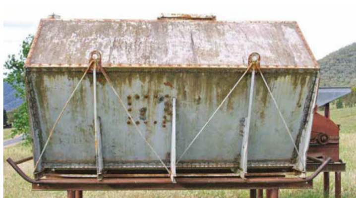
▲ Square on view of cement container with the early lift rings and rods. Photo By Chris Pearce.
