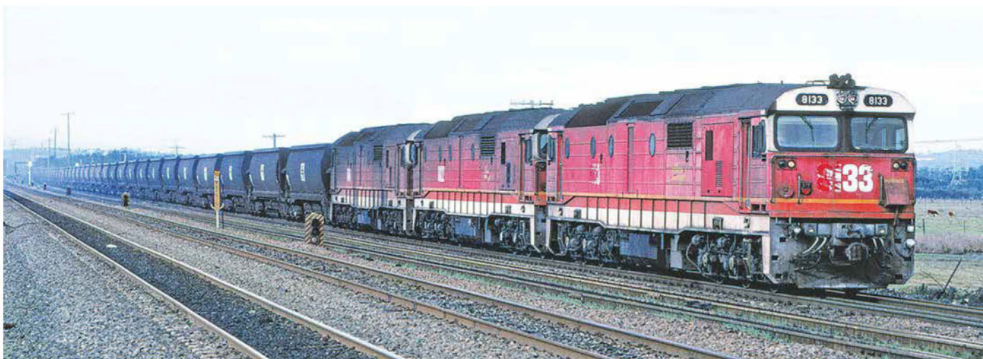
Locomotives 8133, 8122, 8110 and 8175 pass through Hexham with an empty coal train on 20th June 1991. The constant punishing environment of coal haulage operations have clearly affected the physical state of the Hunter Valley 81 class fleet. 8133's numbers are starting to wear away and the body side panels are showing signs of advanced fading. The cab probably leaks like a sieve in the rain! 8110 being the last locomotive in the consist is more heavily coated with exhaust grime.
