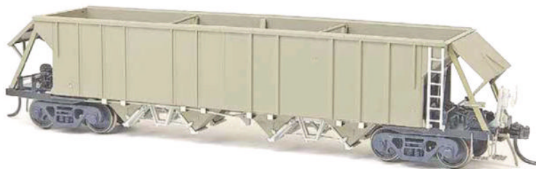
SDS Models unpainted pilot model of their National Rail Corporation's RHGF aggregate hopper.
