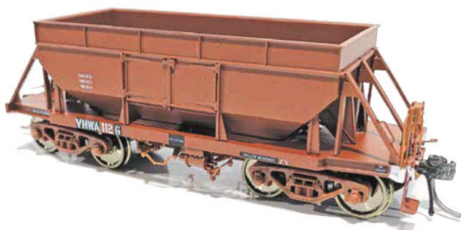
IDR Models painted pilot model of the VR VHWA ballast hopper wagon late version with disk wheels and roller bearings.
