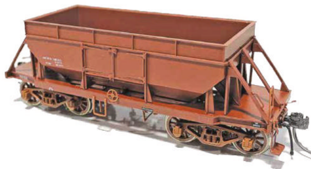
IDR Models painted pilot model of the VR NN ballast hopper wagon, early version with spoke wheels and solid bearings.
