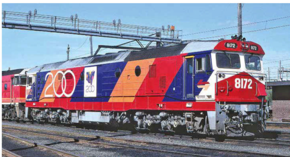
► Locomotive 8172 at DELEC on 5th May 1988 in Bi-Centennial livery, note that the '00' in '200' are a metal plate clearing the air intake grille.
