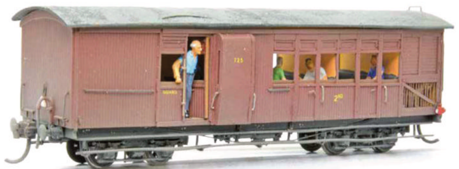
Griffith van No. 725, has two 2nd class compartments. Classed as a GV, in later years this was changed to BGV. There was also a three-compartment version as well. Modelling with the window down and doors open adds another dimension to the model giving that 'in service' appearance. It also opens up the interior, making it visible.
