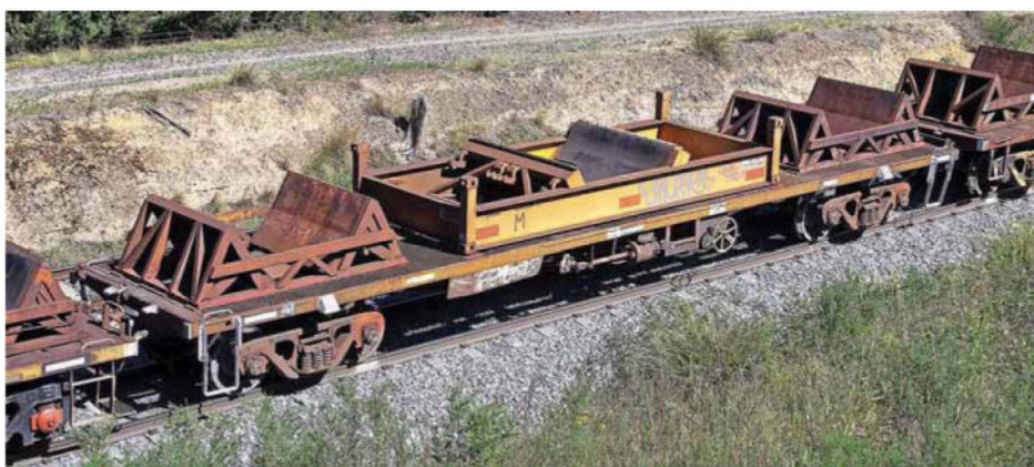
Illustrating the use of fixed and container cradles is RCBF 20426 with a DMJU jumbo coil container.
