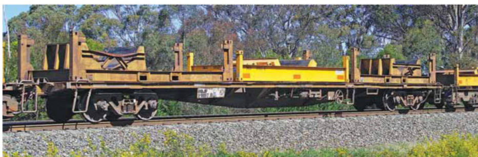
NQJF with a DMJU jumbo coil container in the centre 20ft slot.
