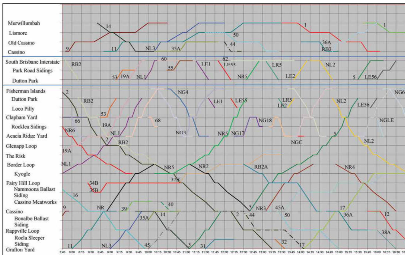
Photo 2: This train graph diagram represents the second eight hour shift from just before 08:00 until just after 16:00. The locations where trains cross or passing movements occur can be identified from the graph.
