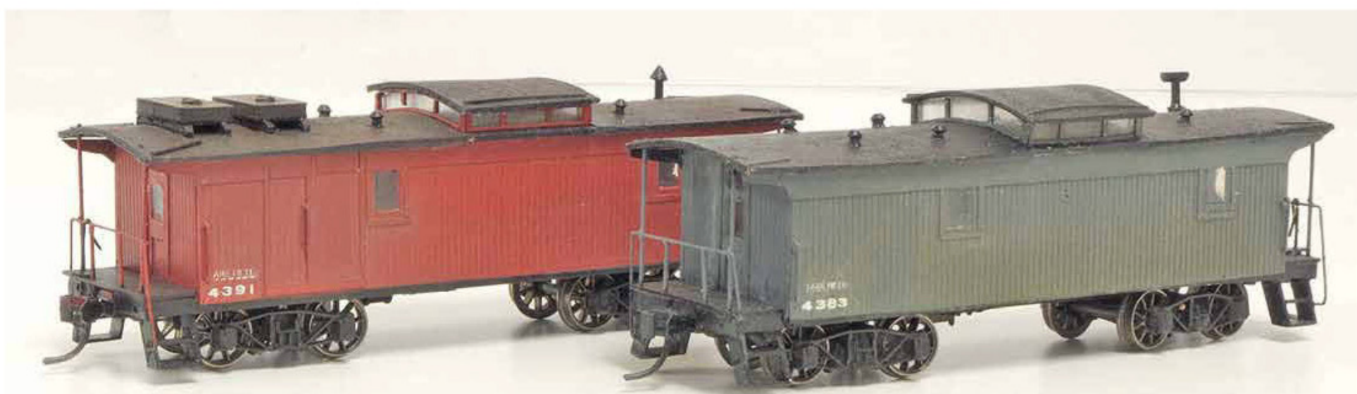
These distinctive pair of Webb design Brakevans, built after Commissioner Webb took over the reigns of the SAR, were scratch built by Ian McGregor in HO scale. Constructed in styrene, the red version with the side loading doors was one of ten vehicles intended for the narrow gauge but didn't eventuate and were issued to traffic on the broad gauge. The grey van was the more common two window variant seen in many old photos of the SAR.
