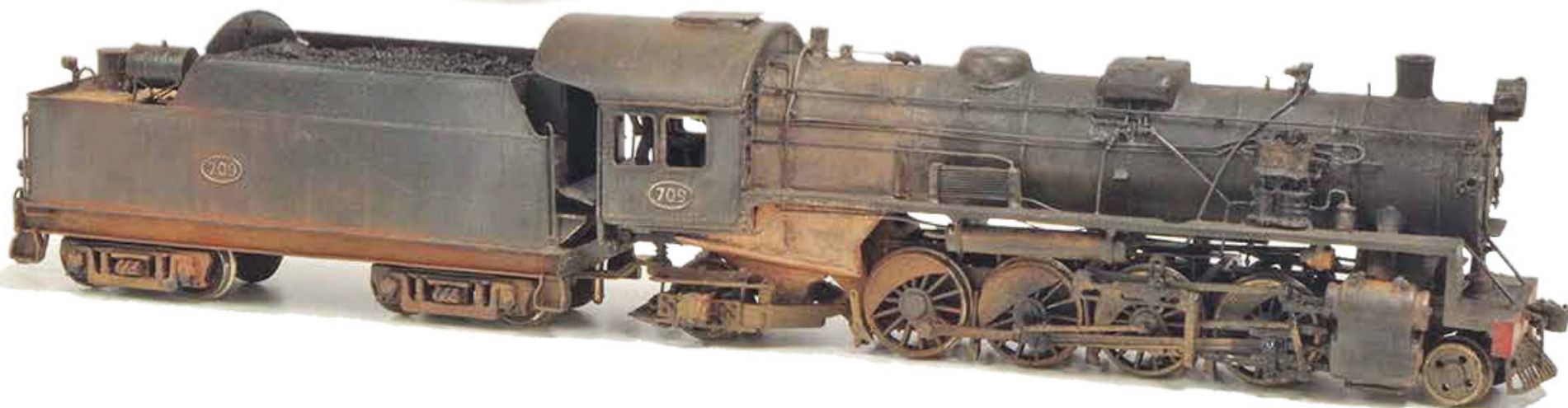
▼ A Broad Gauge Models HO scale white metal and brass SAR 700 Class kit of No.709 by Scott Ferguson. Weathering obviously played a big part of the look of this model, depicting its last days in service. 709 was the only locomotive to be fitted with a footplate mounted after-cooler to remove oil from the compressed air lines, when the two single air compressors were replaced by a single cross compound compressor, as seen on this model.
