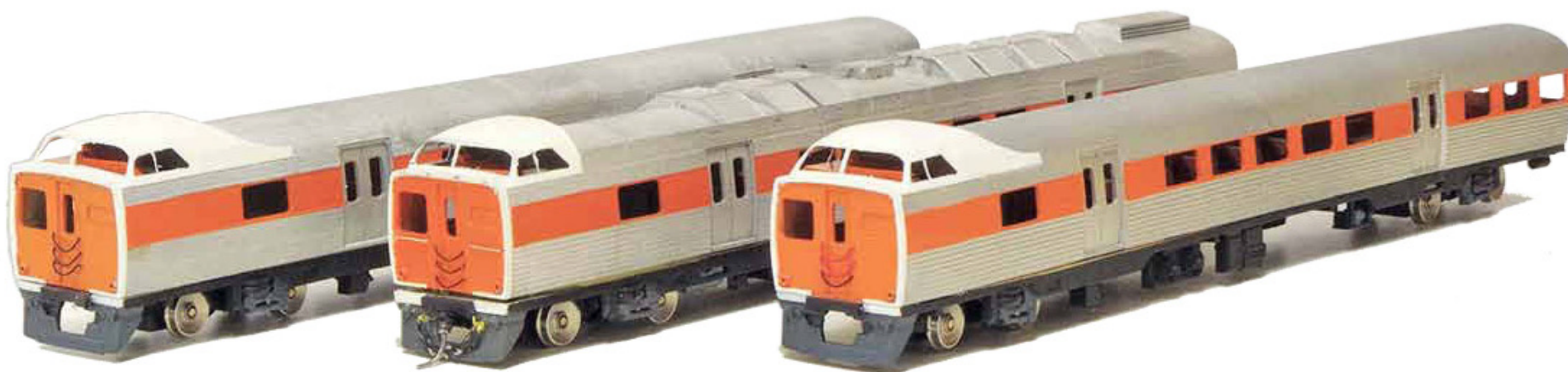
A trio of 'Jumbo' railcars in HO Scale built by Sean Rendell. After acquiring the bodies of these 2100-2000-2100 Class cars, Sean designed, drafted and 3D printed interiors and underfloor details to fit out the models to create the commonly seen railcar set of the 1980s. The prototype vehicles were built for the then State Transport Authority by Comeng and entered into service in 1980 and 1981.
