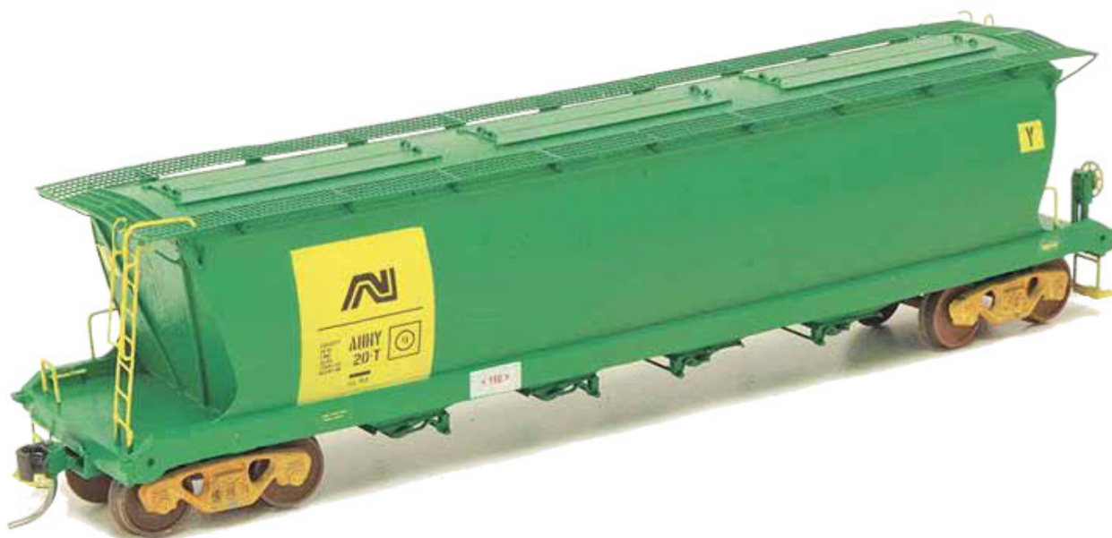
An AHHY Wheat hopper in HO scale built by Sean Rendell in Australian National livery. He has designed it as a craftsman kit, which requires some soldering, with a two piece body. Sean did the design and drafting on Sketchup and 3D printing using his own printer to produce the model. The grid catwalks were also drafted by Sean then sent to an Australian company, Mastercut Technologies, to produce the etches. Decals were produced by Signs Of All Kinds for Sean's requirements. There are other kit items in Sean's small business called Scale Model Reproductions.
