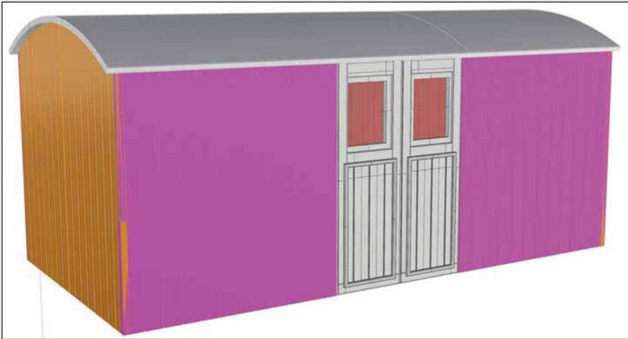
Figure 14. Once the first door has been created, it is mirrored and copied to make the other three doors of the van.
