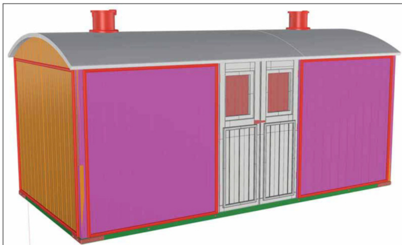
Figure 17. The floor and lamp pots are created using basic primitive solids.
