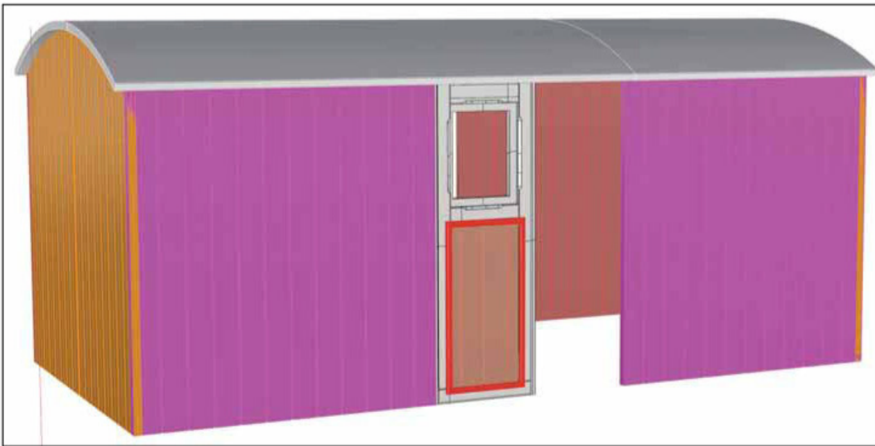
Figure 13. The door is made as a single assembly, from a series of extruded solids in a similar manner to the van sides.
