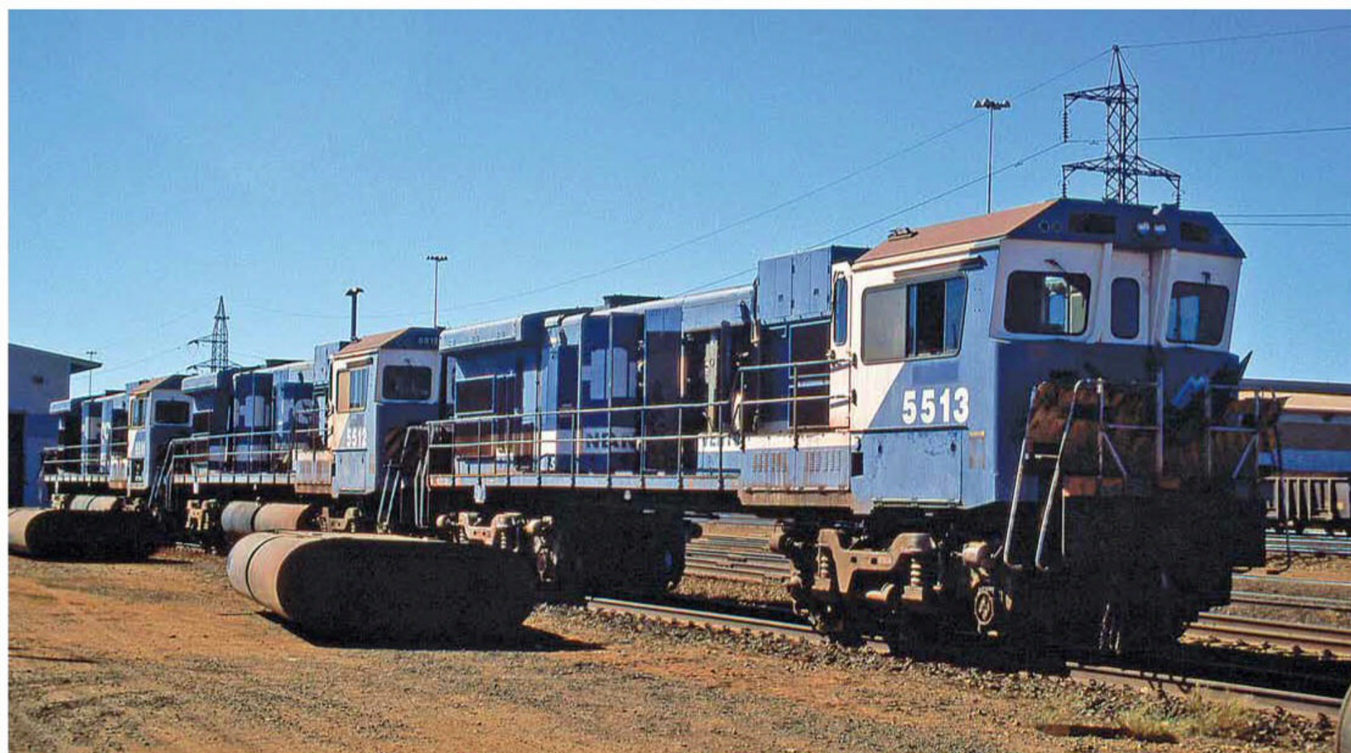
Locomotives 5513, 5512 and 5511 sit at Nelson Point on 1 June 2002. The fuel tanks and snow ploughs have been removed in preparation for transportation. In seven days time 5513 will be the first of the trio to be transported south to Perth. Photo the late Jim Bisdee (Phil Melling Collection)
