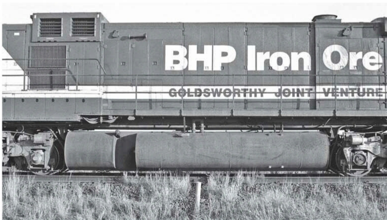
Locomotive 5506 'Mt Goldsworthy'. Observer's side, the resistor grids are visible in the dynamic brake housing. The long hood air horn is mounted on the long hood just aft of the dynamic brake housing.
