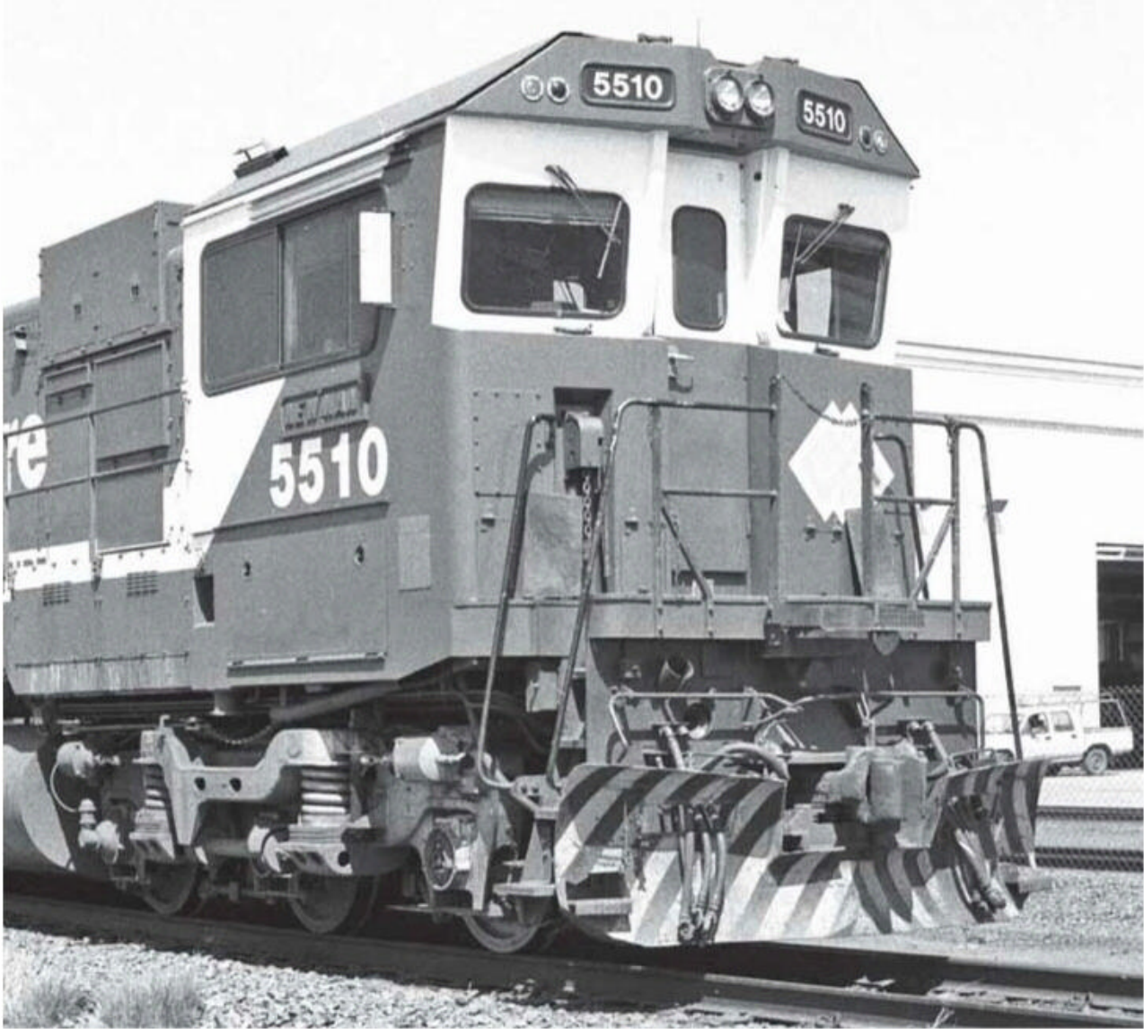
Locomotive 5510 ‘Newman’. As this locomotive is allocated to the Goldsworthy line at this time, it is fitted with rear vision mirrors. Also note the MU cable holder fitted just under the pilot front walkway sill – anti climber.
