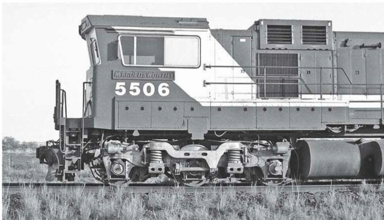
Locomotive 5506 'Mt Goldsworthy'. Observer's side, with an array of access panels which allows access to air equipment racks and electrical equipment under the cab and walkway. The dynamic brake outlets are located behind the Operator's cab in the box assembly which sits above the long hood roof line.
