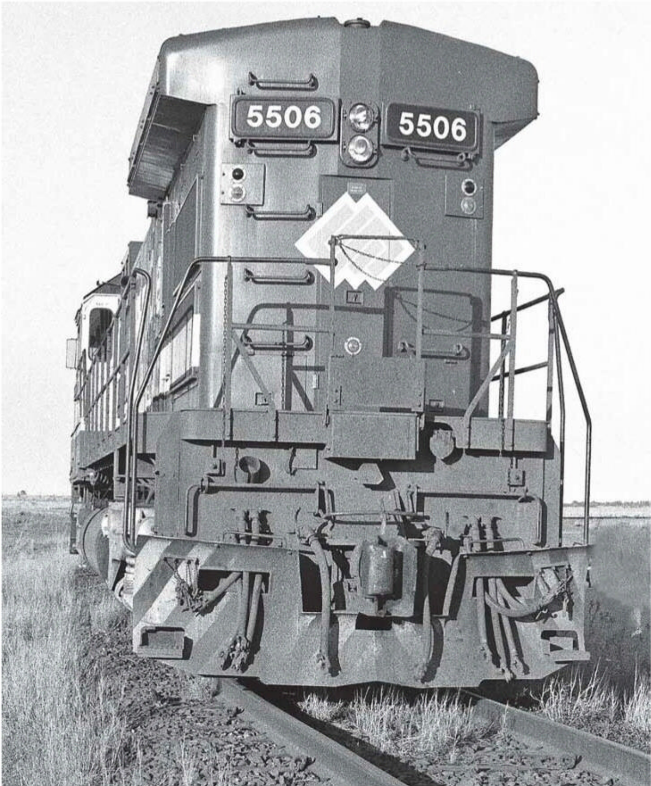
Locomotive 5506 'Mt Goldsworthy'. The radiator end, items of note include double parker lights, coupler light and switches.
