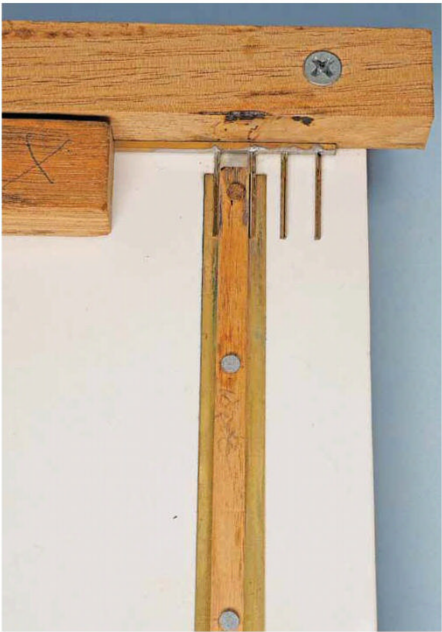
27 Jig for soldering 1.50mm brass U channel on top of 1.00mm angle brass.
