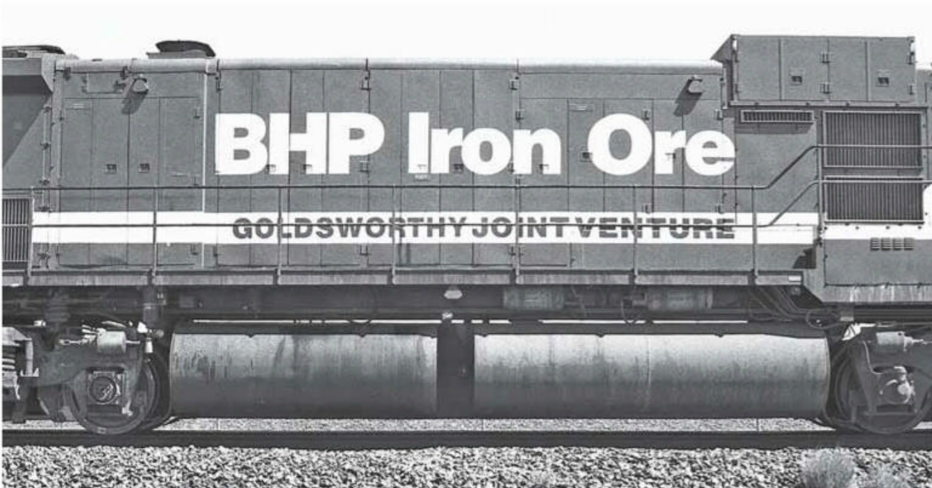
Locomotive 5510 'Newman'. Driver's side. The fire extinguisher bottles can be seen mounted under the walkway next to the frame. Note the positioning of the 'Goldsworthy Joint Venture' lettering in relation to the 'BHP Iron Ore' on each long hood door.
