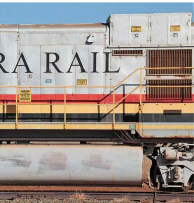
Locomotive 5506 'Mt Goldsworthy'. Observer's side, with an array of access panels which allows access to air equipment racks and electrical equipment under the cab and walkway. The dynamic brake outlets are located behind the Operator's cab in the box assembly which sits above the long hood roof line.
