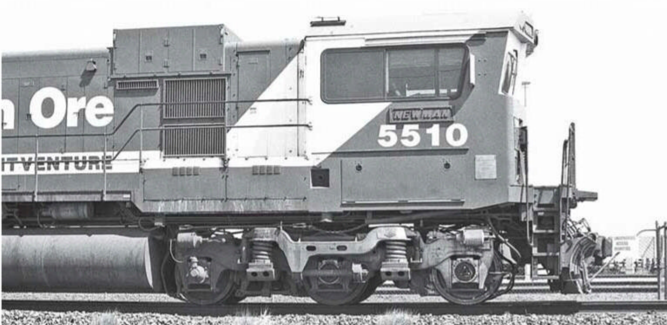
Locomotive 5510 'Newman'. Driver's side. Observe the location of the builder's plate and the nameplate, just above the builder's plate is an additional plate added after delivery, it sits directly on top of the original plate. This plate included the build date and the builder's number, as this was omitted from the original builder's plate. Refer photo 13 which has the original plate removed and additional plate is still installed. Aft of the operator's cab, nestled into the walkway, are the two battery boxes. Compare the battery box covers with the ones installed on 'Pilbara Rail' 5051 and 5052.
