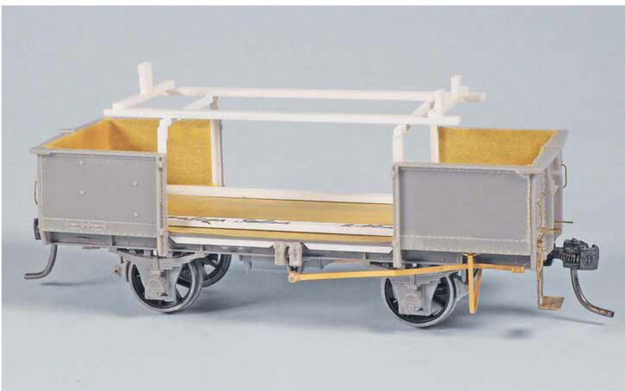
29 Gluing posts to wagon using block of wood to ensure they are square.
