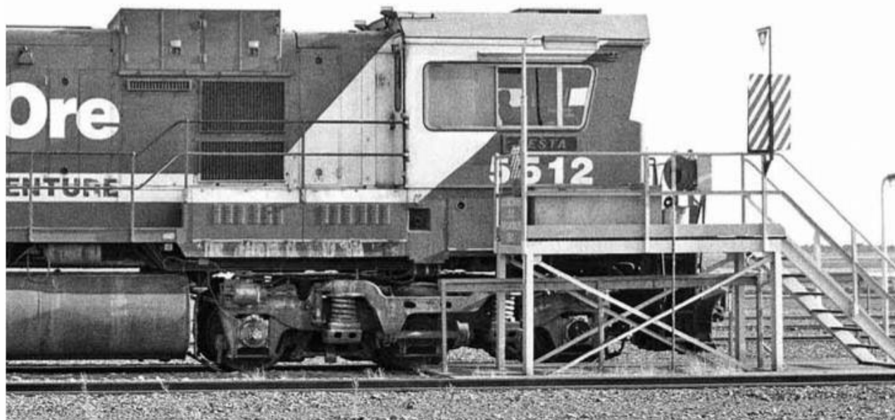
Locomotive 5512 'Hesta'. Driver's side, from this angle the Locotrol antennas are visible mounted on the operator's cab rear wall.
