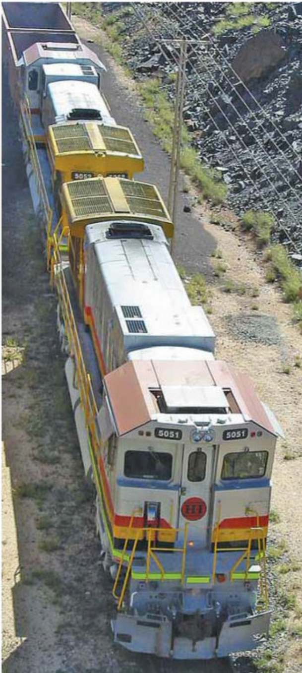
Locomotives 5051 and 5052 are about to depart the empty car line at Parker Point in August 2003. Observe the sand filler caps on the operator's cab roof, (these were installed by BHP after delivery from Goninan) the double skin roof and the positioning of the air-conditioner. Also visible is the dynamic brake air intake.
