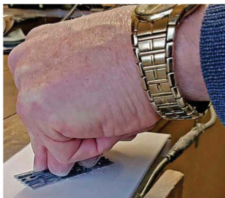
24 Thinning wagon floor on belt sander.
