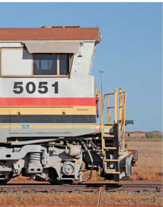
Locomotive 5051. Driver's side (operator's cab). Comparing with 5510, the builder's plate is missing, serial number plate still installed. Battery box covers have a grate instead of louvres. Cab sunshades installed, along with a slimline cab mirror. Sinclair antenna has been removed, and whip aerials installed.
