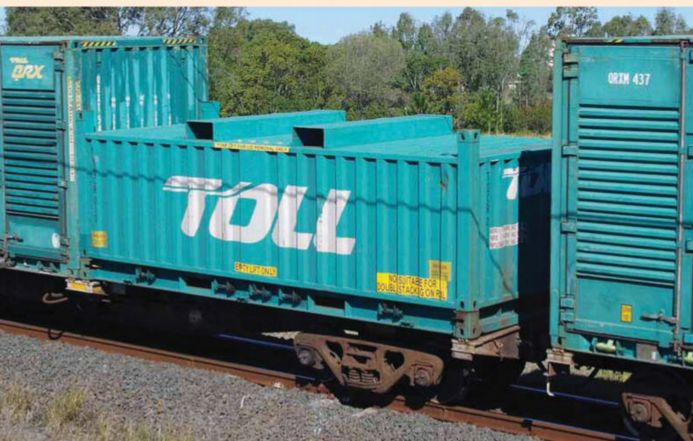
▶ Cartainers have been-and-gone in the rail industry, with the mode of transport lasting around 20 years. This December 2005 image shows an RRYR with a yellow Autotrans cartainer leading three Toll-branded cartainers. All display the mansard roof design; the train is approaching Bowral tunnel.
