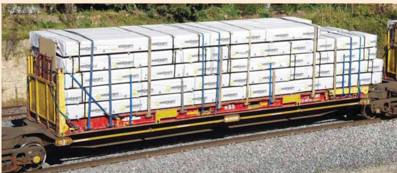
Extremely common freight from Western Australia to the eastern states is Wesbeam timber products. They are moved on K&S flatracks and are packaged in neatly-wrapped bundles that are then meticulously strapped down for the long journey. A head-board reduces the risk of a load shift.
