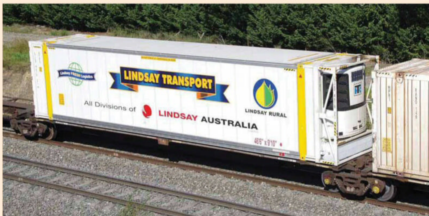
With the now common yellow or orange posts to identify the lifting and securing locations of containers longer than 20 ft, this Lindsay Transport 46 foot 6-inch refrigerated container is fitted with a Thermo King unit. The fuel tank sits below the refrigeration unit.
