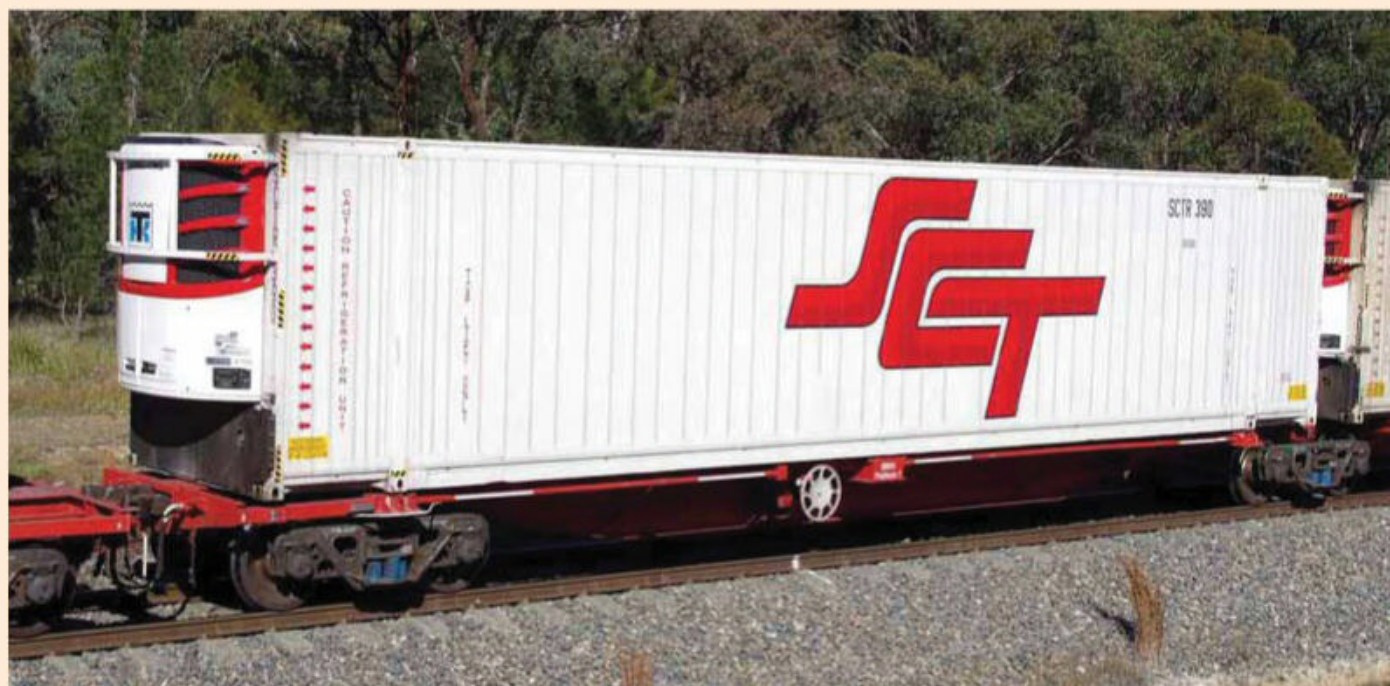
The slim-line fuel tank on this SCT '48plus' refrigerated container is evident when not inside a well wagon. The slim-line fuel tank allows these extra-long refrigerated containers to fit inside a standard 48 foot well wagon for double stacking.
