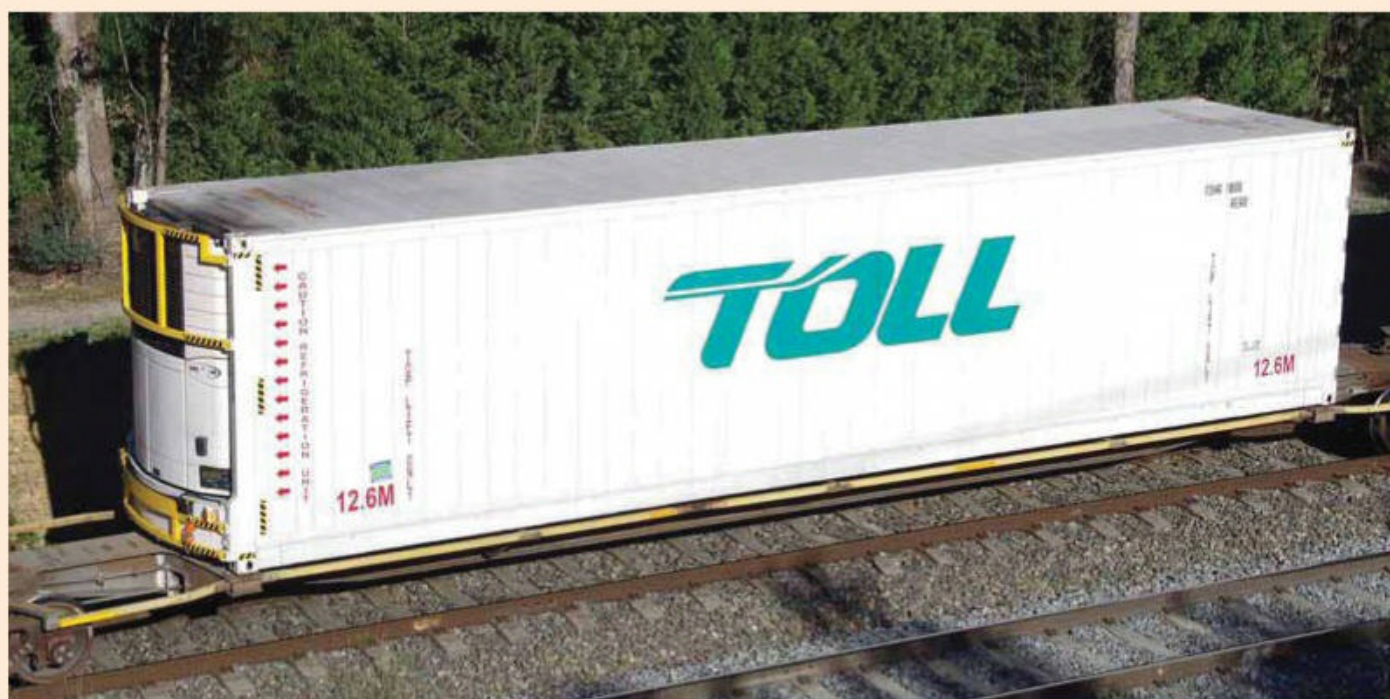
Toll runs a sizeable fleet of '40plus' or 12.6 m self-powered refrigerated containers. Many of them operate up and down the east coast, including across the Tasman to Burnie on the Toll ferry. The compact refrigeration unit allows these containers to sometimes be placed on the end of a wagon or facing another container without the end unit protruding too far to cause a problem.
