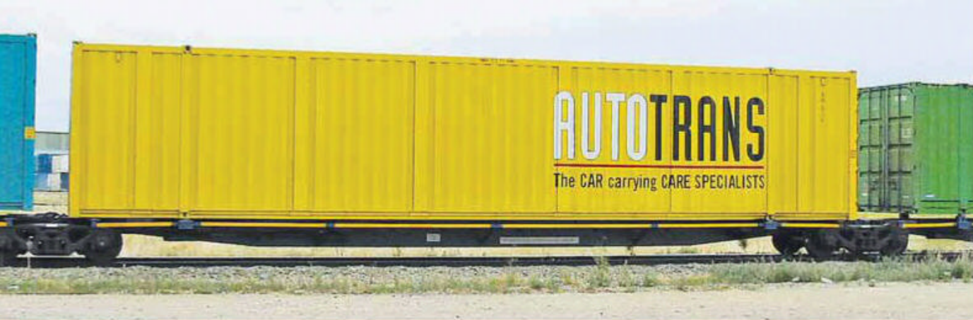
◀▶ An early version flat-roof Autotrans 53 foot cartainer on an MP5 service on 28 January 2005. A Toll mansard roofed version shown below for comparison. Photo by Scott Fitzgerald.
