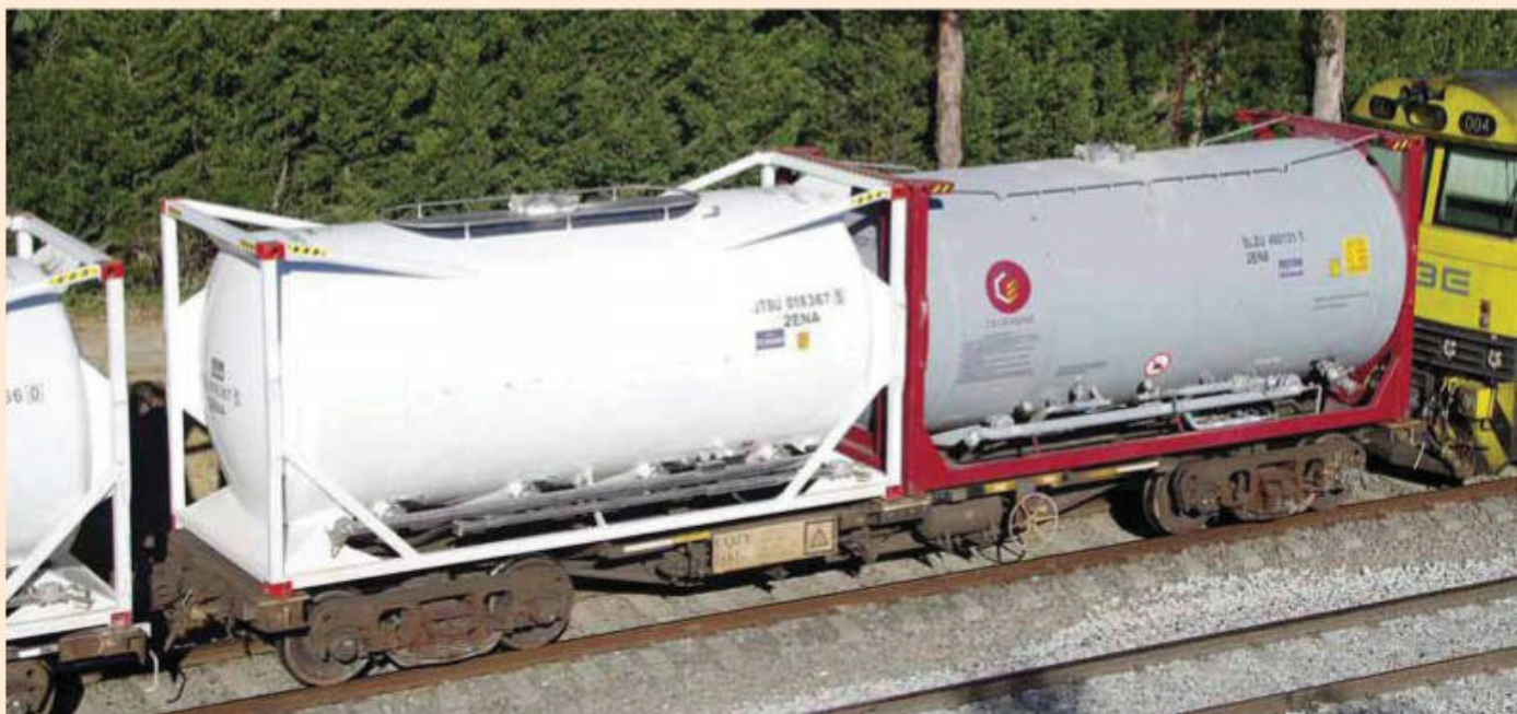
Cement and dry powders are commonly moved long distance by rail due to the mass of the product. Dry tanks are common across most rail networks and can often be found on both dedicated trains and common intermodal services.
