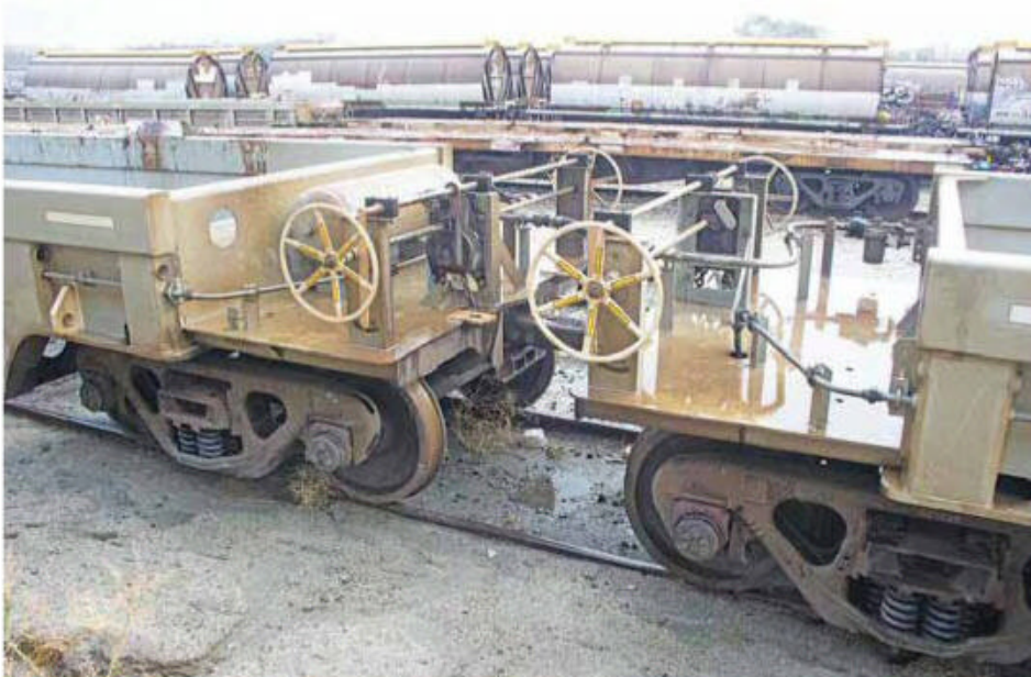
Handbrake assemblies. Note the drawbar and that the hand brakes are located in the centre of each two-pack.
