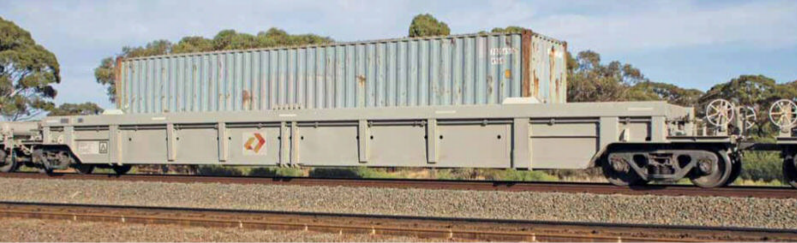
On this side the main reservoir (MR) airline utilises the upper pipe line position.
