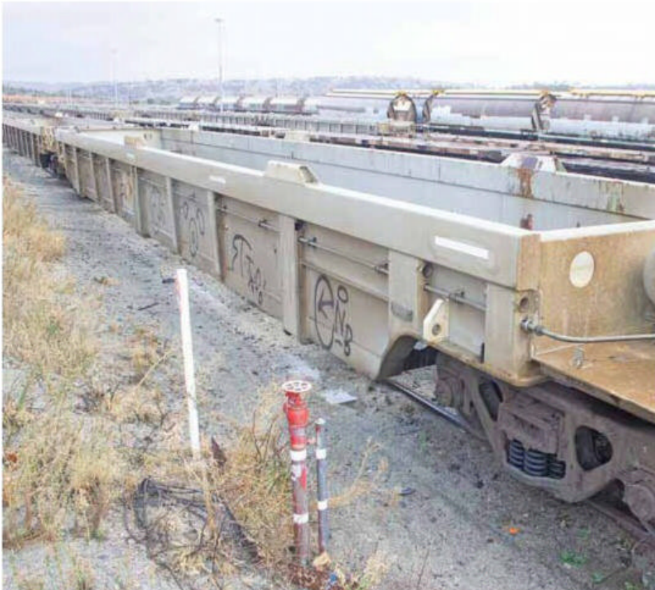
The reservoir non-hand-brake end of the platform. In this view you can see the two airline raceways installed through each upright and the air reservoir stand-offs.
