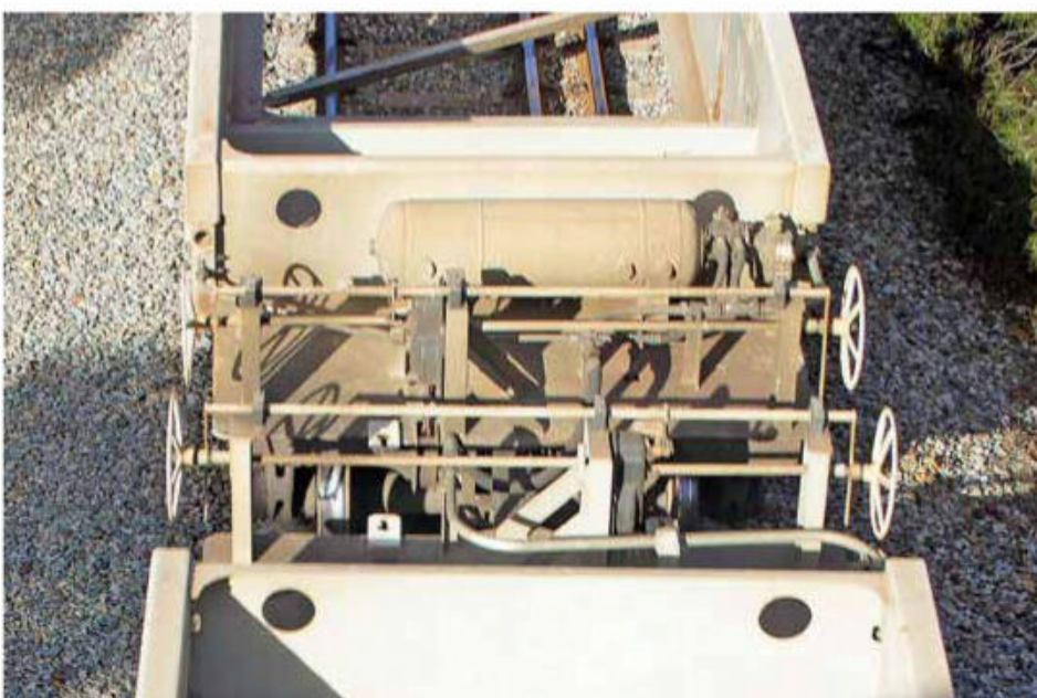
Handbrake assemblies and reservoir top detail.
